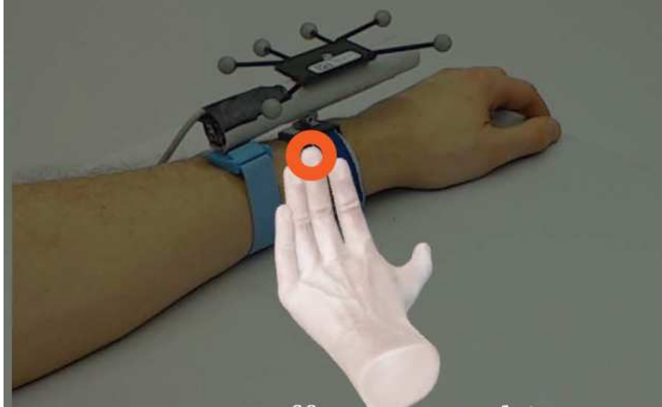
Figure 2.5: The stylo device and the handifact cue in action. Taken from [6].
