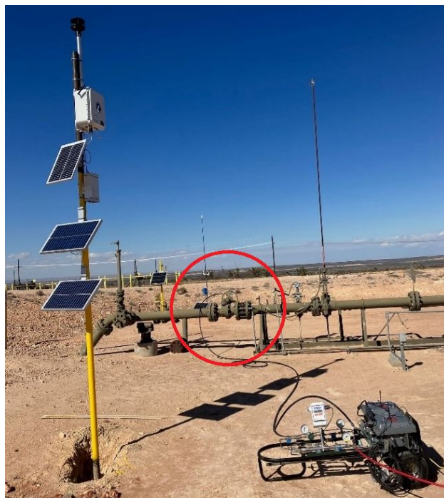
Figure A.6: Mobile release rig with supply inlet connected to the gas line at an oil and gas site during the field campaign.
