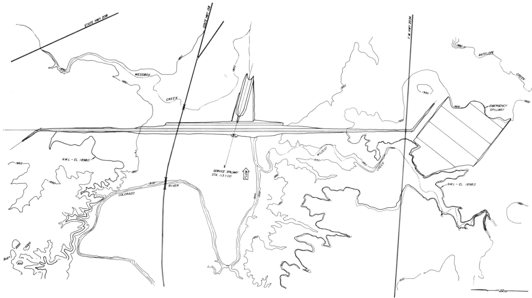
FIGURE 1 GENERAL PLAN OF DAM AND APPURTENANT WORKS
