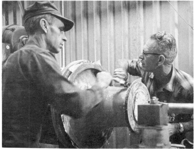
Figure 8. Morning glory mold being covered with fiberglass
