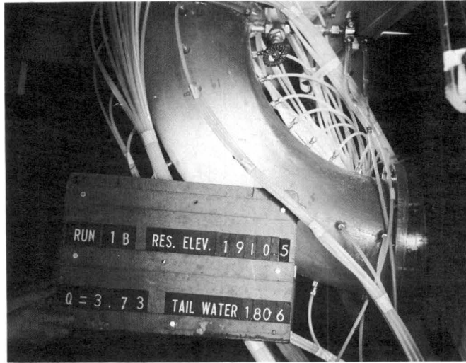
Figure 22. Flow through the vertical bend Q = 37,300 cfs
