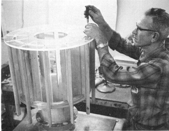
Figure 10. Morning glory spillway during construction
