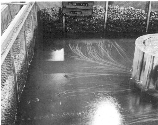
Figure 18 (a). Flow lines into spillway II from the reservoir with water level at 1890.0
