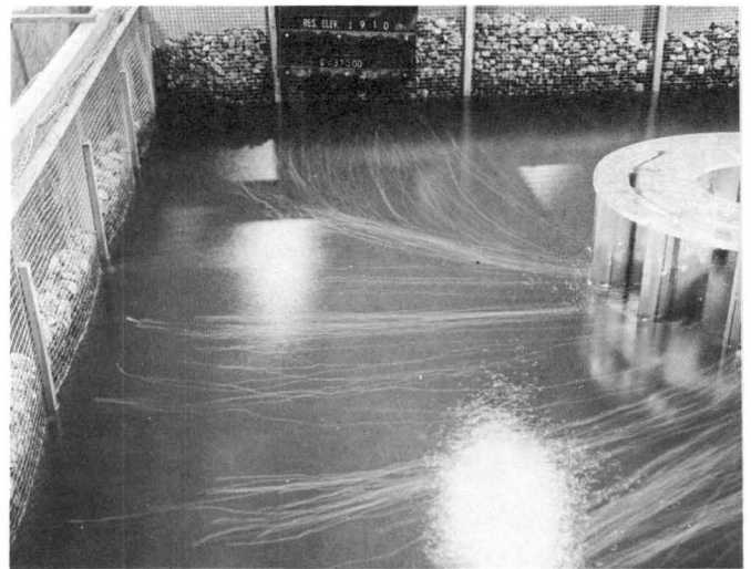
Figure 18 (b). Flow lines into spillway II from the reservoir with water level at 1910.0
