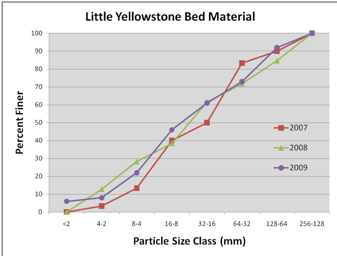
Figure 4.19. LY bed material size distribution 2007-2009. No change is detected during this period. LY was upstream of the 2003 debris flow and therefore not affected.
