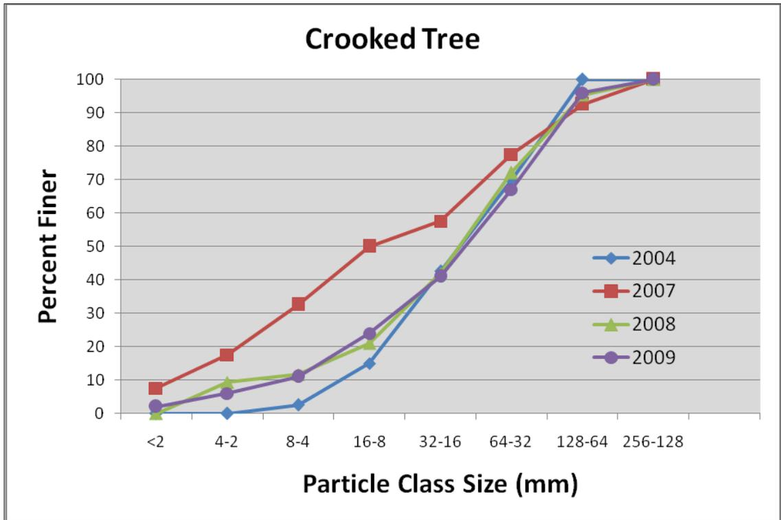
Figure 4.20. CT bed material size distribution 2004 and 2007-2009. Fining of the bed occurred in 2007, followed by coarsening in 2008 and no change in 2009.
