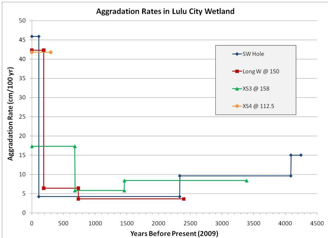
Figure 3.12. Aggradation rates were calculated based on the mean radiocarbon age for each sample and assuming constant rates between each age control point. Each age control point is indicated by a symbol. Locations of radiocarbon-dated cores presented in Figure 3.2.
