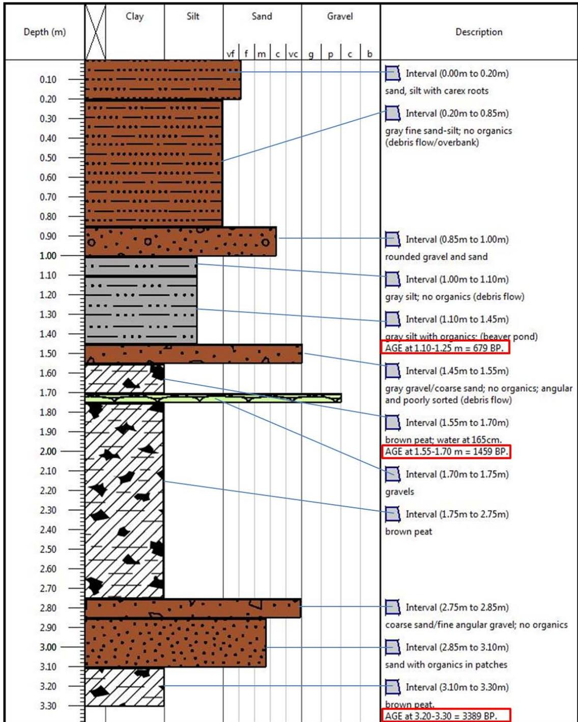
Figure 3.11. XS3 @ 158 m is in the northeast portion of the wetland. The most recent radiocarbon date is from a historic beaver pond at ~1.2 m depth and is dated as ~679 yr BP. Previously, peat was the dominant aggradational process, although four coarse deposits are present from ~679 to 2289 yr BP.
