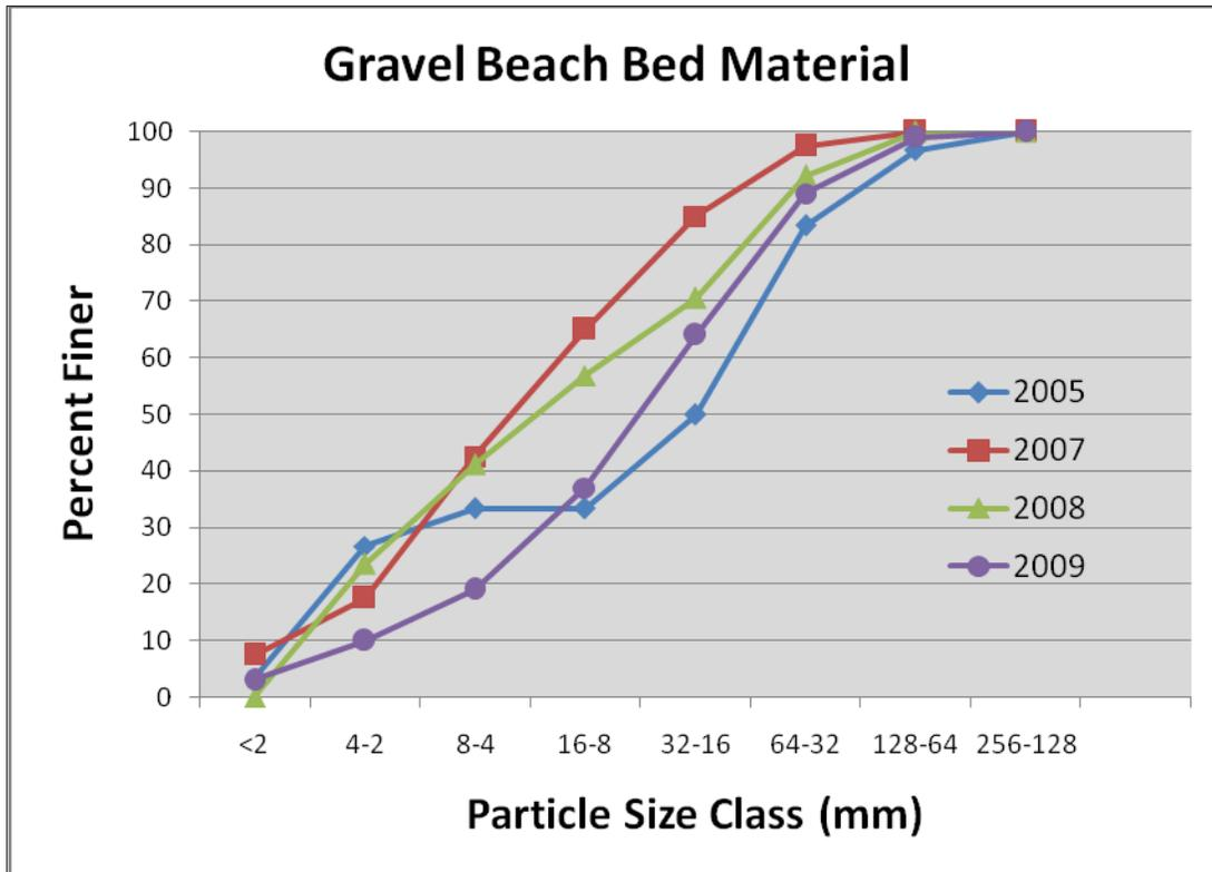
Figure 4.21. GB bed material size distribution 2005 and 2007-2009. Fining of the bed occurred in 2007, followed by coarsening in 2008 and 2009.
