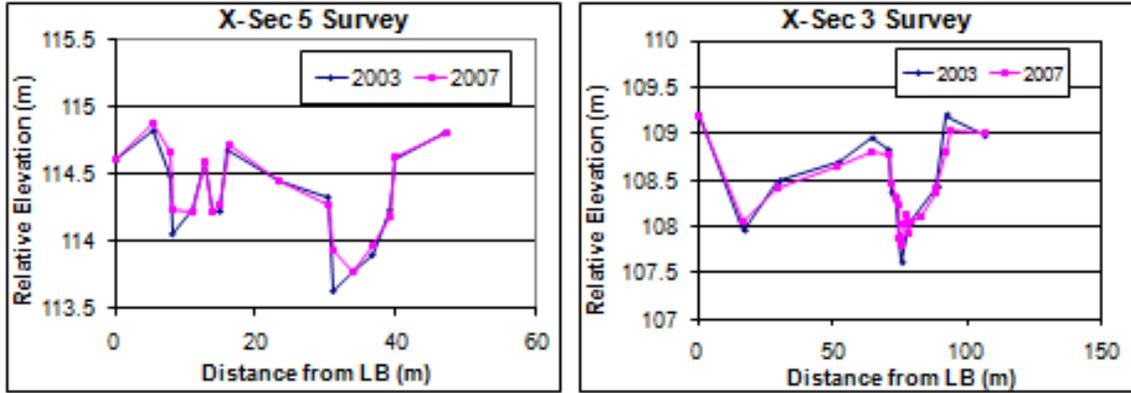
Figure 4.22. Repeat surveys at cross section 5 (250 m downstream of CT) and cross section 3 (20 m upstream of GB), 2003 and 2007. At cross section 5, 20-30 cm of aggradation occurred in the main channel. At cross section 3, no net change was observed.
