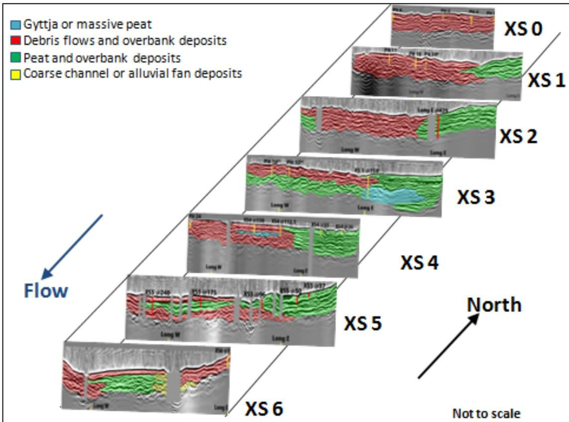
Figure 3.6. GPR surveys show distinctly different facies on the west and east sides of the Lulu City wetland. The east side is dominated by peat and overbank deposits between XS1 and XS5 with no fluvial reworking. The west side is vertically and laterally heterogeneous, although deposits are debris-flow dominated.
