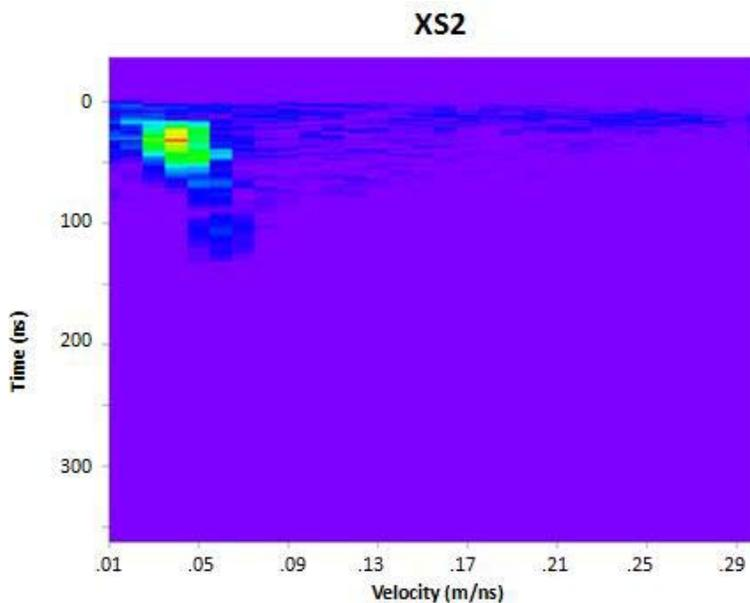
Figure 3.3. XS2 CMP survey velocities are indicated by warm colors over depth. Warm colors indicate electromagnetic propagation velocities and can be used to convert the time of radar return signals to depth in the GPR reflection surveys. In XS2 as well as XS4, a velocity of 0.05 m/ns was observed. The velocity of 0.05 m/ns was applied to all GPR transects to convert reflection time to depth.
