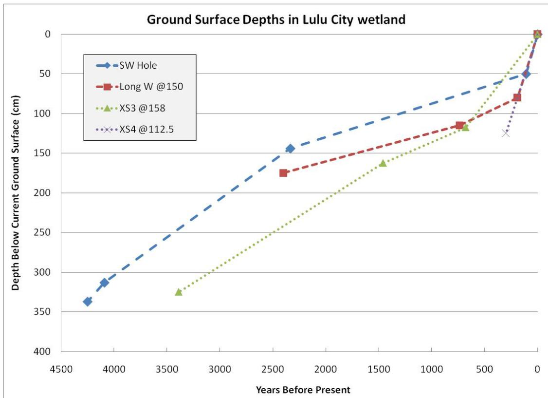
Figure 3.13. The ground surface over time at dated profile locations is generally consistent throughout the Lulu City wetland, assuming no loss of elevation (e.g., deposition and subsequent erosion, or compaction) between dated samples. Steeper slopes indicate faster aggradation rates. Each age control point is indicated by a symbol. Locations of radiocarbon-dated cores are presented in Figure 3.2.
