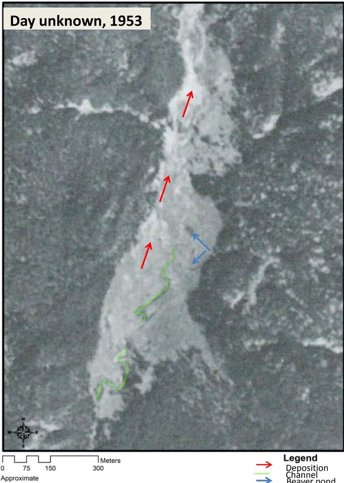
The 1953 image shows extensive deposition in the northwest corner of the wetland. Except in segments where the 1937 channel is still intact, there is no main channel. A second beaver pond is visible, though more may have been present but not visible due to low resolution.
