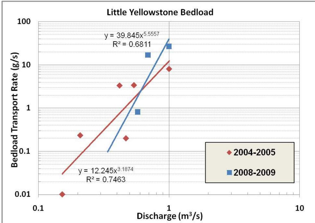
Figure 4.16. LY bedload sediment rating curve comparison of 2004-2005 with 2008-2009. LY was not affected by the 2003 debris flow and no change in bedload transport is seen.
