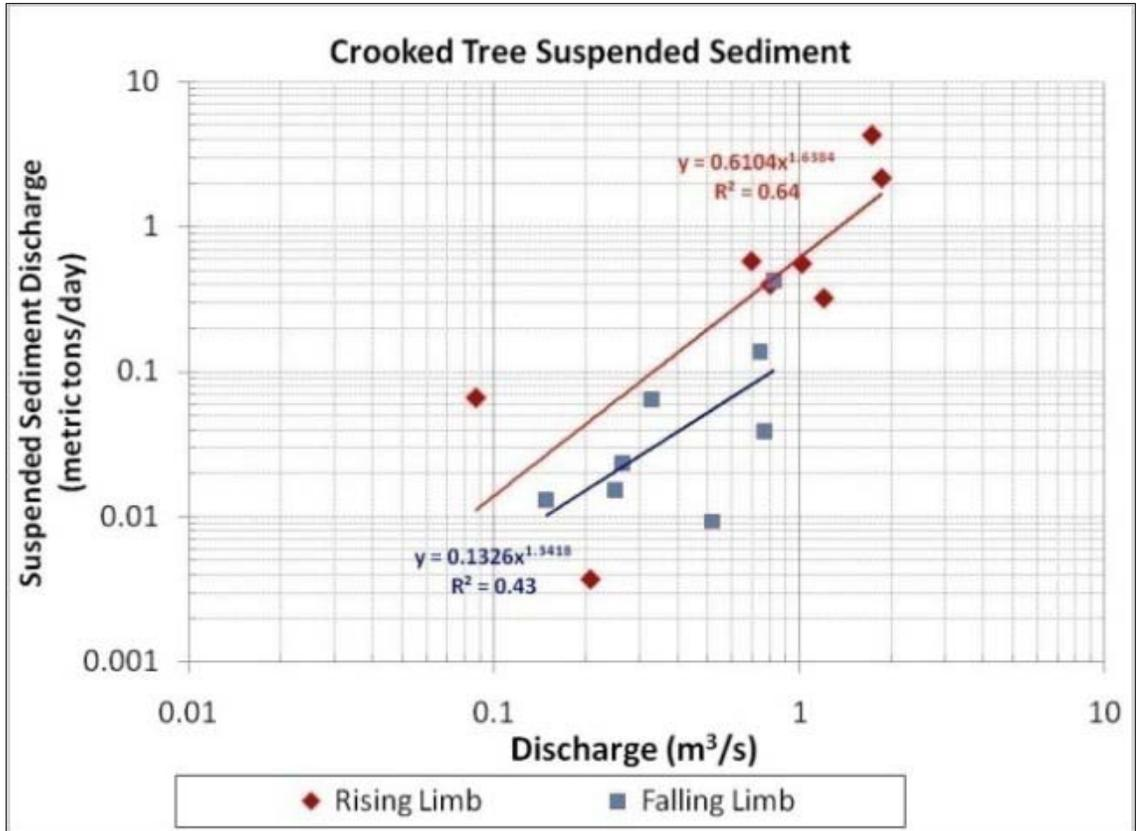
Figure 4.12. CT suspended sediment rating curve comparison of rising and falling limb flows. Data suggest clockwise hysteresis.
