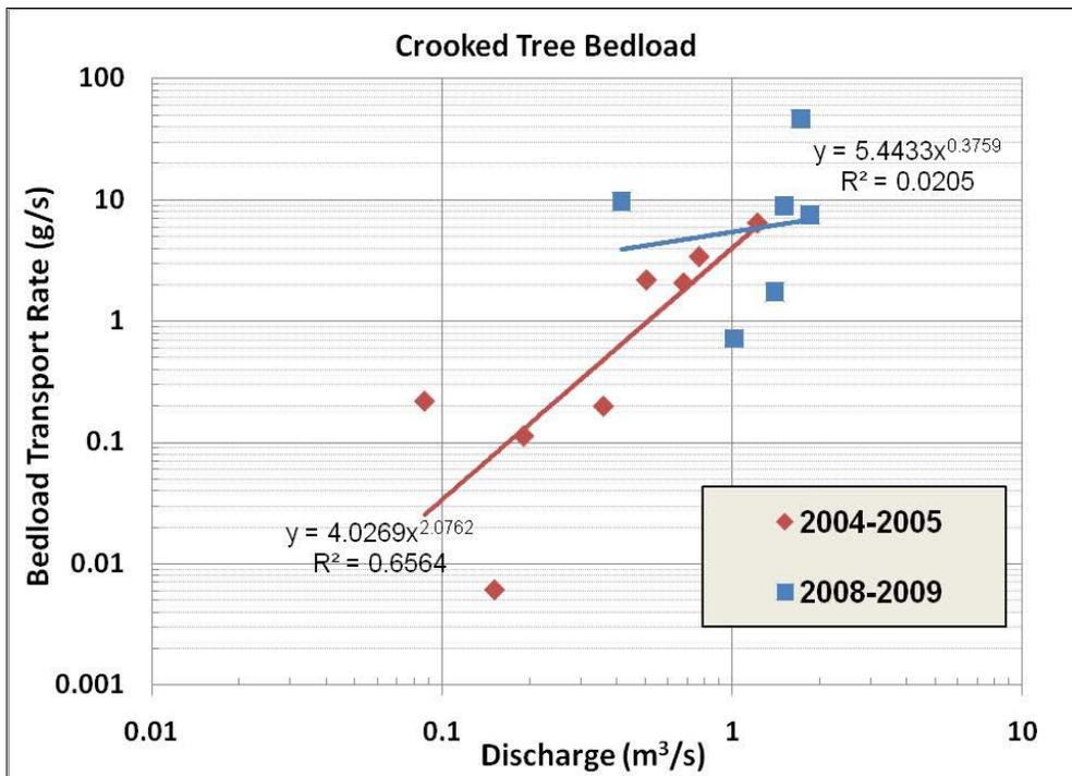
Figure 4.17. CT bedload sediment rating curve comparison of 2004-2005 with 2008-2009. There is no change in bedload transport.
