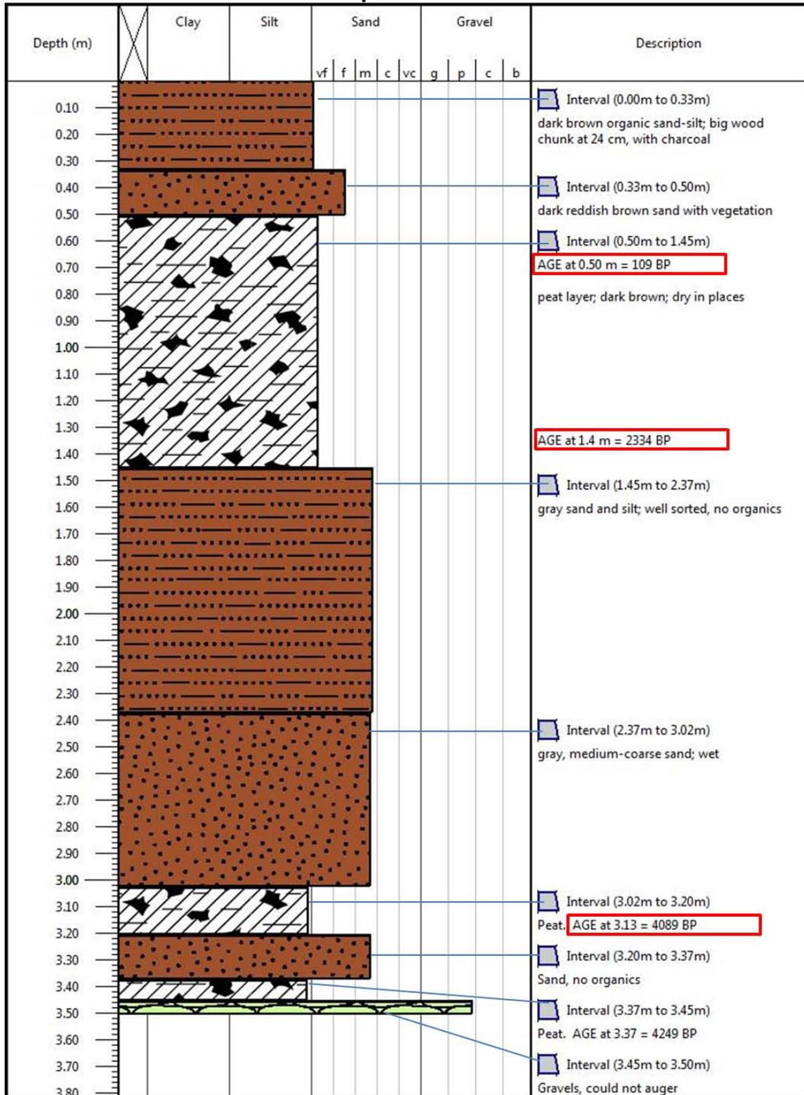
Figure 3.10. SW Hole is in the southwest portion of the wetland. This was dug with shovels to ~2 m, then augered to 3.5 m. Radiocarbon dates from 0.5 and 1.4 m depth indicate 90 cm of peat accumulation in ~2200 years prior to ~50 cm of sediment deposition in the past two centuries.
