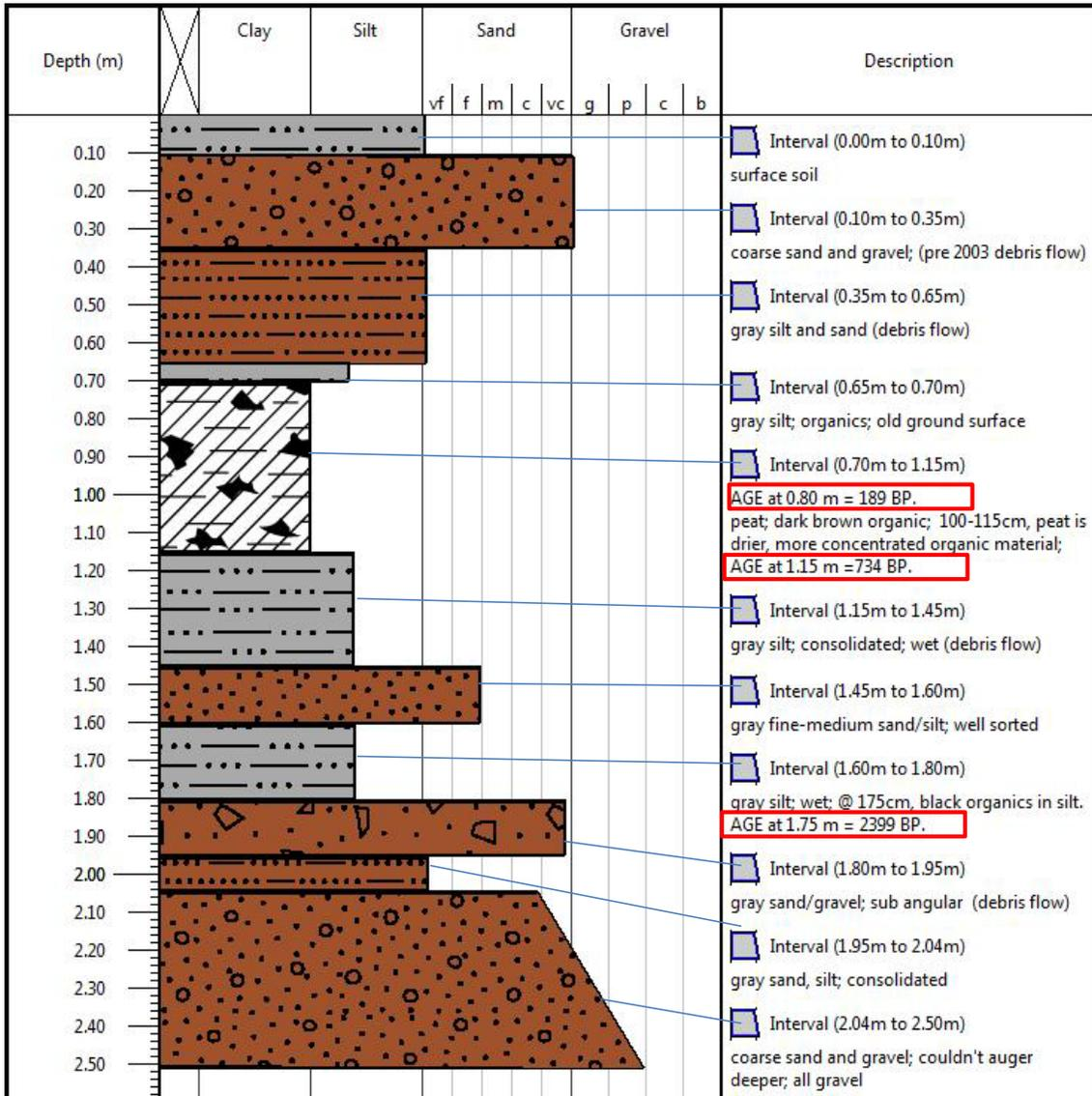
Figure 3.9. Long W @150 m is in the southwest portion of the wetland between XS4 and XS5. Ages obtained from radiocarbon dating are outlined in red for emphasis. Dates from 1.15 m and 0.8 m depth indicate 35 cm of peat accumulation in the ~545 years prior to 65 cm of sediment deposition in the past two centuries.
