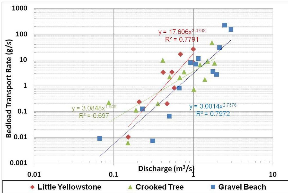
Figure 4.15. Bedload transport rating curves for LY, CT, and GB are similar at all three stations.
