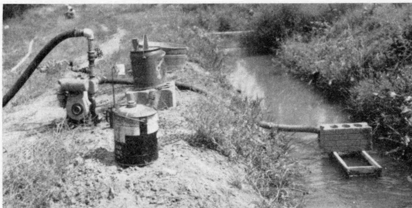
Figure 9.—Portable engine-powered pumping plant on ditch bank. Water is being drawn temporarily from within a frame covered by a screen which required frequent cleaning.
