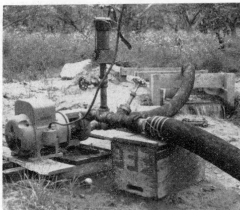
Figure 5. — Portable electric-powered pumping unit. Surplus water flows over horizontal screen. The suction hose enters from the top. Better design would be a side entrance to avoid a high spot objectionable in suction pipes.
