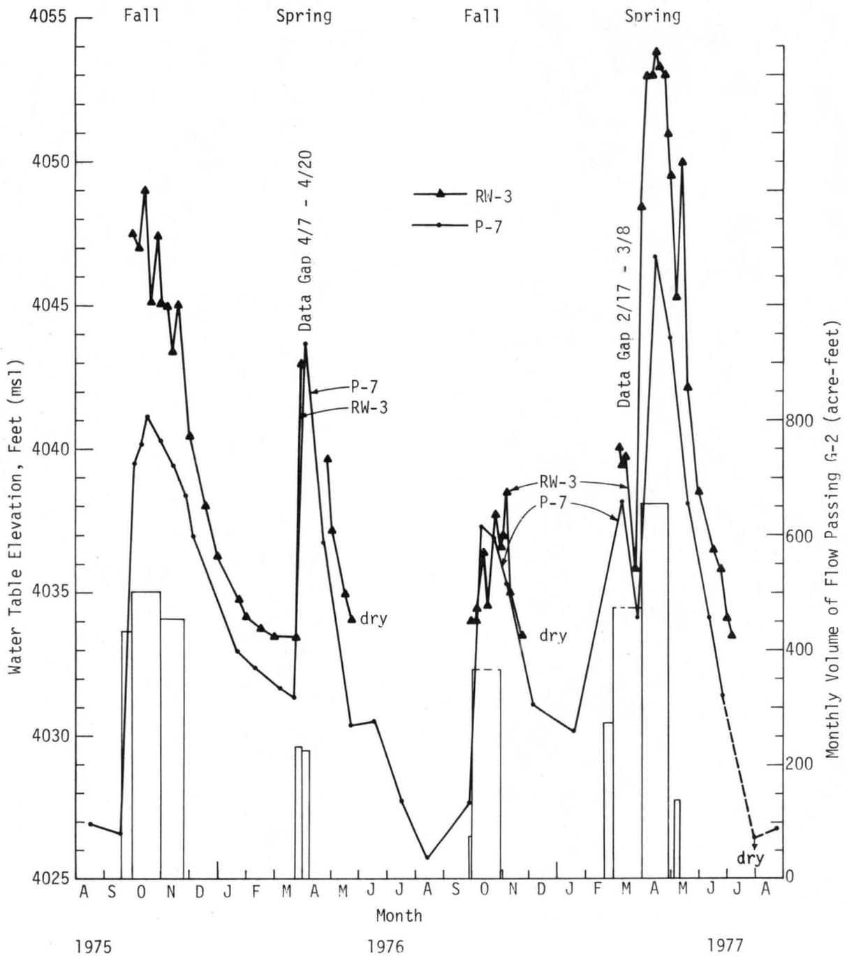
Figure 10. Water Table Hydrographs for Observation Wells P-7 and RW-3 With Bar Graphs of Recharge Flows
