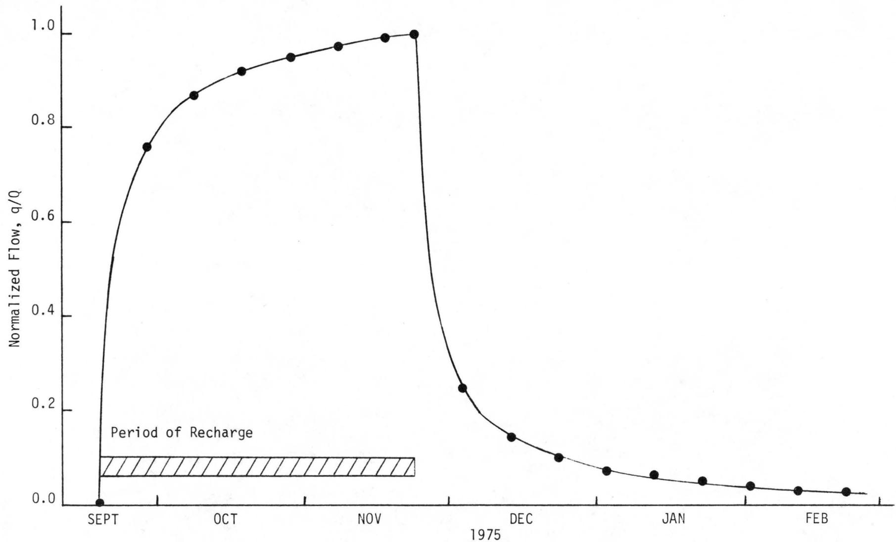
Figure 11. Normalized Flow into Drainage Ditch as a Function of Time for Cross-section through P-14 and P-15.
