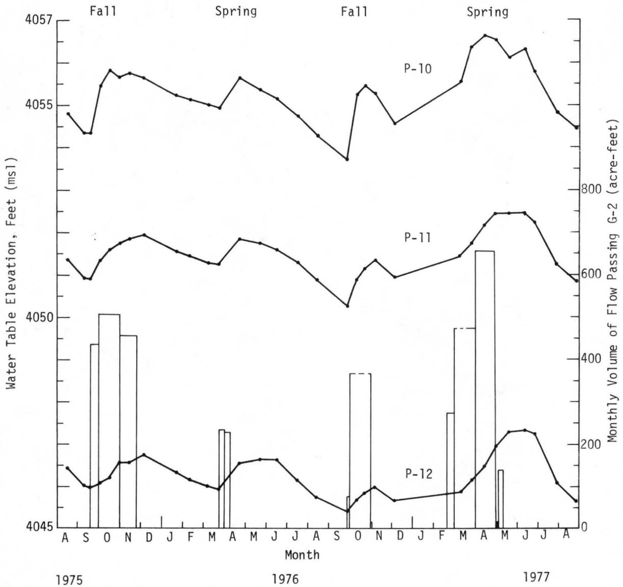
Figure 9. Water Table Hydrographs for Selected Observation Wells With Bar Graphs of Recharge Flows
