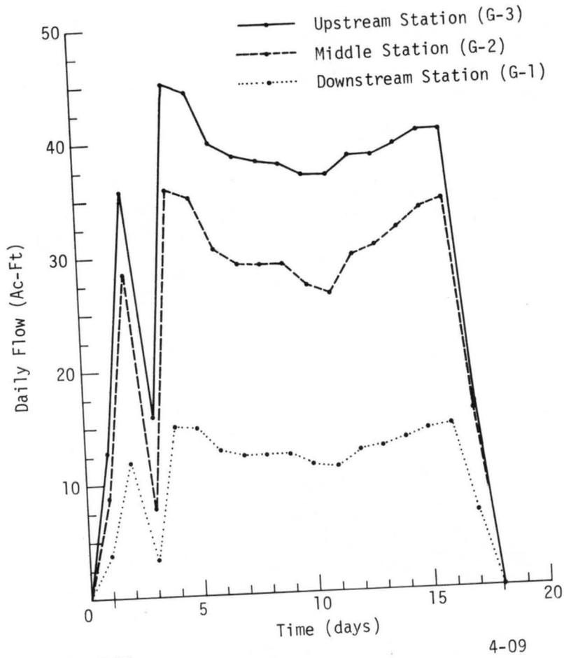
Figure 6. Sand Hill Lateral Hydrographs for Spring 1976
