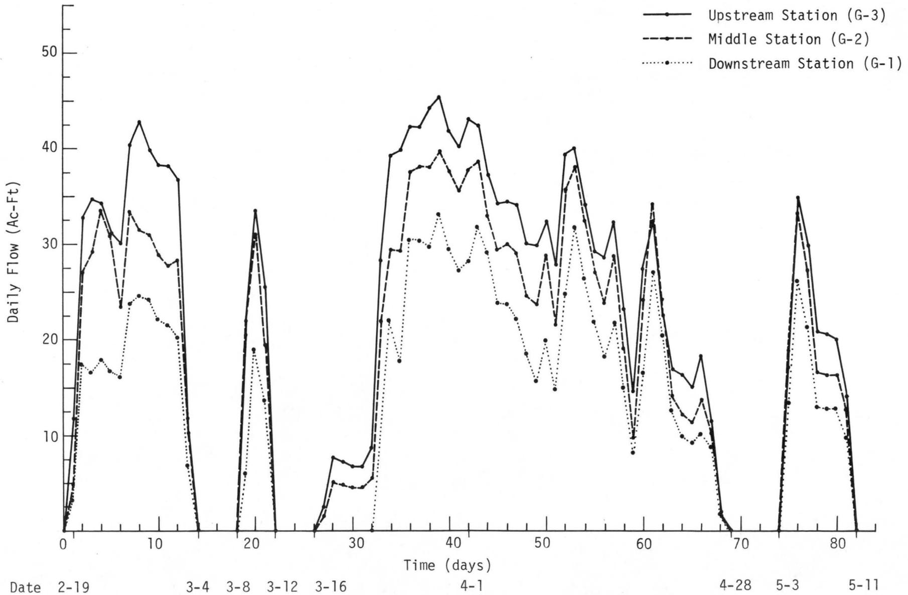
Figure 8. Sand Hill Lateral Hydrographs for Spring 1977
