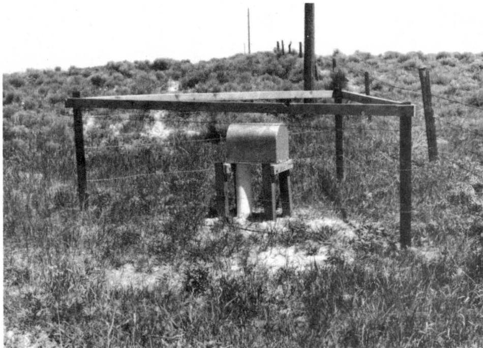
Figure 4. Observation Well with Recorder.
