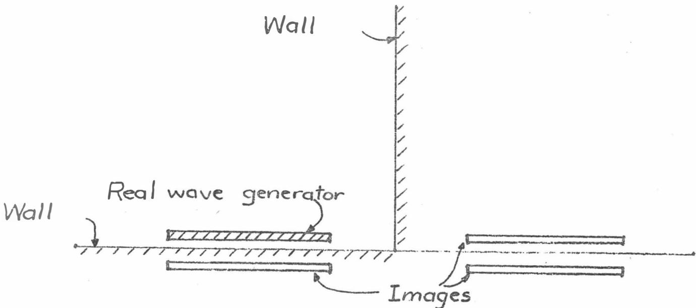
Fig. 5. Wave generator in a corner.
