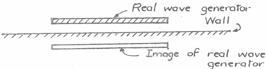
Fig. 4. Wave generator near a wall.
