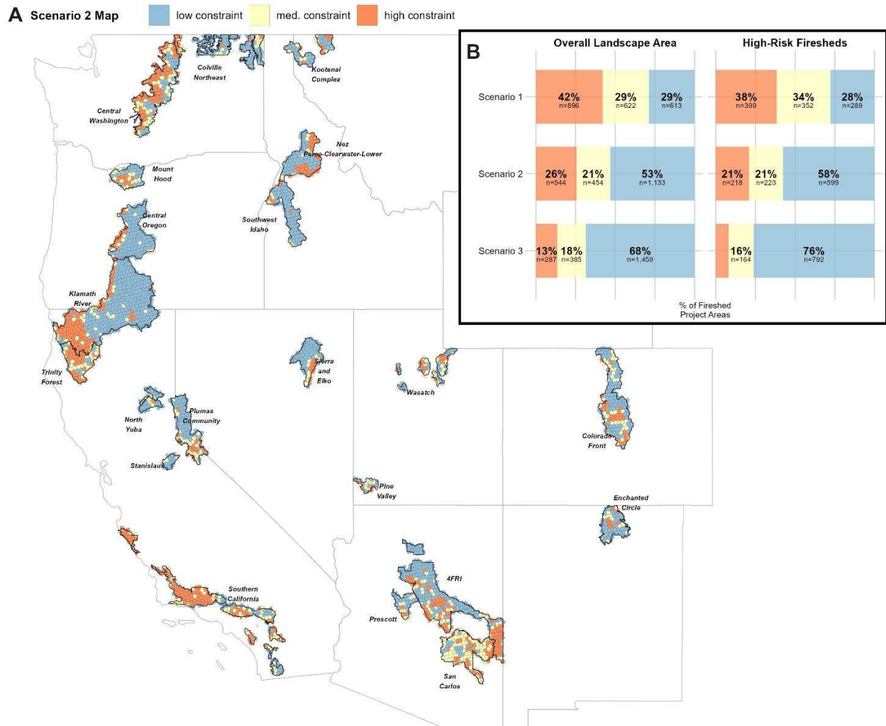
Figure 1.4. Fireshed project areas were divided into three classes of mechanical constraint: high (81–100% constrained; 0–19% available for mechanical treatment), medium (60–80% constrained; 20–40% available), and low (0–59% constrained; 41–100% available). (A) Fireshed project areas in USFS Wildfire Crisis Strategy priority landscapes were mapped and shaded by level of constraint under scenario 2 mechanical constraints. (B) The distribution of fireshed project areas by level of constraint was determined within the overall landscape area and within high-risk firesheds only.
