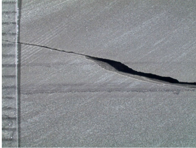
Figure A11: Massive gray-green siltstone with rare continuous gradational-bounded OM-rich shale laminations, dark gray; 517-4.
