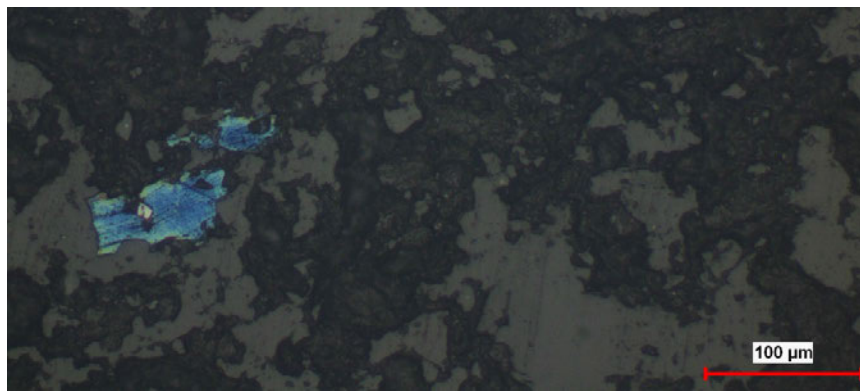
Figure A48: Covellite matrix grain suspended in calcite vein PPL and REFL. Sample SF-5B2.
