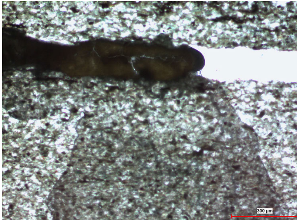
Figure A62: PPL shrinkage cracks are apparent at one end of the solid bitumen mass - which may suggest that this is pyrobitumen, cf. Rasmussen and Buick (2000). Note also the dark gray translucent stain, potentially representing bitumen expelled in association with shrinkage crack contraction. Sample LIR 2.
