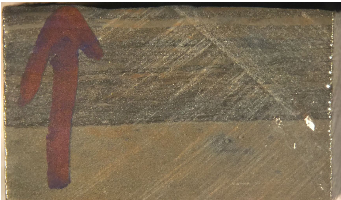
Figure A15: Hand sample showing brown clay-rich layers. Field of view is 5 cm wide. Sample 517-6.
