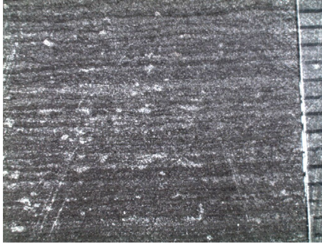
Figure A29: Irregular to wavy parallel, very thin black shale laminae with crudely-laminated, calcareous, silty gray laminae, and f.g. shaley gray very thin lams of phyllosilicates. Gray-white calcareous concretions throughout distort laminations, and are sub 2 mm maximum dimension. Thin laminations, continuous except for the silty gray laminae, some of which are discontinuous. Millimeter ruled scale at R. Sample PC5-8.
