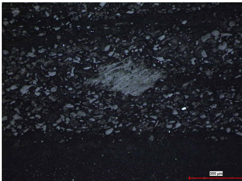
Figure A31: PPL shows calcite concretion at center, with brightly reflecting yellowish opaque chalcopyrite present, replacing v.f.g. round pyrite grains. Chalcopyrite is most apparent as miniscule bright yellow flecks (under 5 micron diameter) at margin of calcite mass at center. Sample PC5-8.
