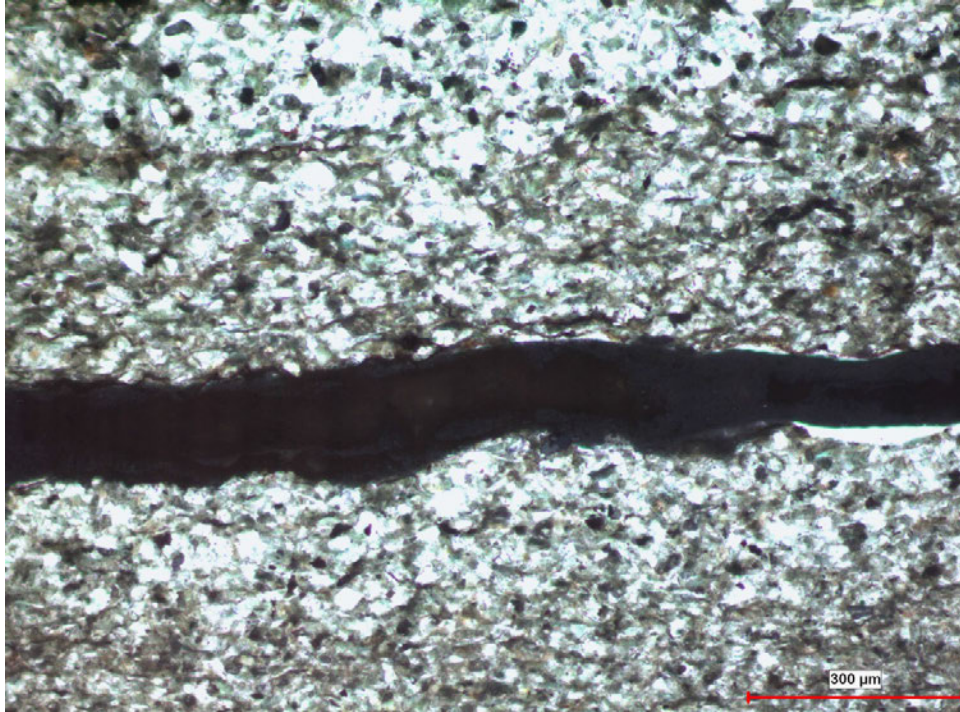
Figure A61: REFL PPL solid bitumen in lamination concordant mass, showing highest reflectivity coincident with highest opacity. Sample LIR 2.
