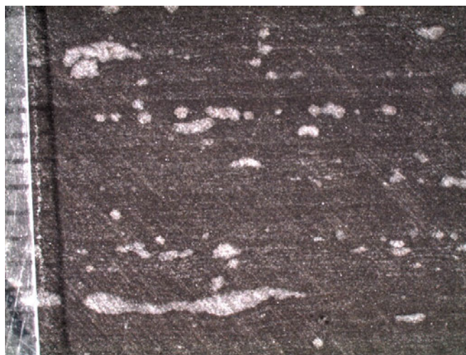
Figure A19: Hand sample with mm scale at L of calcareous concretions distorting but concordant with silt and shale laminae. Sample 523-1.
