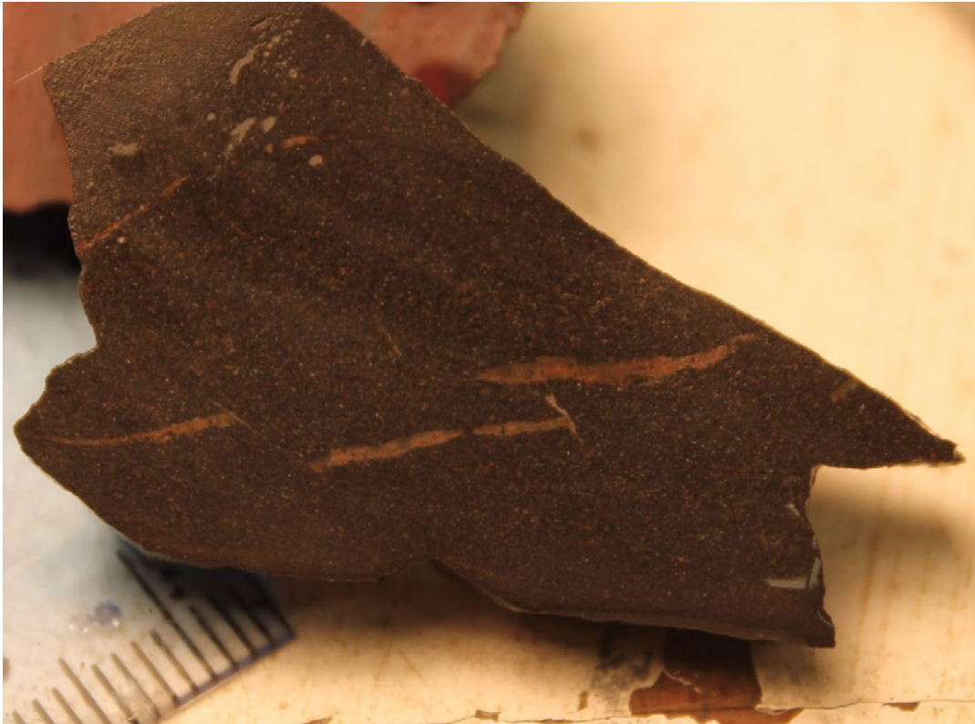
Figure A47: Hand sample showing massive bedded en echelon hematitic calcite veined siltstone. Sample SF-5B2:
