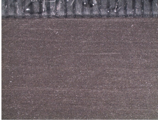
Figure A17: Hand sample with mm scale, of chalcopyritic dark gray thinly wavy discontinuous laminated shaly siltstone. Sample 523-4.
