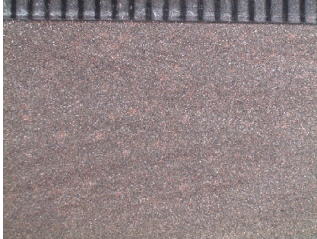
Figure A16: Dominantly massive siltstone with visible crossbedding and pinkish calcite cement in isolated sub mm concentrations. Scale is mm ruled, top. Sample 523-8.
