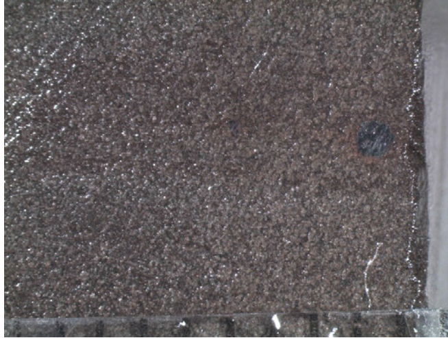
Figure A24: Hand sample with mm scale at bottom showing 9 mm diameter chalcocite nodule and crudely laminated siltstone substrate. Sample PC1-6.
