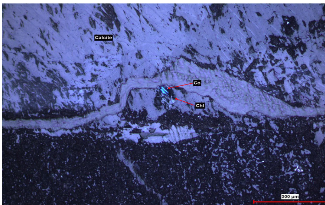
Figure A70: XPL and REFL – chlorite partially encasing an anhedral covellite grain, in association with vein calcite. Sample BIR 10.
