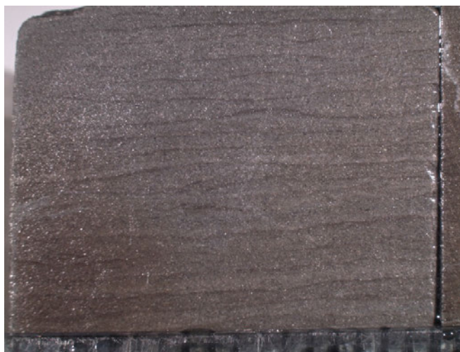
Figure A2: Halved core sample of laminated shaly siltstone with mm scale at bottom. Light colored laminae are composed primarily of quartz silt. Darker laminae are composed of clay, mica, pyrite and OM. The opaque appearance of the darker layers is due in part to the presence of small spherical framboids of pyrite that are 10-20 microns diameter and concentrated in OM rich laminations. Sample WPB1-5.
