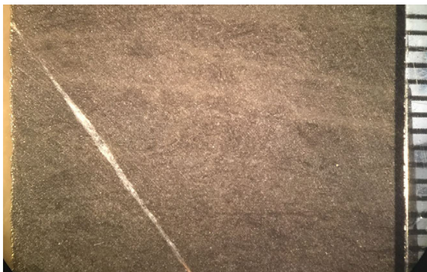
Figure A22: Hand sample with mm scale, showing one of the stable isotope sampled hematitic calcite veins oblique to bedding. Sample 523-2.
