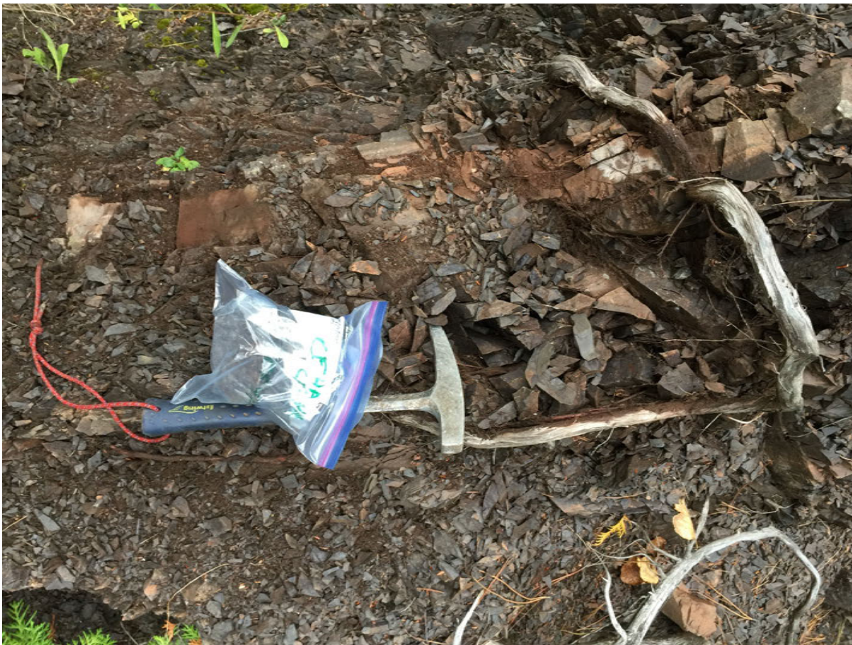
Figure 40: Fractured fissile shaley siltstone at Copper Falls, Bad River, WI. The majority of samples from this site were too broken to collect as singular specimens.
