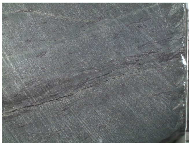
Figure A3: Wet sediment deformed greenish gray micaceous siltstone, mm scale at R. Sample WPB1-7.
