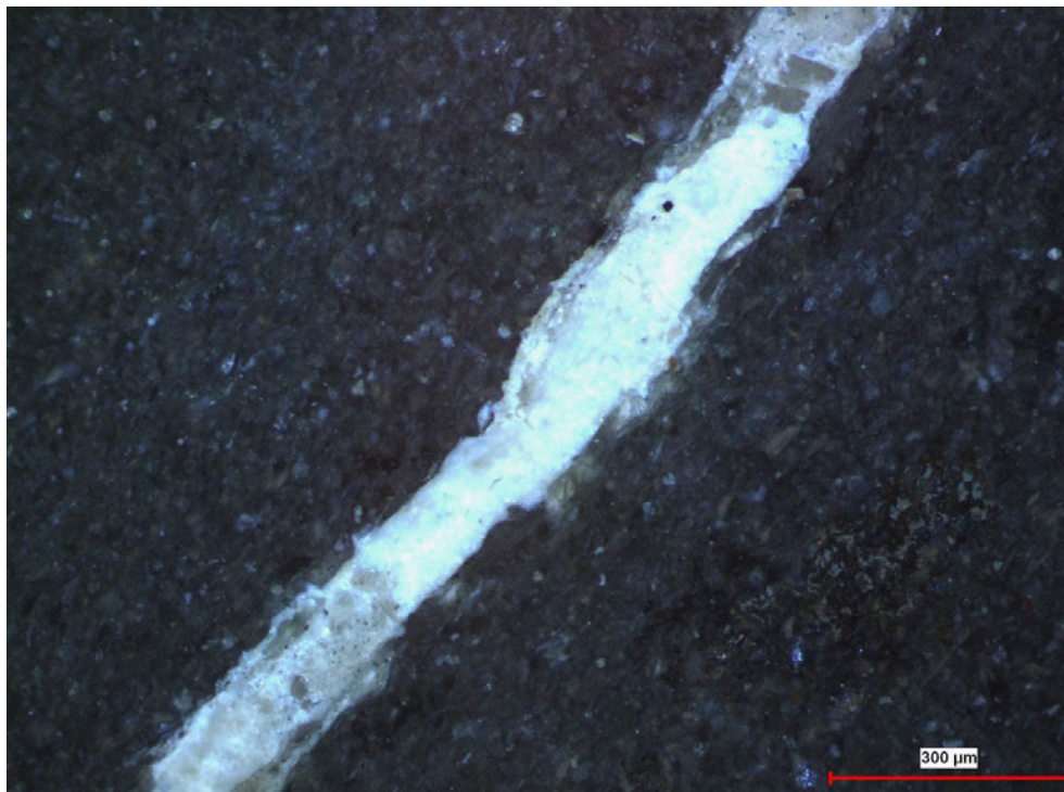
Figure A64: XPL REFL, showing subhedral chalcocite, tarnished (lower right). Sample LIR2. Note also anisotropy of the bituminous lamellar mass, as compared to Figure A65.
