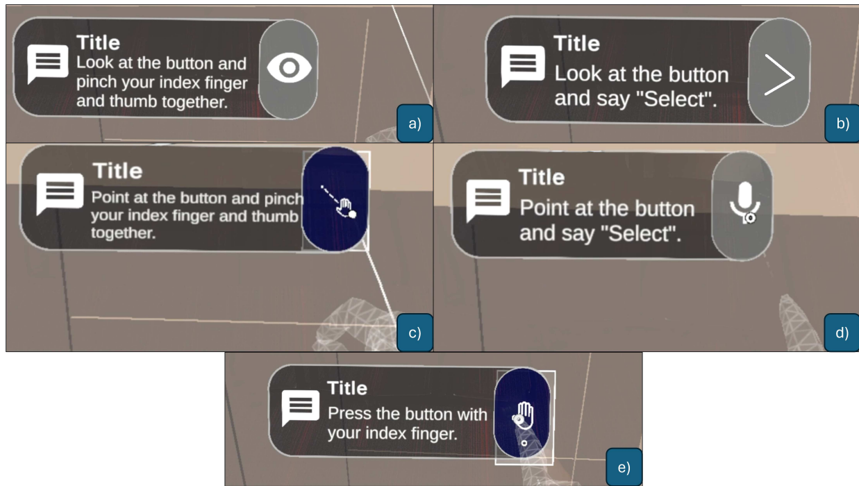
Fig. 3: Interaction techniques used in the experiment: a) Gaze and Pinch; b) Gaze and Speech; c) Point and Pinch; d) Point and Speech; e) Touch
