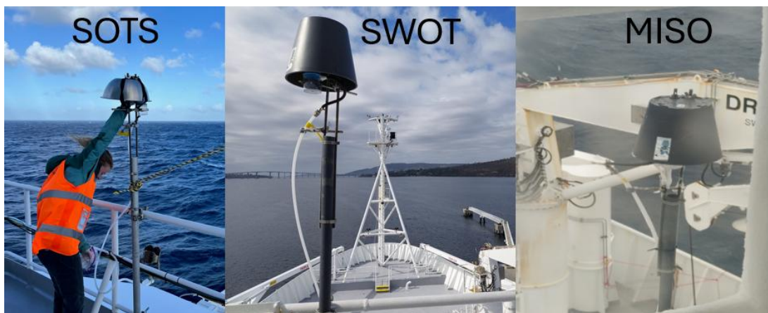
Figure 13. INP tower set-ups onboard the RV Investigator for SOTS, SWOT, and MISO voyages. Note that the aerosol lab inlet is also pictured at the front of the bow in the SWOT image.
