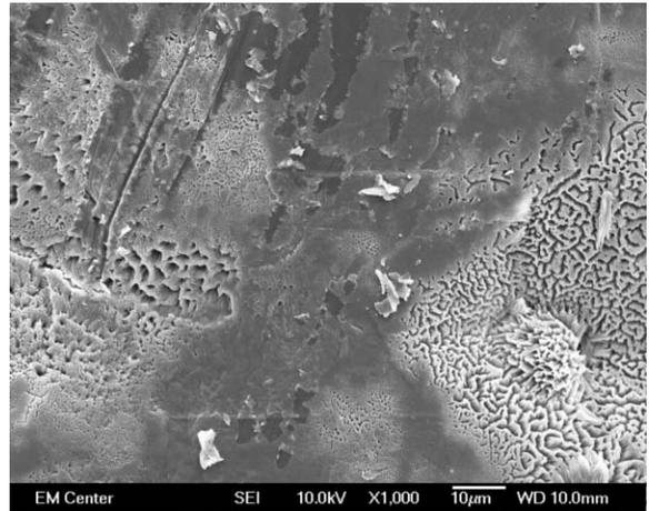
Figure 4-17: SEM image of DSPC test 16 imaged at 10 kV, 1,000X original magnification. E-field 0.67 kV/cm, voltage 8 kV, E-sprayed for 4.5 mins.
