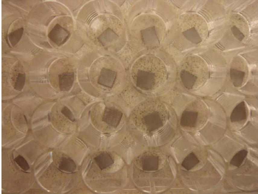
*Figure 5-22: Photograph showing DOPS/cholesterol week 2 end-point. Note near complete retention of coatings of coatings in upper 3 rows (containing GS).*
