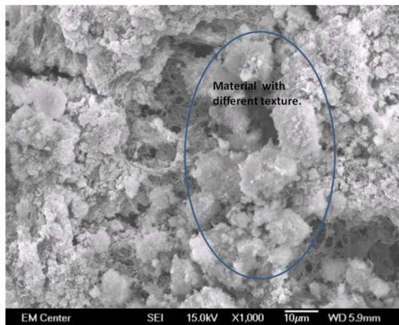
*Figure 7-70: SEM image of **DOP/GS week 1**, imaged at 15 kV, 1000X original magnification. Thick coating remains, with two distinct materials.*
