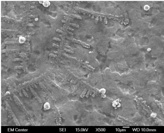
*Figure 5-25: SEM image of calcium-chloride pretreated titanium with DOPS with cholesterol without GS, imaged at 15 kV.*
