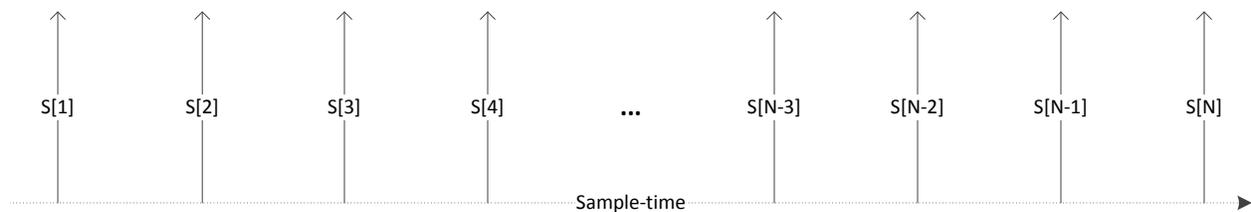
**Figure 6.2:** Receive pulses in sample-time for one range bin in the single polarization processing modes.
