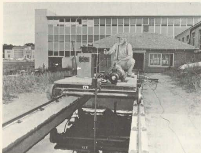
Fig. 3.3. Electrically propelled tow car.
