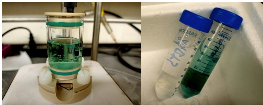
Figure 24 Electrodes not electrochemically active still exhibit signs that laccase enzymes are present on the electrode. Whether they were directly bound versus adsorbed is unknown
