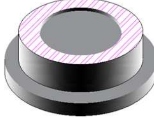
Cap top view - hatched area shows upper surface.
