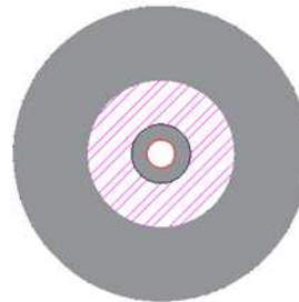
Base bottom view - empty red circles represent tapped hole for bleed screw, lowest face of base is represented as hatched surface for clarity only.
