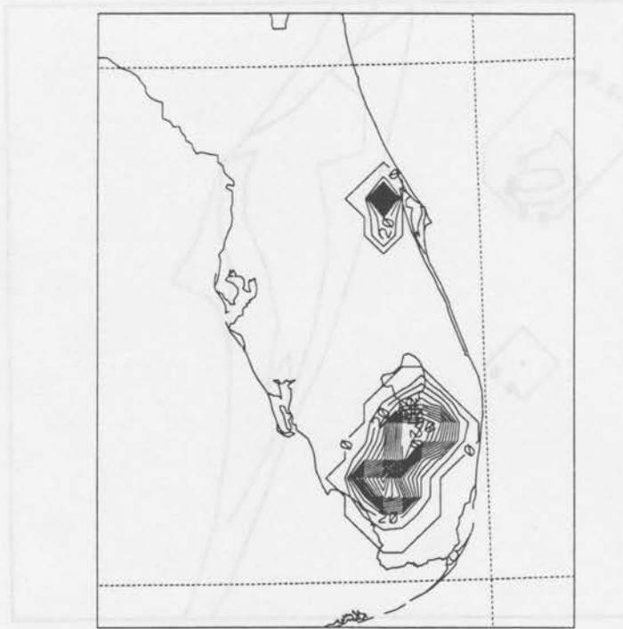
Figure 3.30: Condensate mixing ratio (g/g), elevation = 48.6 m contour = 1 E-5 g/g, maximum contour = 14 E-5 g/g; 21Z 29 July
