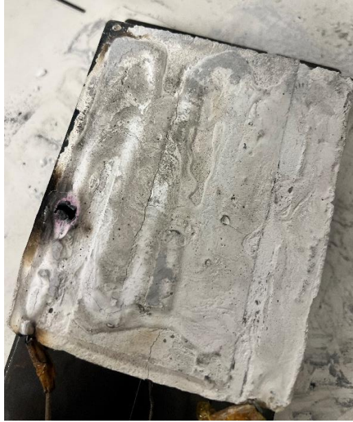
Figure 1: Heater Failure due to air bubble
