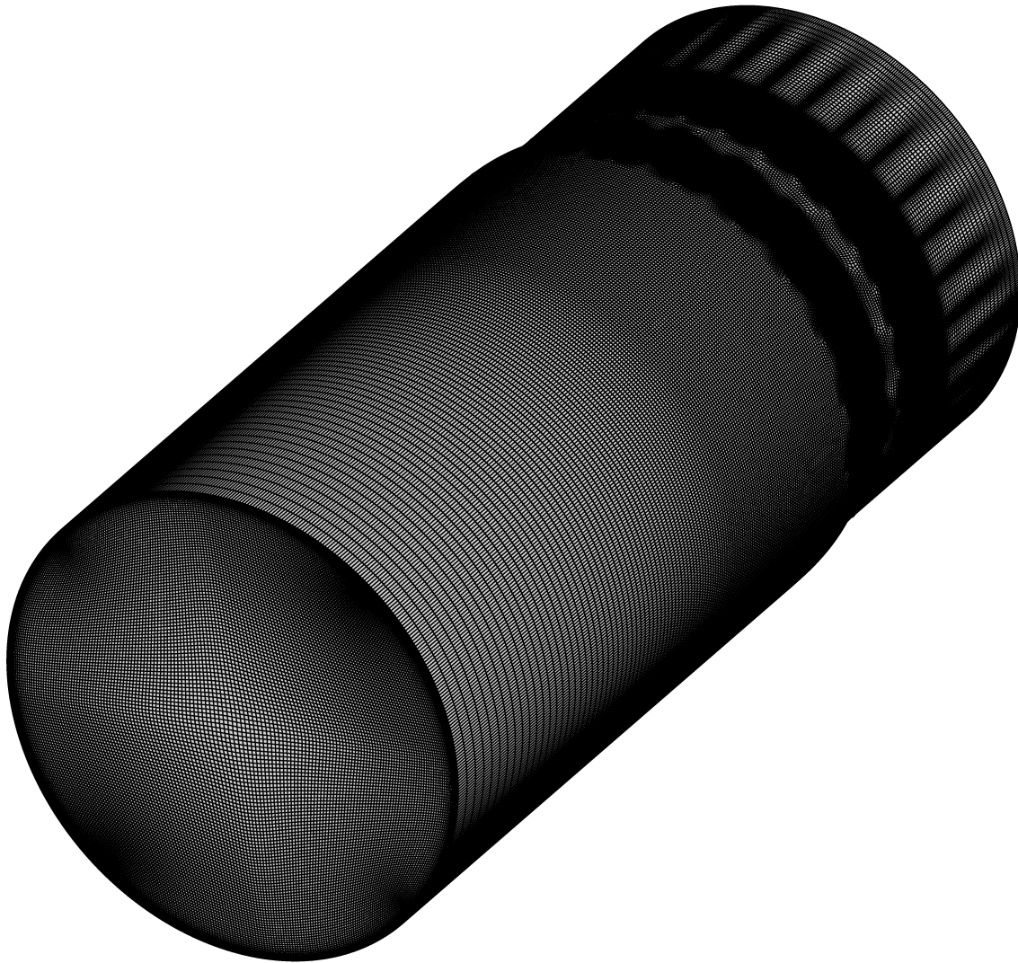
FIGURE 2.13. Isometric view of full-annulus grid used for URANS simulations with circumferential distortion.
