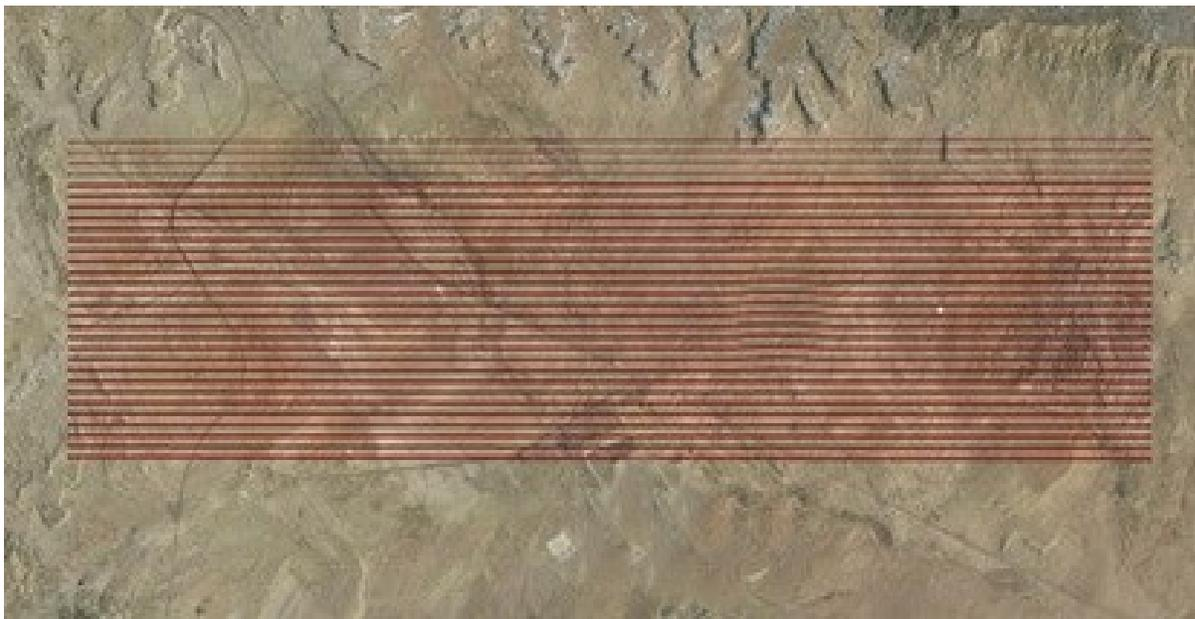
Figure 4: 16 km × 4.8 km (10 mile × 3 mile) flight grid of the ASPECT aircraft over the Uranium mine. Flight spacing was 152 m.
