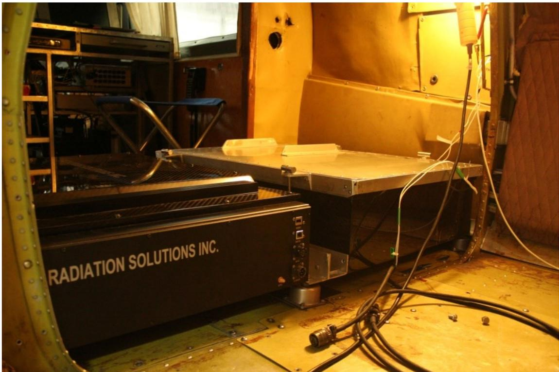
Figure 7: RadAssist radiation detectors mounted in the tail section of the aircraft
