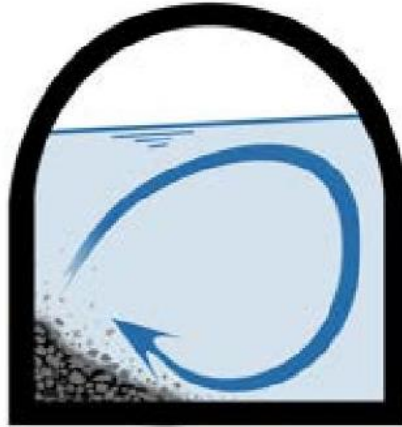
Figure 4. Sketch from Solis physical model report. The sketch shows the effect of secondary flow and primary flow on sediment transport at an SBT bend. (Solis 2010)
