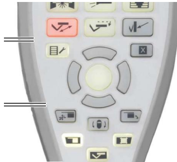
Figure 21: Pendant Controls for Treatment Fields
