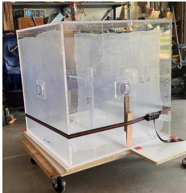
Figure 11: cementing the top sheet to rest of tank (tank is laying upside down on top of sheet).
