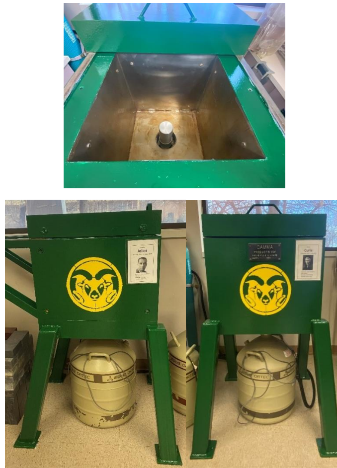
Figure 4: HPGe detectors used in this report, named Joliot and Curie.
