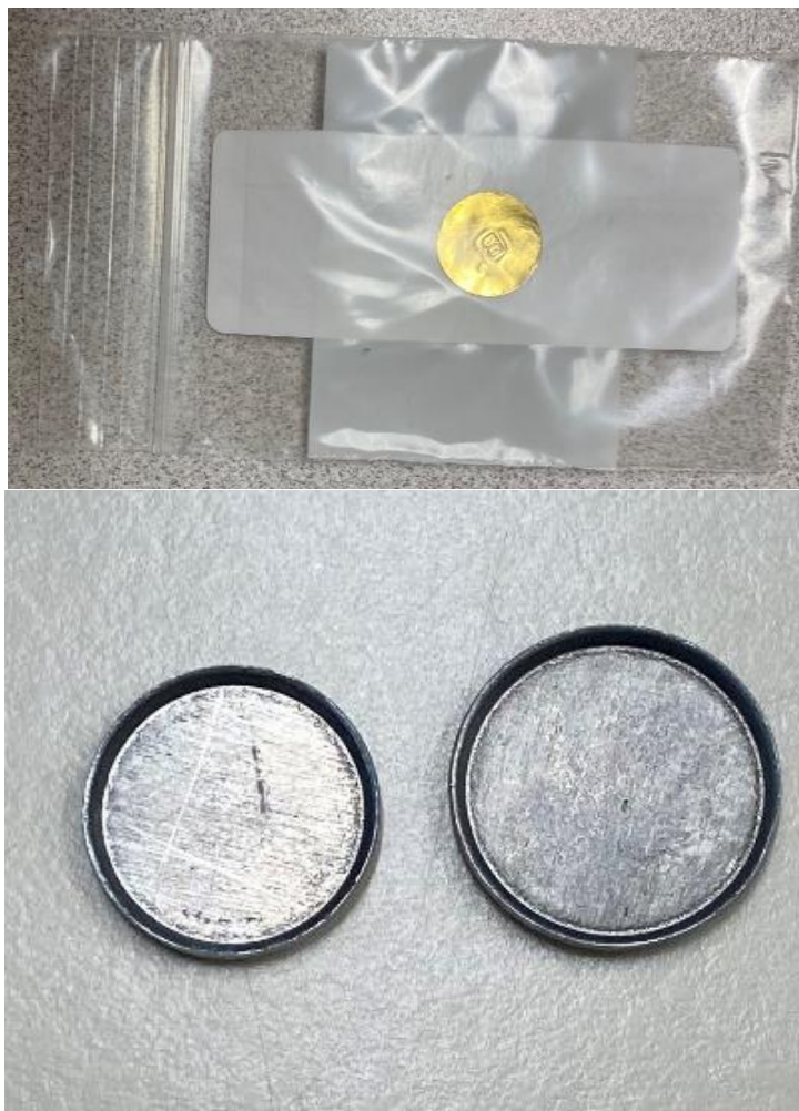
Figure 6: Gold foil used in NAA of 1 cm diameter and Cd covering.
