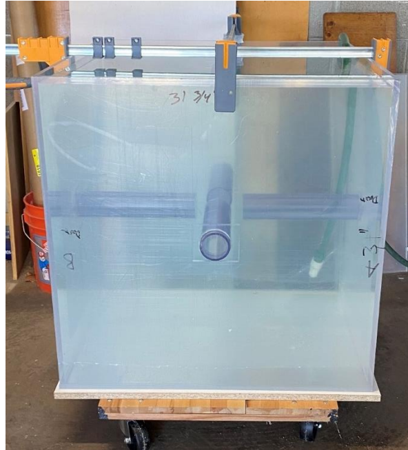
Figure 10: Leak testing tank full of water before adhering top sheet on tank. After letting the full tank rest for a couple of days, all joints and edges were checked for leakage. No deformations or leaks were spotted.
