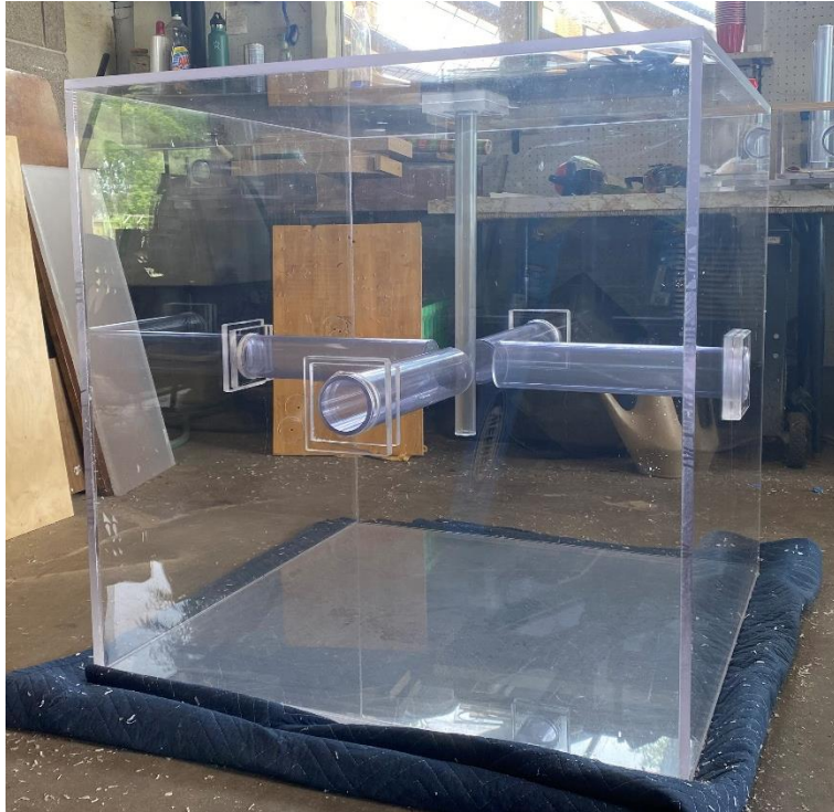
Figure 12: Final additions to tank were completed and protective film removed from the main body.
