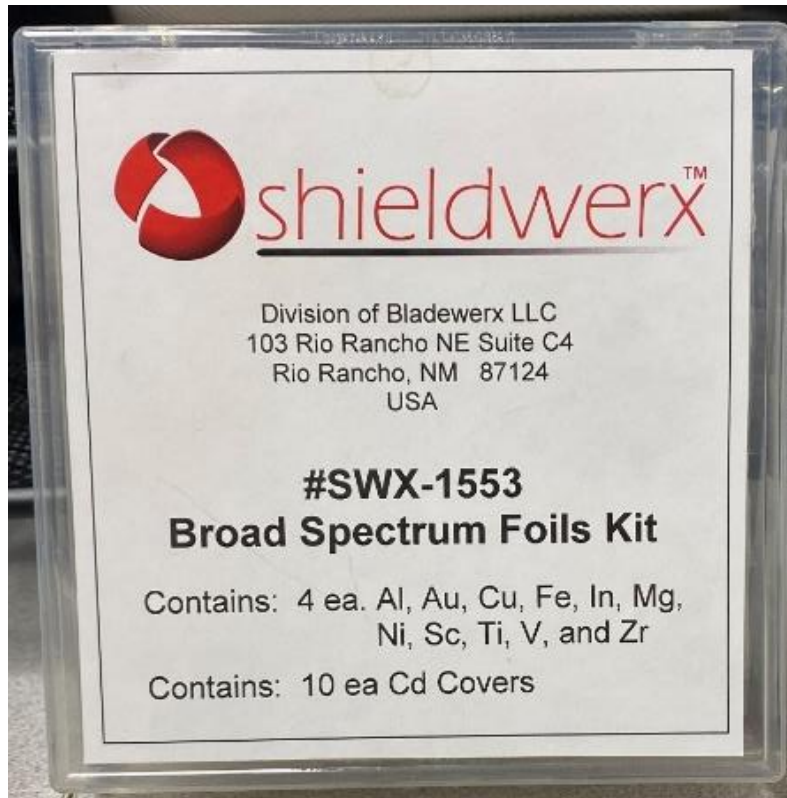
Figure 5: Activation foil kit used for NAA.
