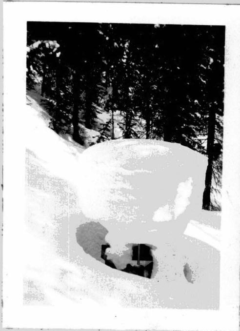
Figure Three - A Sacramento gage fitted with an Alter snow shield. The throat of the gage has capped over, preventing further catch of precipitation.
