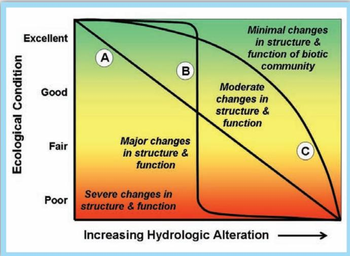
Figure 1. This chart illustrates three of several possible forms of flow alteration-ecological response relationships: linear (A), threshold (B), and curvilinear (C). The form of the curve depends on the specific ecological and hydrological variables analyzed. (TNC 2008)
