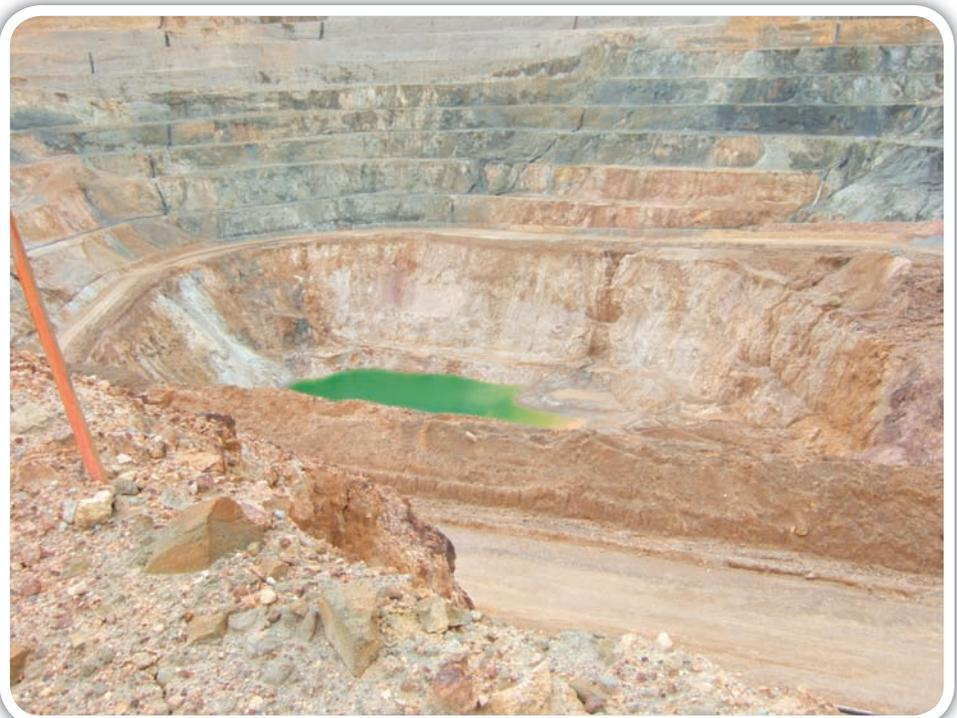
*The effluence of groundwater results from mining excavations at the Yanacocha Mine, partially located at the headwaters of the Mashcon and Chonta Rivers in south Cajamarca, Peru.*
