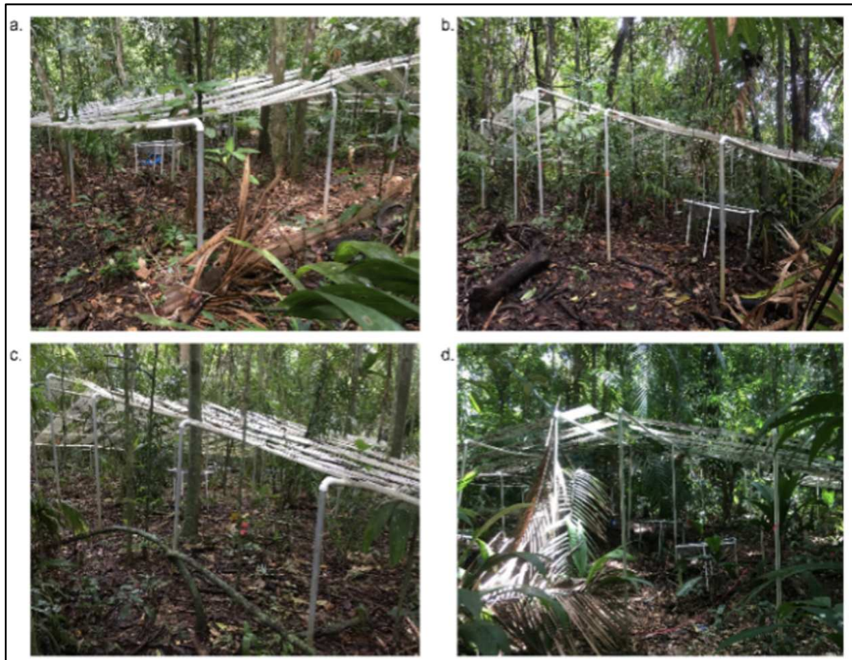
Figure 3: Partial throughfall exclusion structures are shown at the four PARCHED forest sites. a) Gigante; b) P12; c) P13; d) Sherman Crane
