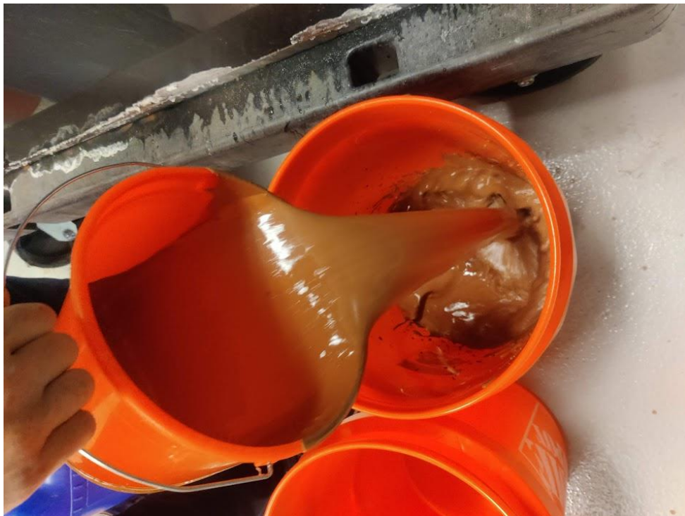
Transfer of claystone slurry to buckets
