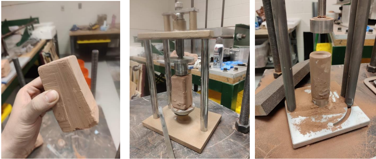
Sanding down the intact rock to cylindrical shape
