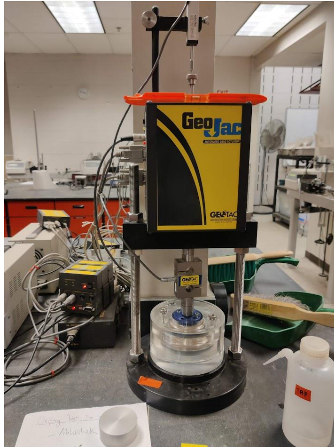
1-Dimensional consolidation test of remolded sample in Geojac
