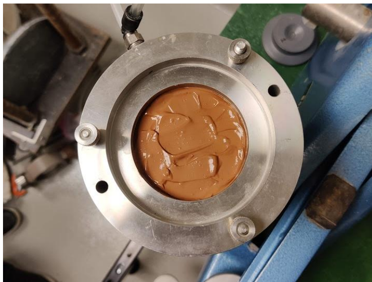
Slurry claystone for 1-dimensional in conventional oedometer
