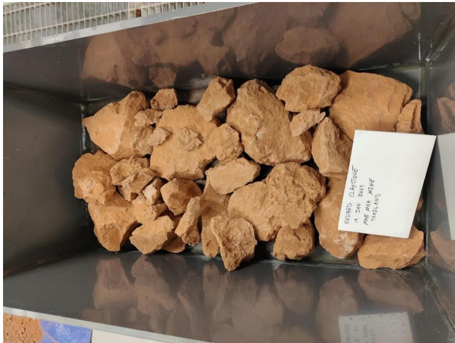
Intact Redbed Claystone Prior to Wetting
