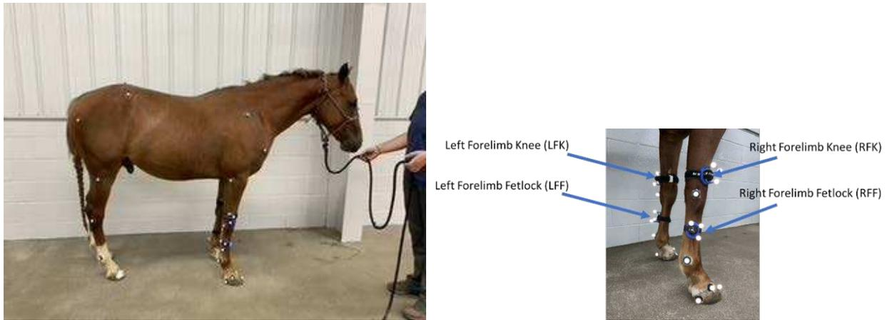
**Figure 5.1:** Placement of four MoveSense IMU sensors on the left and right fetlock, as well as just above the left and right knee of the horse.
