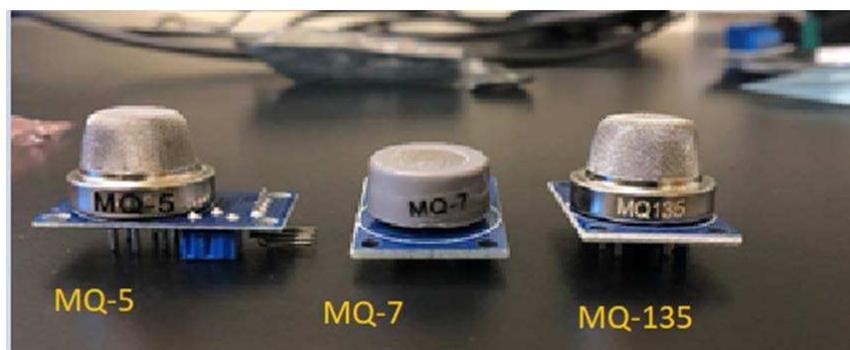
**Figure 6.1:** MQ sensor series used for this study, including the MQ-5, MQ-7, and MQ-135.
