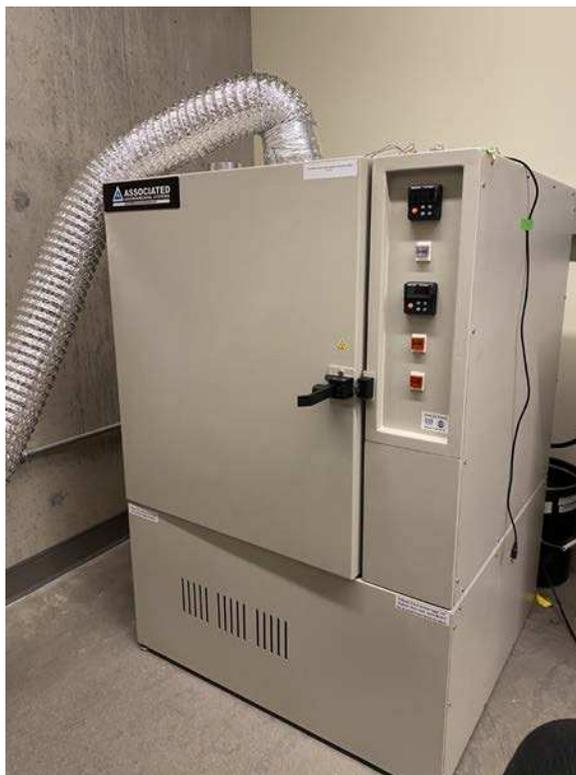
**Figure 6.2:** Environmentally controlled chamber selected for this study, The LHE-6 Stability Benchtop-Style Test Chamber from Associated Environmental Systems (AES).
