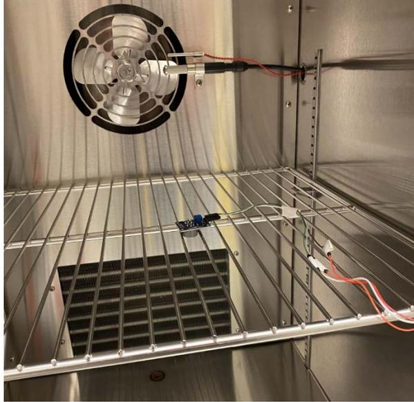
**Figure 6.3:** Sensor placement inside of environmentally controlled chamber.
