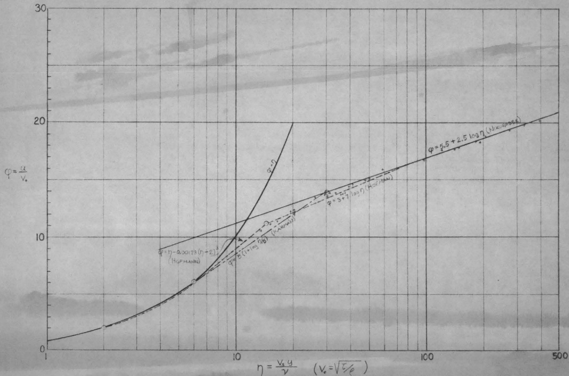
FIG. 1 COMPARISON OF KARMAN'S AND HOFMANN'S VELOCITY DISTRIBUTIONS FOR TURBULENT FLOW WITH NIKURADSE'S DATA
