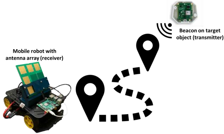
Figure 2.1. Configuration of proposed setup of Bluetooth homing controller.
