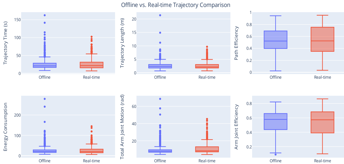
Figure 5.5. Comparison of performance metrics between offline and real-time simulated trajectories.
