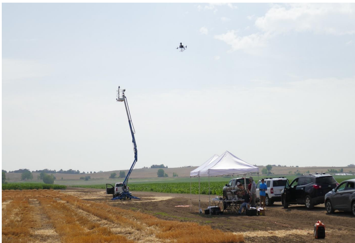
Figure A1.3. Sampling setup and demonstration of location for elevated field trials used in chapter 2. Samplers were located at the Colorado State University Agricultural Research, Development, and Education Center (ARDEC). Samplers were placed in an agricultural area on the side of a empty field and gravel road. The Full SASS was placed on the boom lift and the Light SASS was placed on the drone (DJI Matrice 350 quadcopter pictured).
