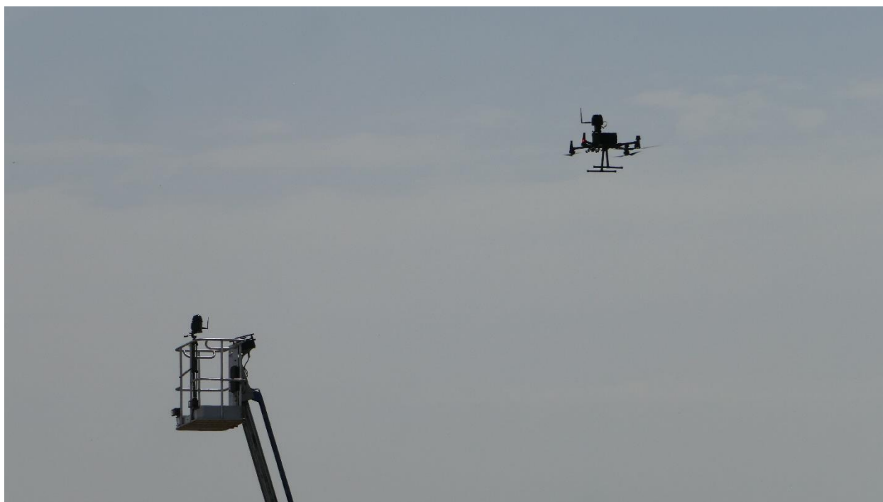
Figure A1.5. Close up image of sampling setup and demonstration of location for elevated field trials used in chapter 2. The Full SASS was placed on the boom lift on the left side of the image and the Light SASS was placed on the drone on the right side of the image (DJI Matrice 350 quadcopter pictured).
