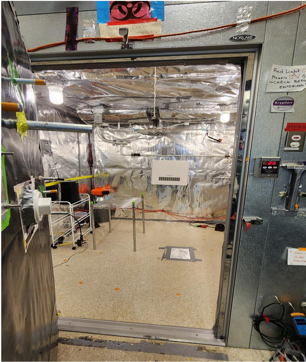
Figure A1.1. Sampling setup and demonstration of location for chamber trials used in chapter 2. The chamber is a sealed 10m 3 location allowing for the nebulization of tracer organism in a controlled environment. Both the Full SASS and Light SASS were setup on the metal table to the left of center in the room.
