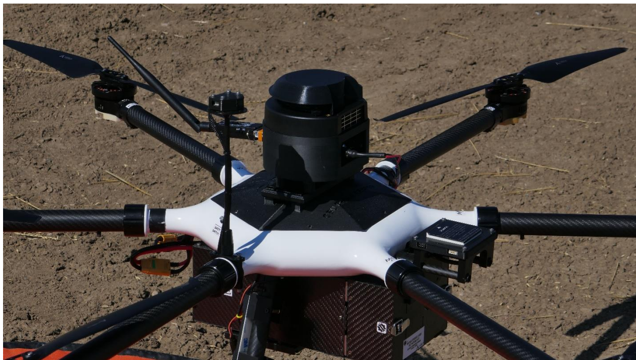
Figure A1.7. Detailed image of Light SASS air sampler setup on the Aurelia X6 Pro V2 hexacopter drone. Both the drone and the sampler were thoroughly cleaned to reduce the chance of contamination.
