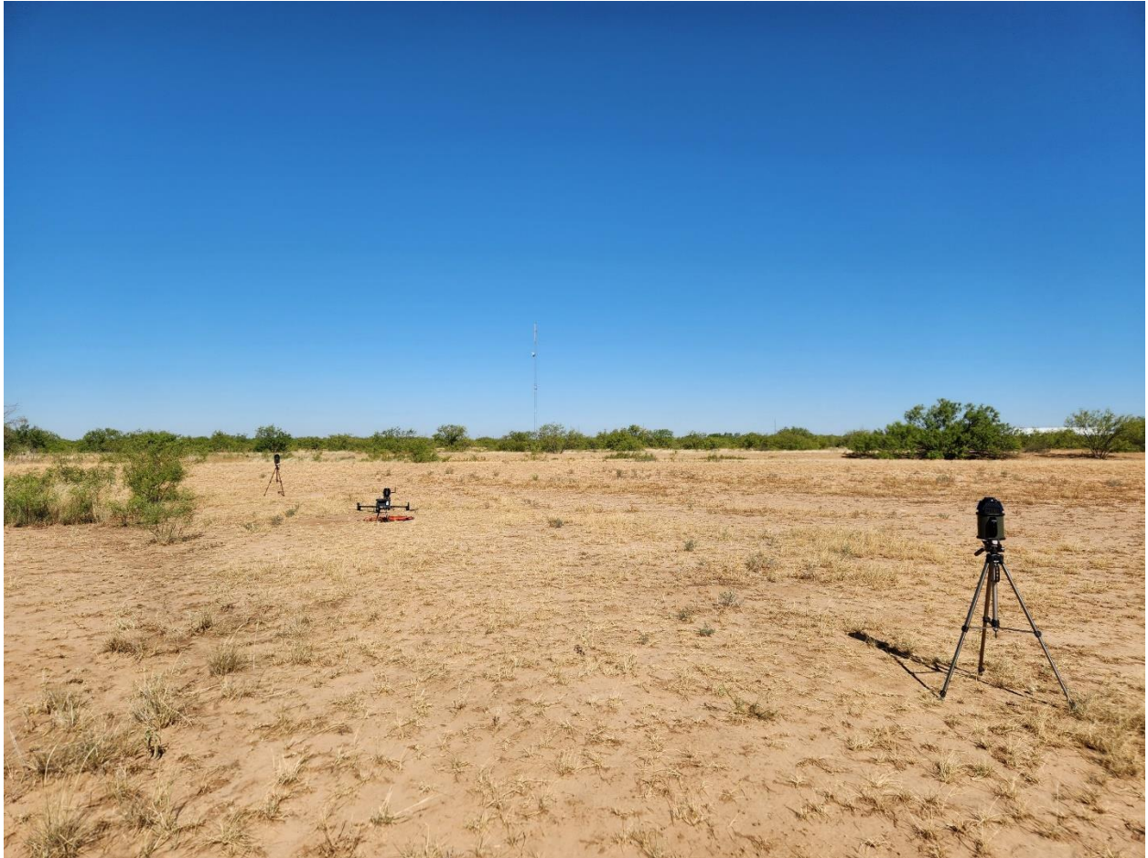
Figure A2.1. Sampling setup and demonstration of location during field sampling. Ground-level samplers were set up 25 feet away from the drone landing pad, seen in the center. The ground-level tripods were equipped with the Full SASS 3100, while the drone was equipped with the Light SASS prototype. Sight conditions were arid to semi-arid, with dry soil and sparse vegetation.
