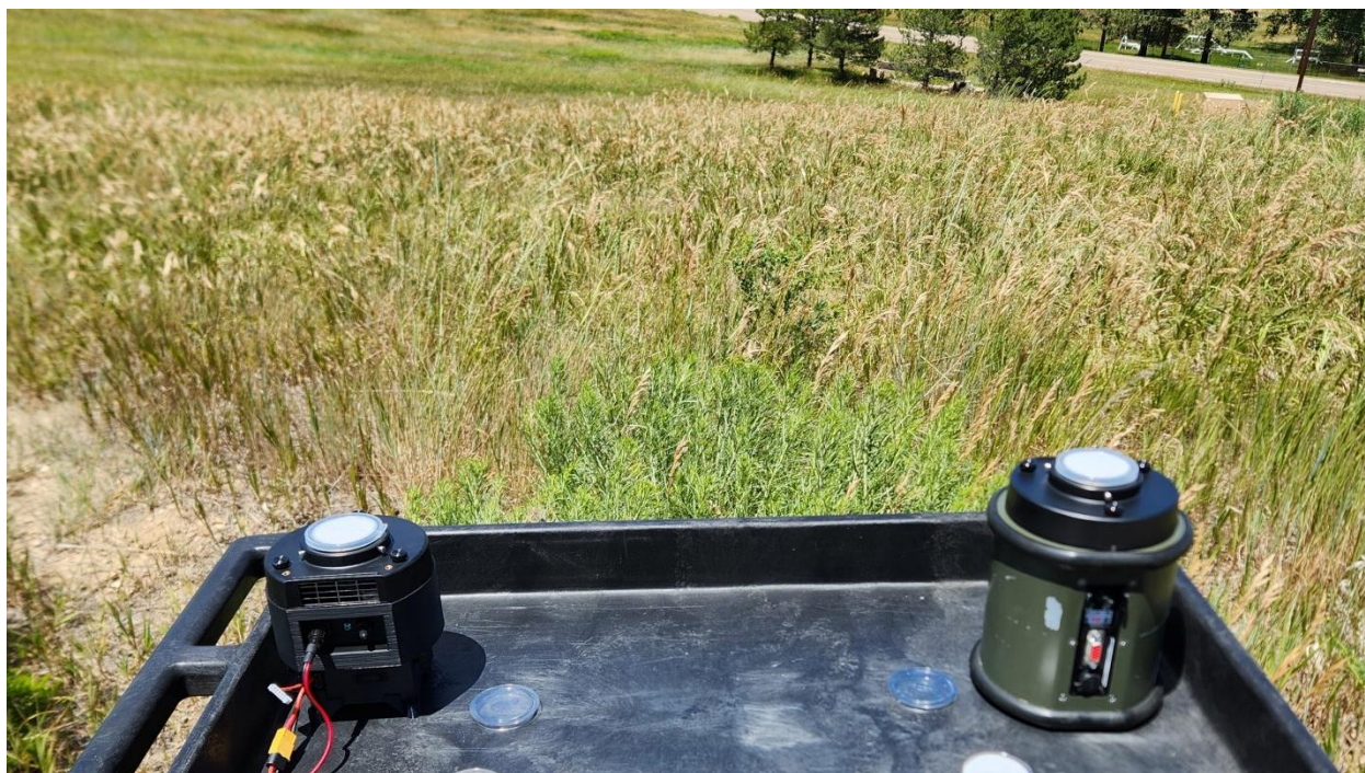
Figure A1.2. Sampling setup and demonstration of location for ground-level trials used in chapter 2. Samplers were located at the Colorado State University Foothills Campus. Samplers were placed away from builds at the edge of a large field and approximately 4 feet off the ground and 2 feet apart.
