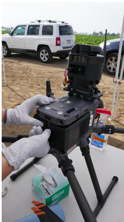
Figure A1.6. Detailed image of Light SASS air sampler setup on the DJI Matrice 350 quadcopter drone. Both the drone and the sampler were thoroughly cleaned to reduce the chance of contamination.
