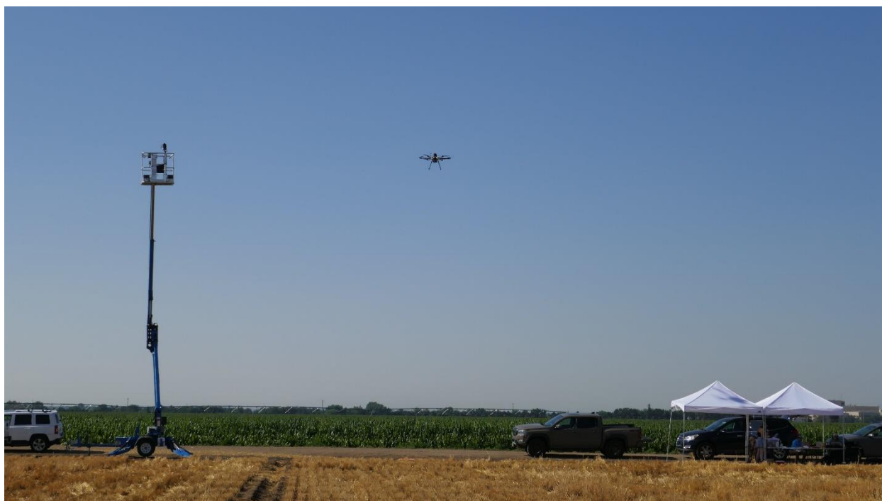
Figure A1.4. Sampling setup and demonstration of location for elevated field trials used in chapter 2. Samplers were located at the Colorado State University Agricultural Research, Development, and Education Center (ARDEC). Samplers were placed in an agricultural area on the side of a empty field and gravel road. The Full SASS was placed on the boom lift and the Light SASS was placed on the drone (Aurelia X6 Pro V2 hexacopter pictured).
