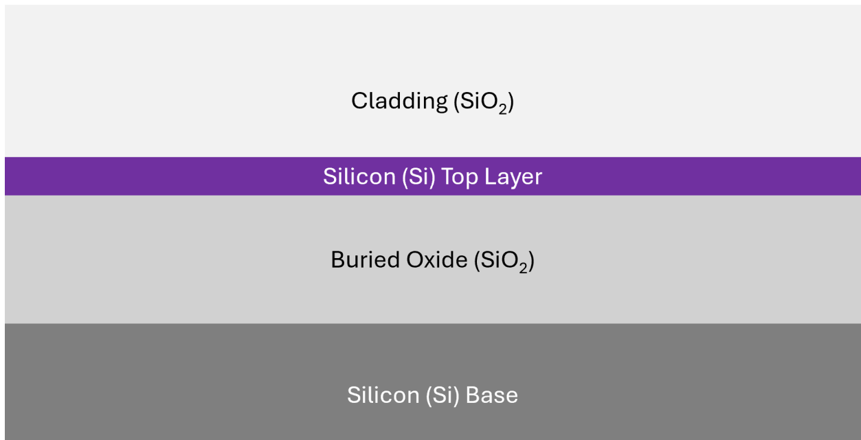
Figure 2.1: The structure of an SOI wafer. There is a silicon base, followed by an SiO 2 layer, which insulates the following Si layer. Lastly, there is a cladding layer made from SiO 2 on top.
