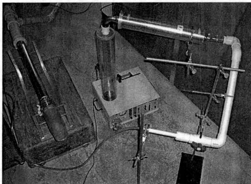
Figure 5.12. Photograph of the experimental calibration setup showing drop collection on a nylon membrane filter prior to drop injection into the axial-flow cyclone inlet.
