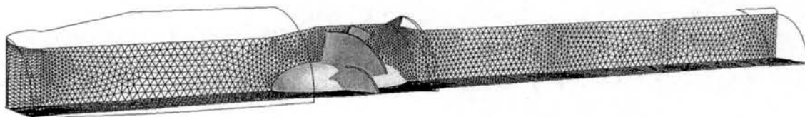
Figure 4.1. The interior flow domain of the axial-flow cyclone cloud water collector containing the curved vane assembly and the extraction slot. The use of rotationally periodic boundary conditions allowed a 90^\circ sector of the duct to be modeled.
