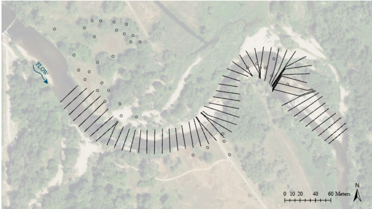
Figure 6. Cross-sections used for sediment transport analysis, dark lines are cross sections and open circles are placement of log jams.
