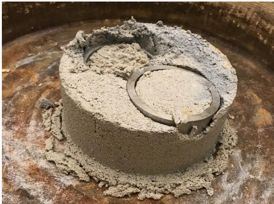
Figure A4. Hydraulic conductivity specimen being cut using cutting ring. Two sub-specimens were obtained from each hydraulic conductivity test.
