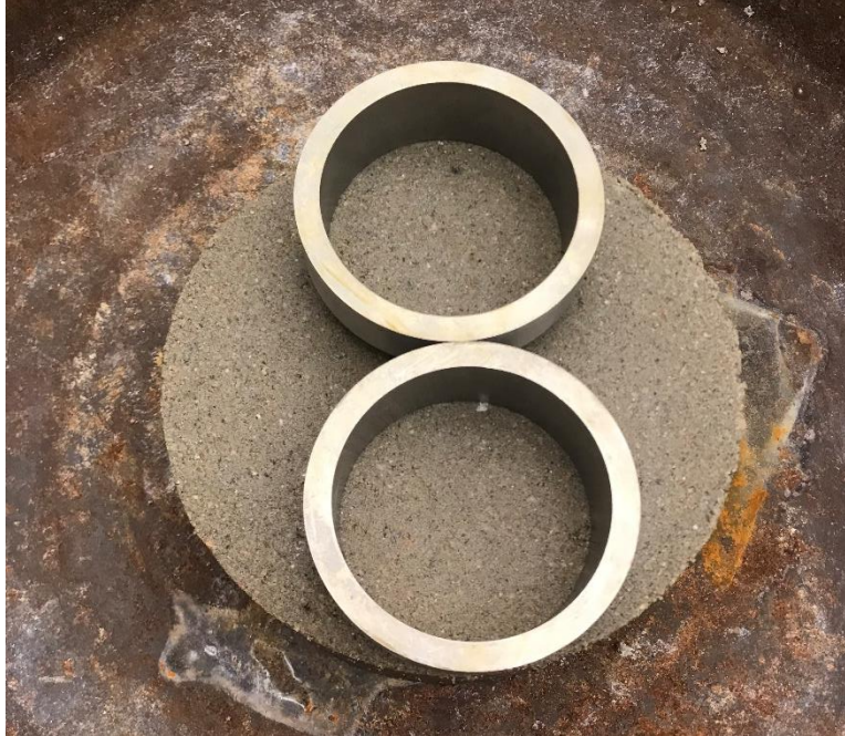
Figure A3. Specimen before using cutting-rings to extract sub-specimens. Sub-specimens were cut side by side on permeated specimens.
