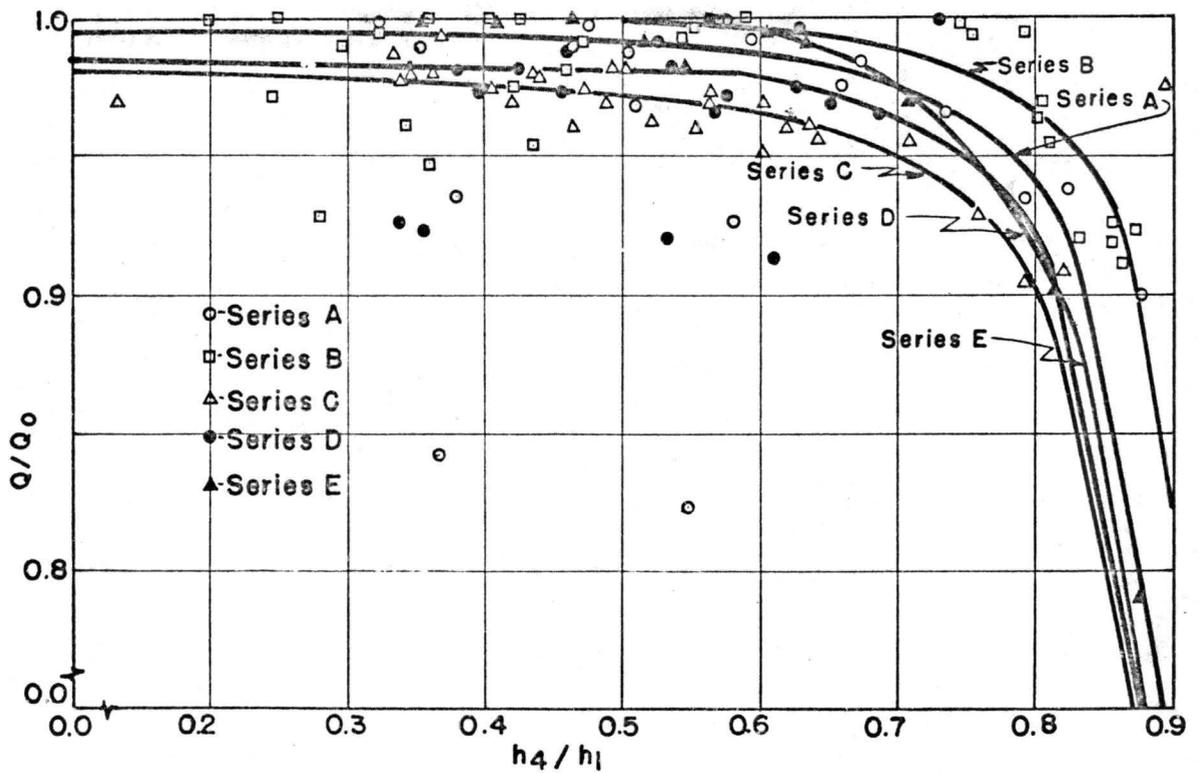
Figure 4. Submergence correction for Romijn type weir using  $h_4$  stage reading.
