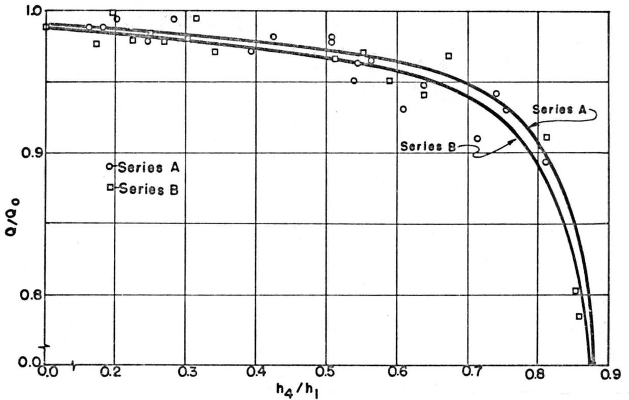
Figure 7. Submergence correction for Crump type weir using  $h_4$  stage reading.
