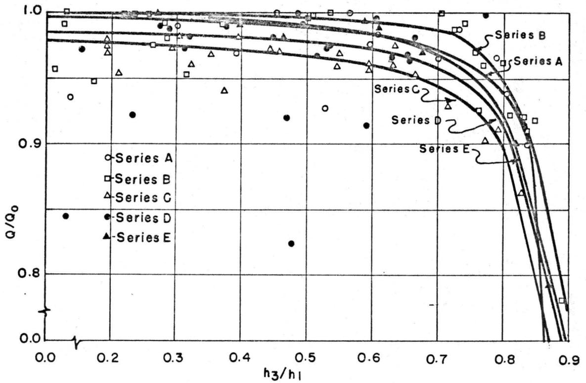
Figure 3. Submergence correction for Romijn type weir using  $h_3$  stage reading.
