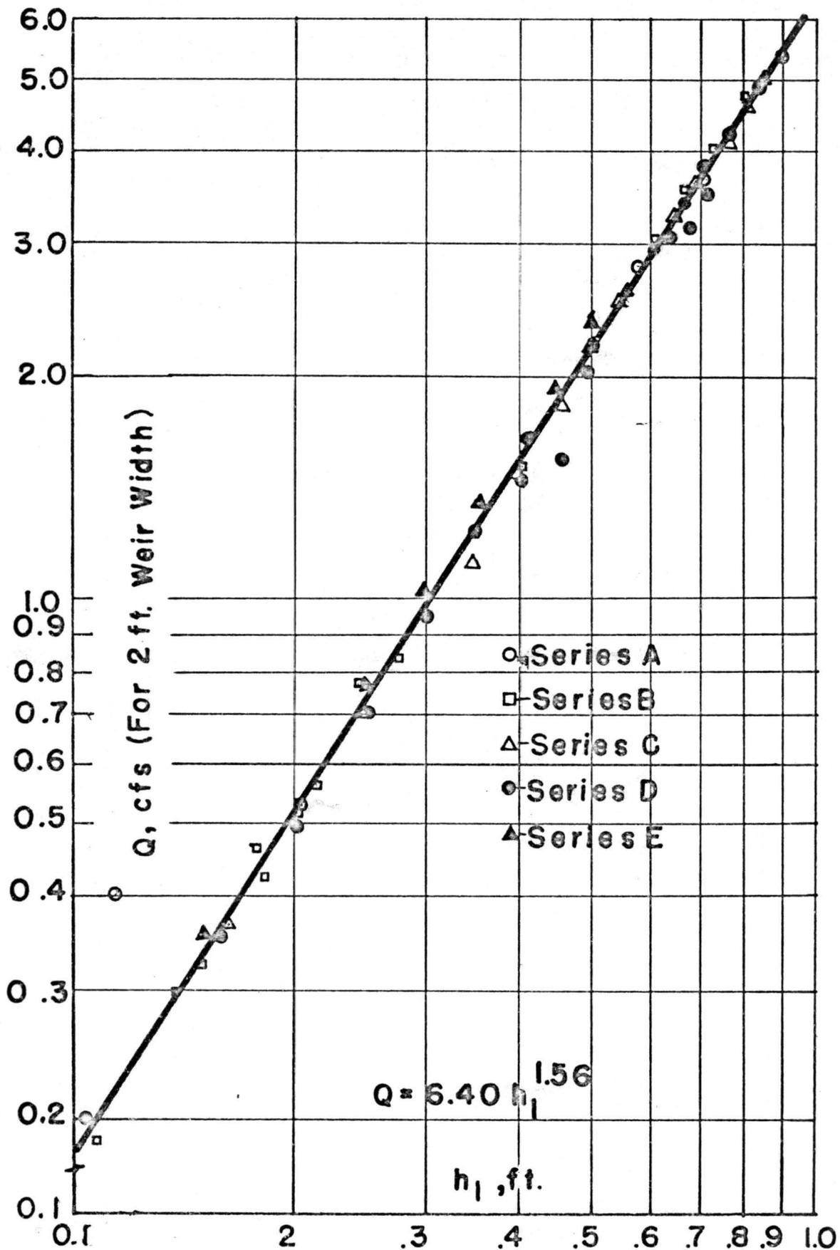
Figure 2. Calibration curve for 2-foot Romijn type weir.
