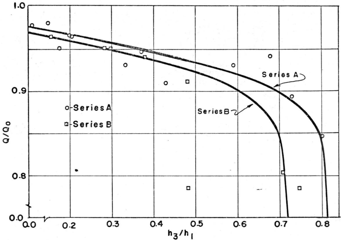
Figure 6. Submergence correction for Crump type weir using  $h_3$  stage reading.
