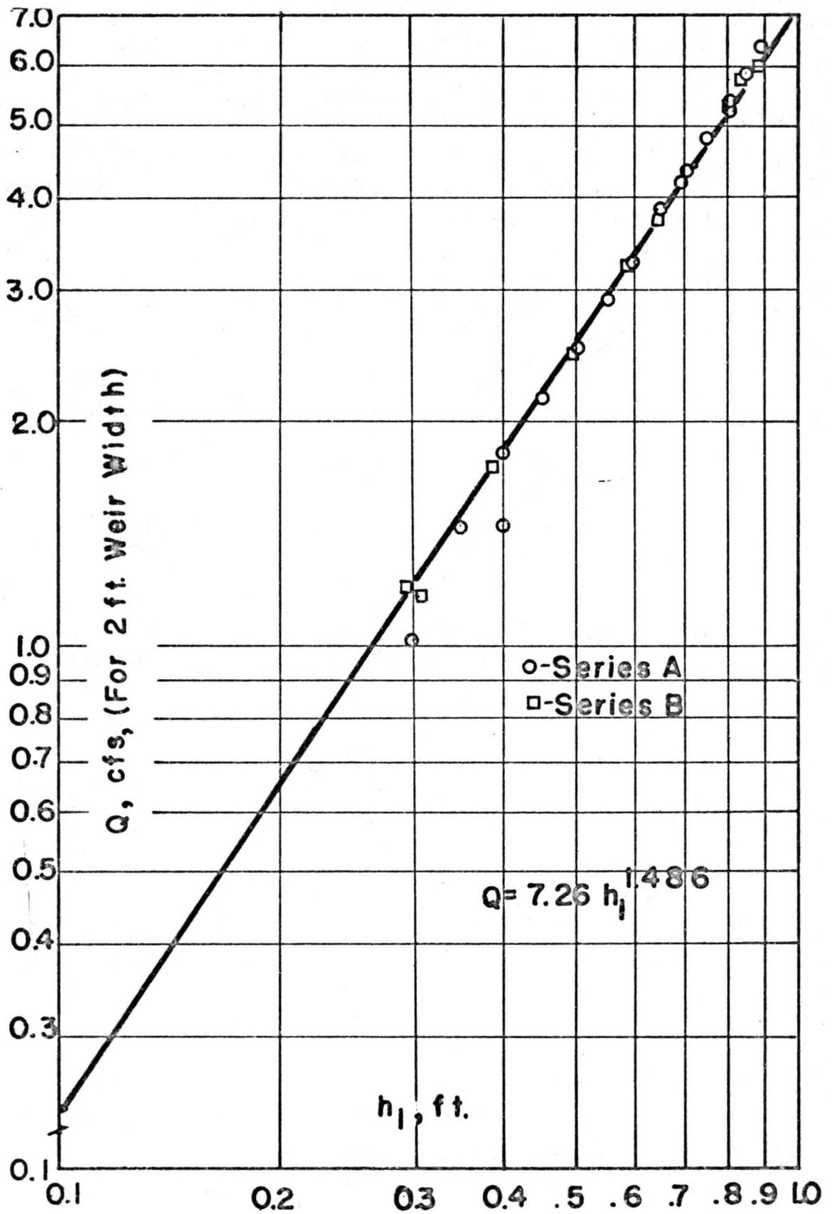
Figure 5. Calibration curve for 2-foot Crump type weir.
