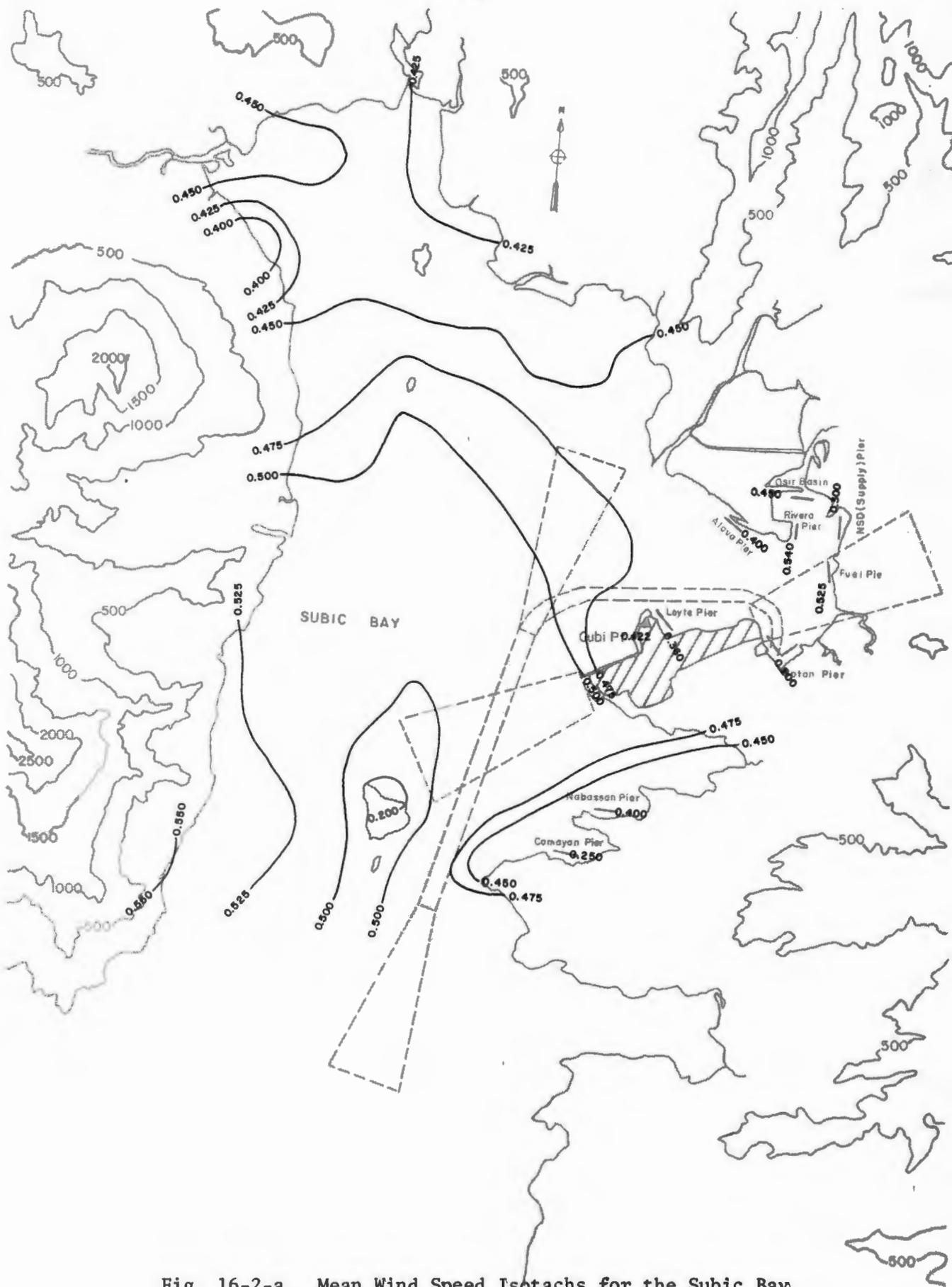
Fig. 16-2-a. Mean Wind Speed Isotachs for the Subic Bay Basin at 195°T, z = 150 ft (45.7 m)
