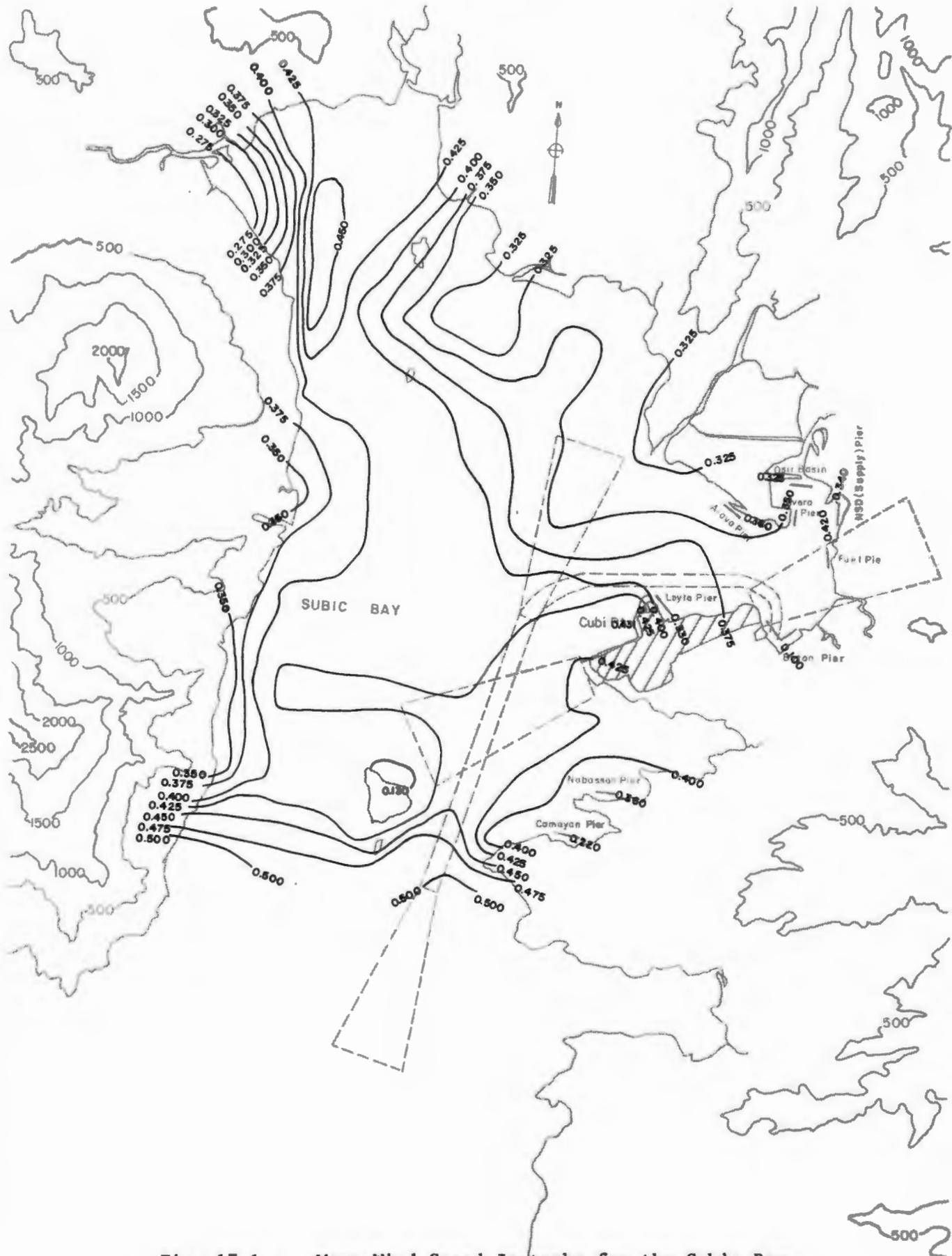
Fig. 17-1-a. Mean Wind Speed Isotachs for the Subic Bay Basin at 210°T, z = 70 ft (21.3 m)
