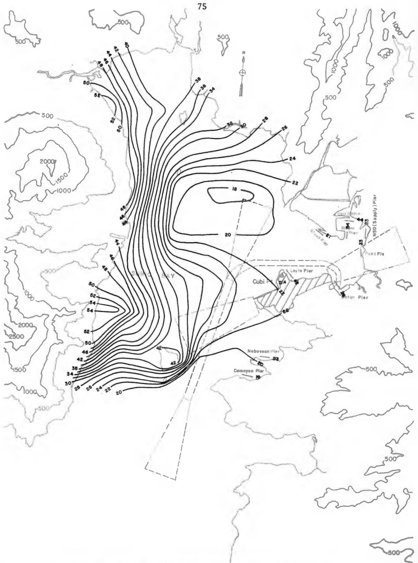
Fig. 20-2-b. Turbulence Intensity Contour Lines for the Subic Bay Basin at  $255^{\circ}T$ ,  $z = 150$  ft (45.7 m)
