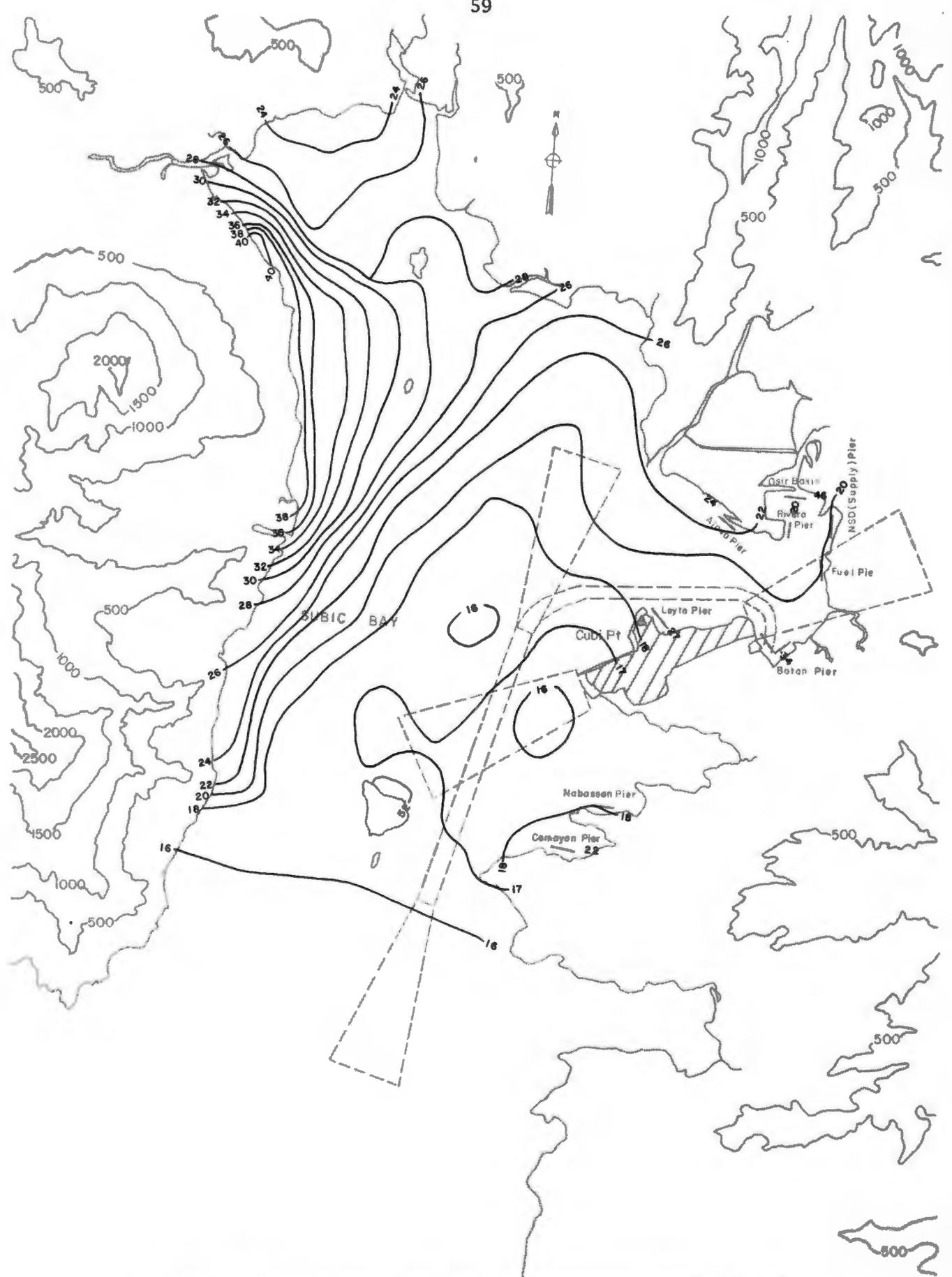
Fig. 18-2-b. Turbulence Intensity Contour Lines for the Subic Bay Basin at 225°T, z = 150 ft (45.7 m)
