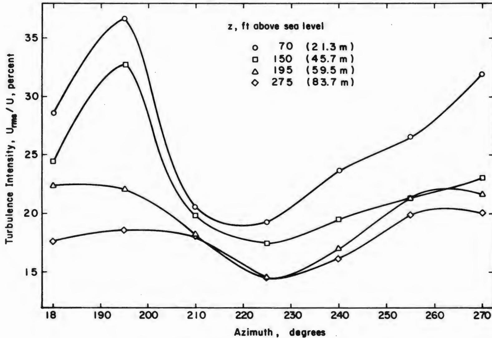
Fig. 24. Turbulence Intensity at Cubi Point Meteorological Station
