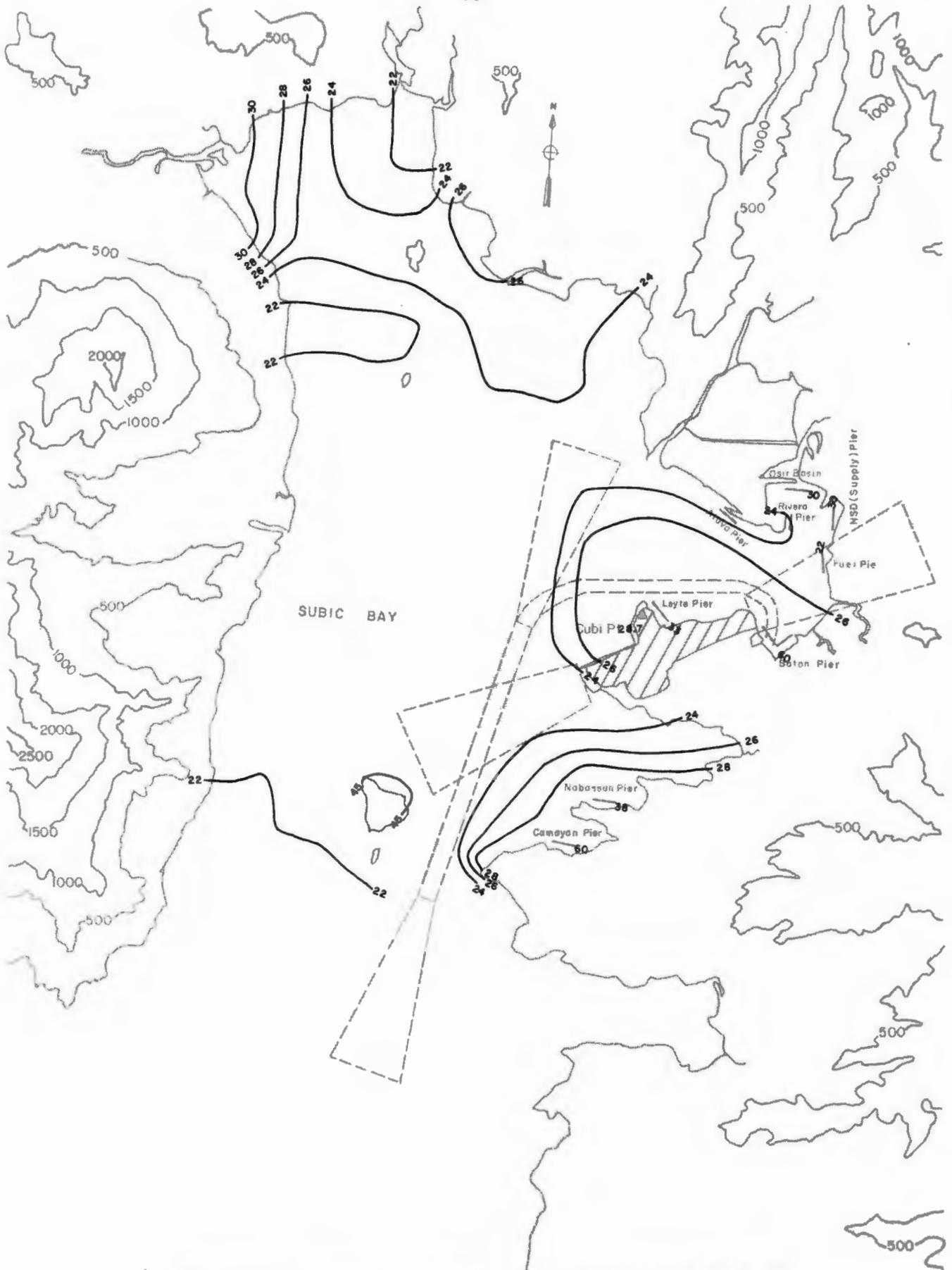
Fig. 15-1-b. Turbulence Intensity Contour Lines for the Subic Bay Basin at 180°T, z = 70 ft (21.3 m)
