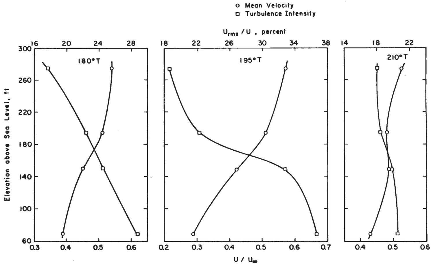
Fig. 22-a. Mean Velocity and Turbulence Profiles at Cubi Point Meteorological Station at 15 Degree Intervals
