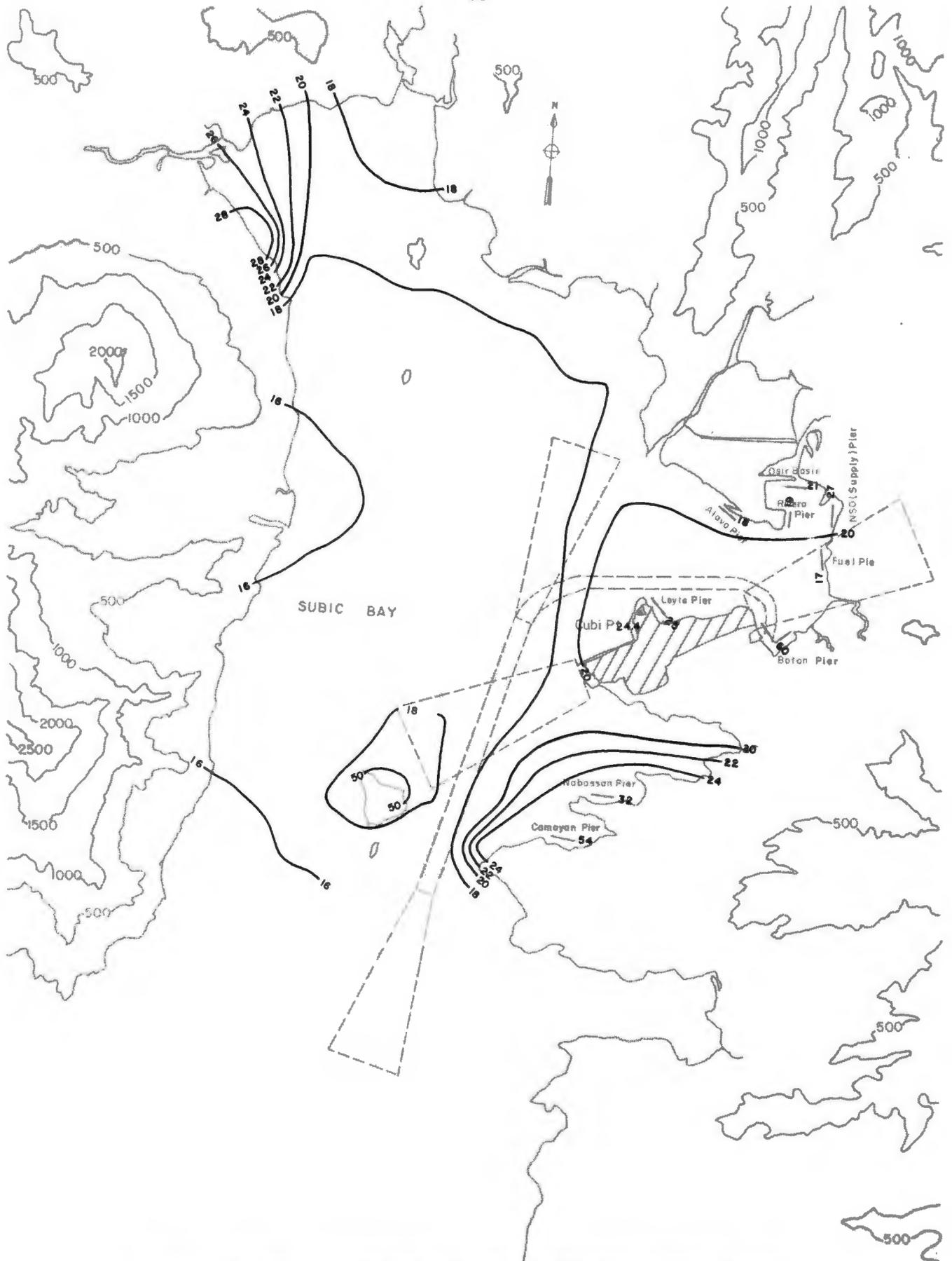
Fig. 15-2-b. Turbulence Intensity Contour Lines for the Subic Bay Basin at 180°T, z = 150 ft (45.7 m)
