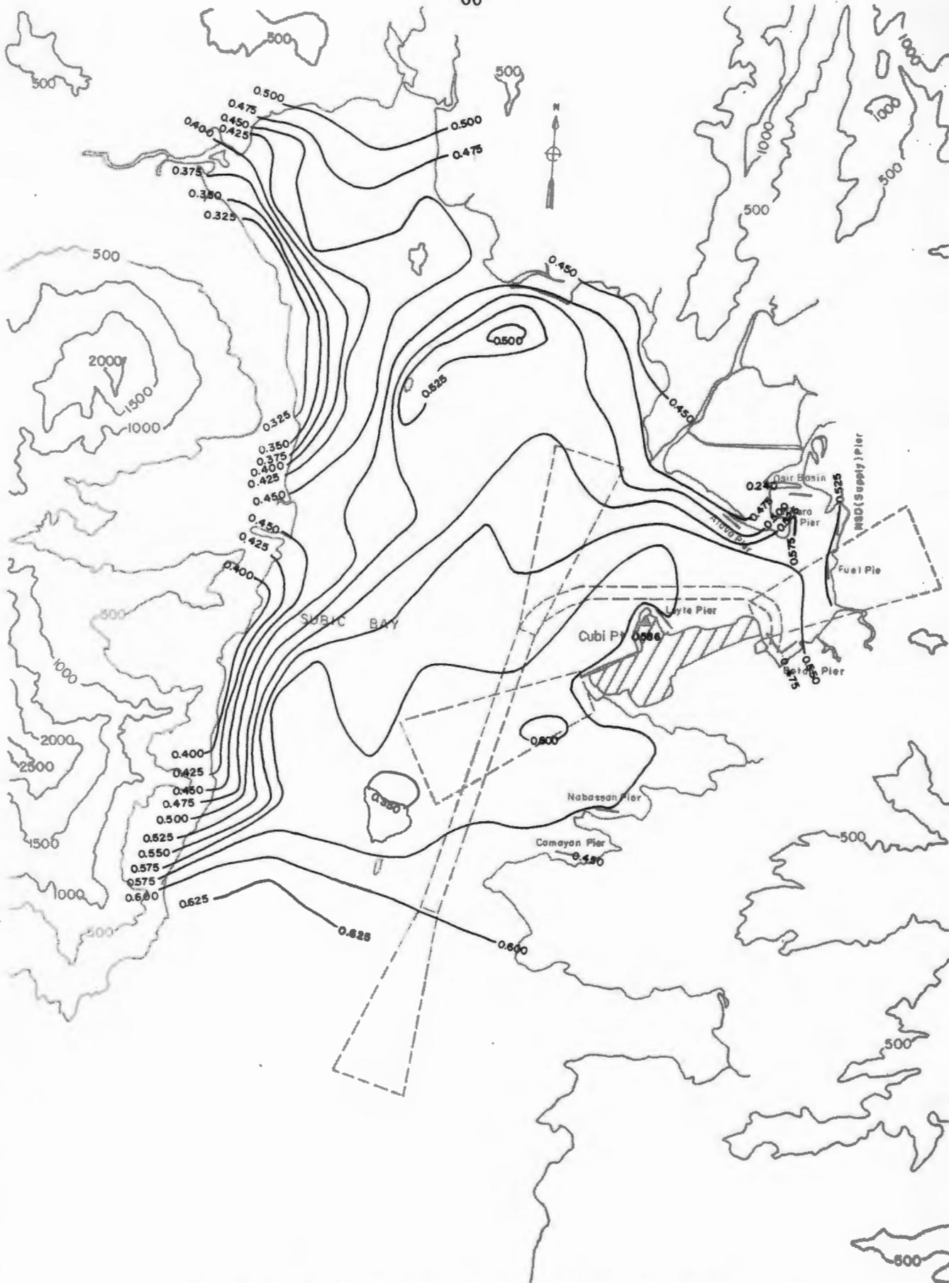
Fig. 18-3-a. Mean Wind Speed Isotachs for the Subic Bay Basin at 225°T, z = 195 ft (59.5 m)
