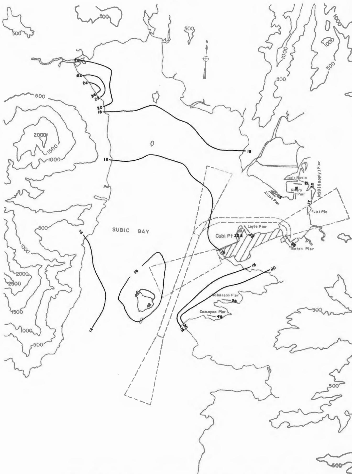
Fig. 16-3-b. Turbulence Intensity Contour Lines for the Subic Bay Basin at  $195^{\circ}\text{T}$ ,  $z = 195 \text{ ft}$  (59.5 m)
