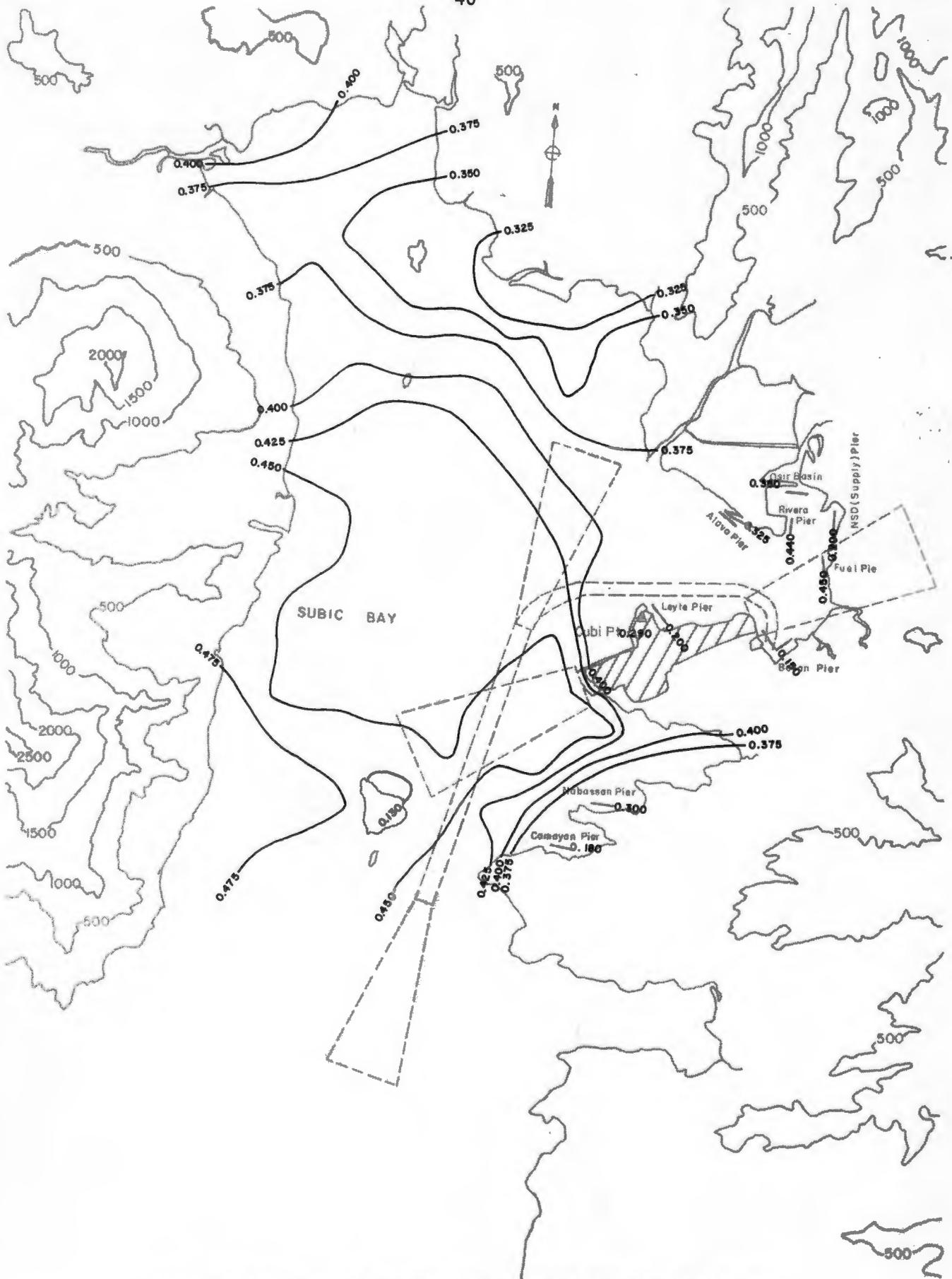
Fig. 16-1-a. Mean Wind Speed Isotachs for the Subic Bay Basin at 195°T, z = 70 ft (21.3 m)
