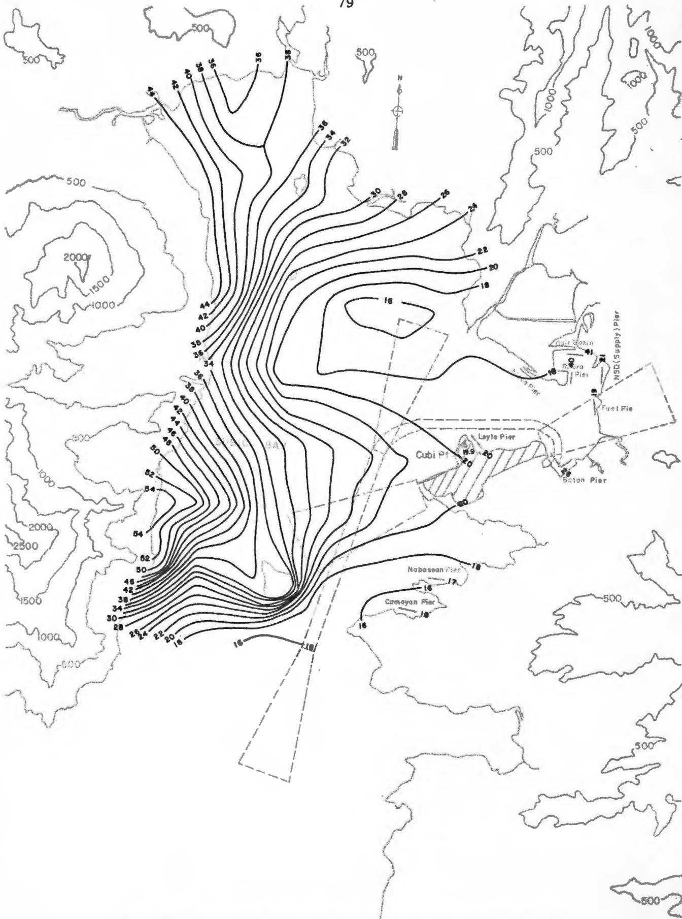
Fig. 20-4-b. Turbulence Intensity Contour Lines for the Subic Bay Basin at 255<sup>ft</sup>T, z = 275 ft (83.9 m)
