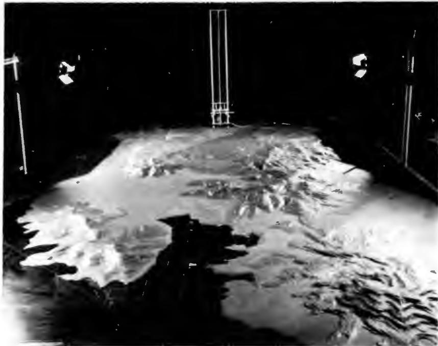
Fig. 2. Topographical Model in Wind Tunnel
