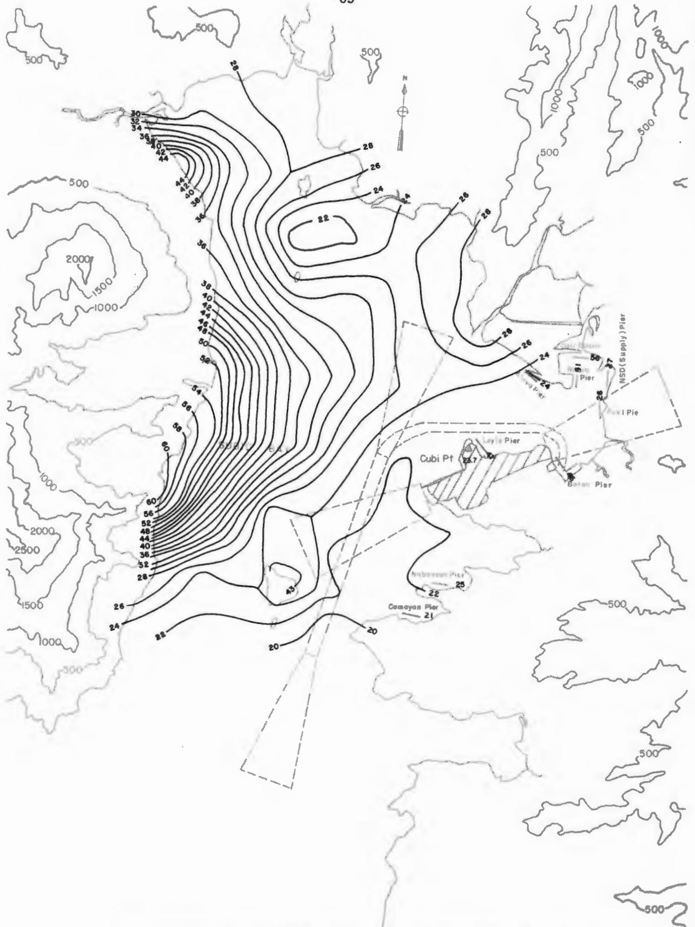
Fig. 19-1-b. Turbulence Intensity Contour Lines for the Subic Bay Basin at 240°T, z = 70 ft (21.3 m)
