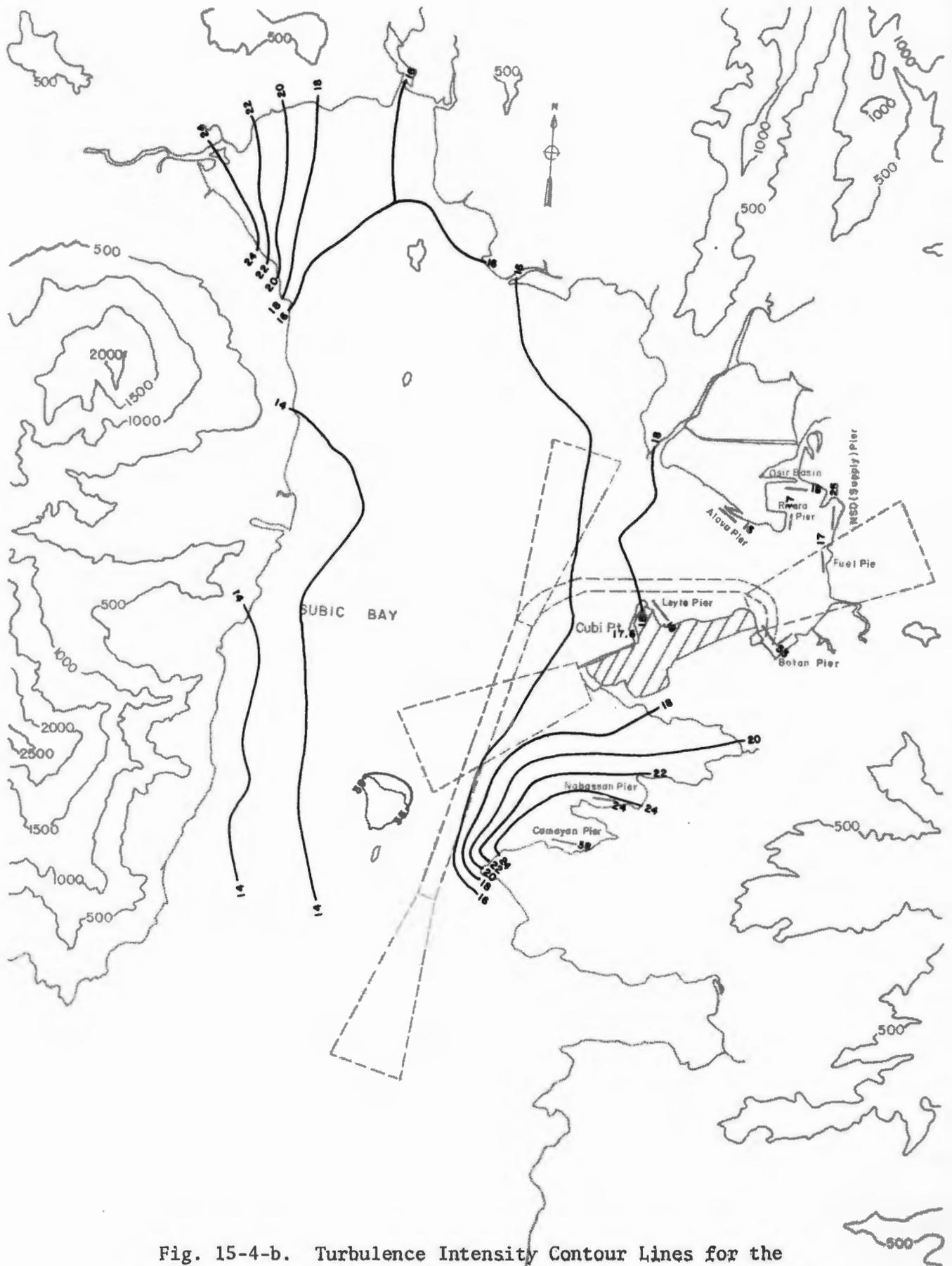
Fig. 15-4-b. Turbulence Intensity Contour Lines for the Subic Bay Basin at  $180^\circ T$ ,  $z = 275$  ft (83.9 m)
