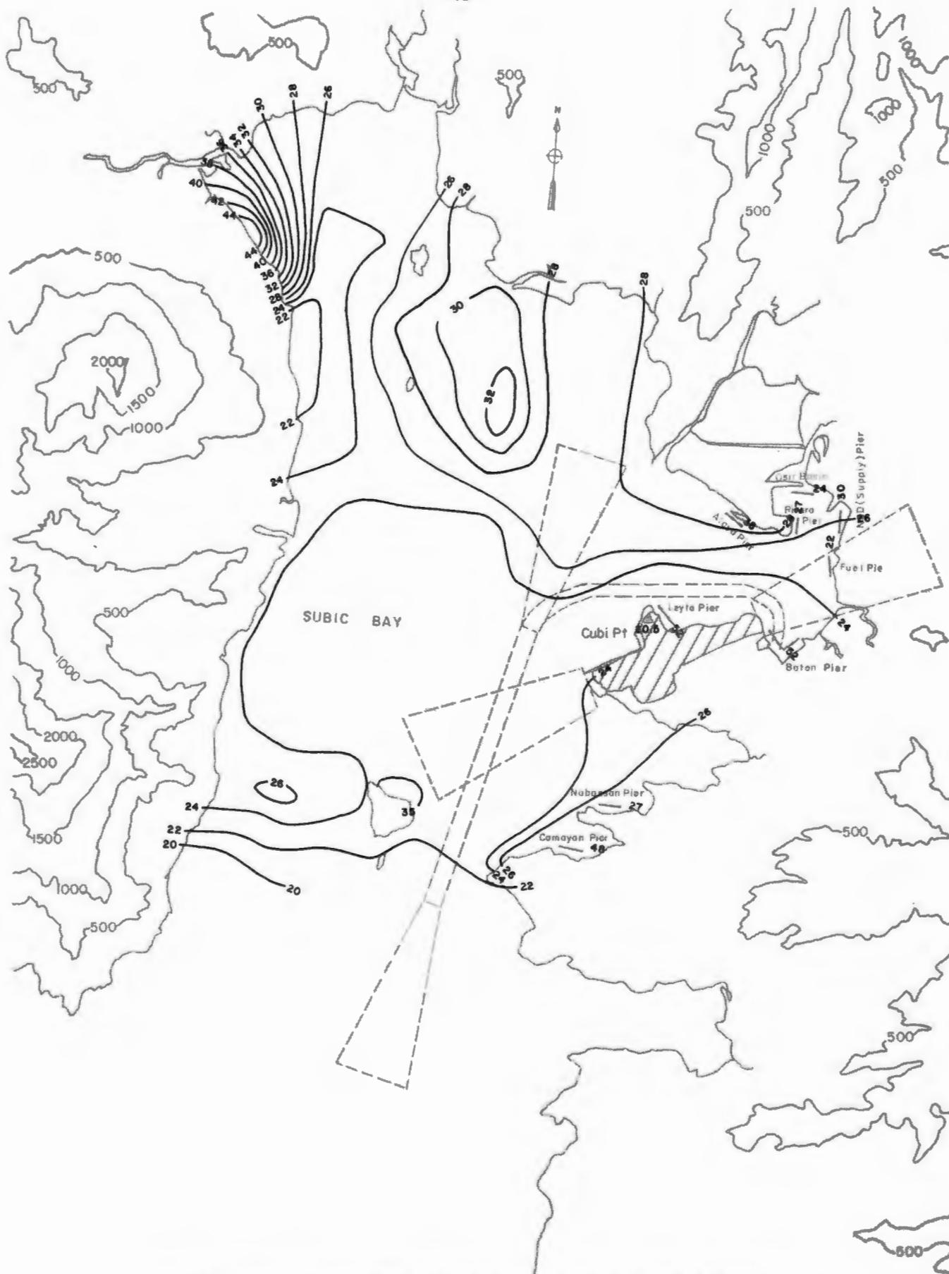
Fig. 17-1-b. Turbulence Intensity Contour Lines for the Subic Bay Basin at 210°T, z = 70 ft (21.3 m)
