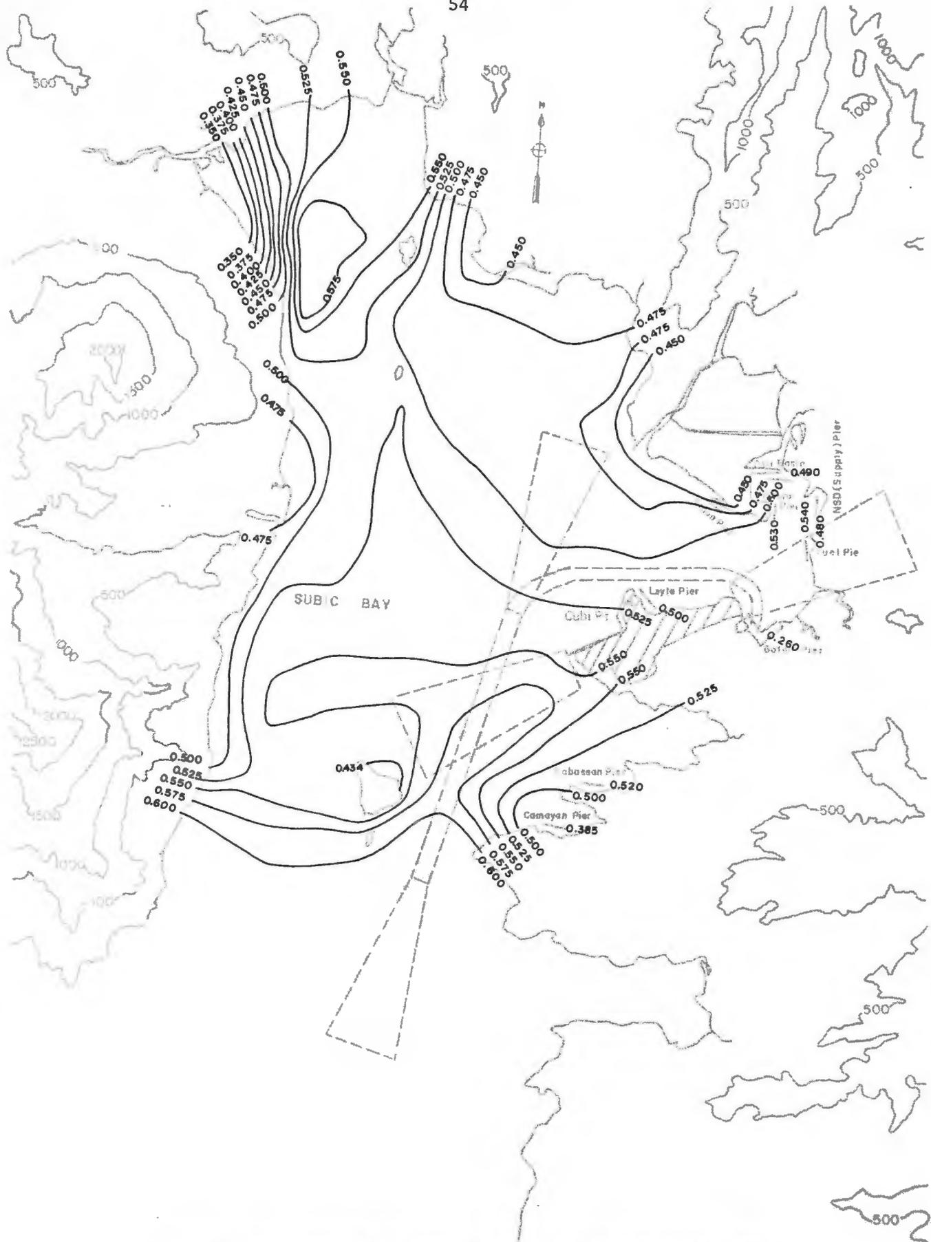
Fig. 17-4-a. Mean Wind Speed Isotachs for the Subic Bay Basin at 210°T, z = 275 ft (83.9 m)
