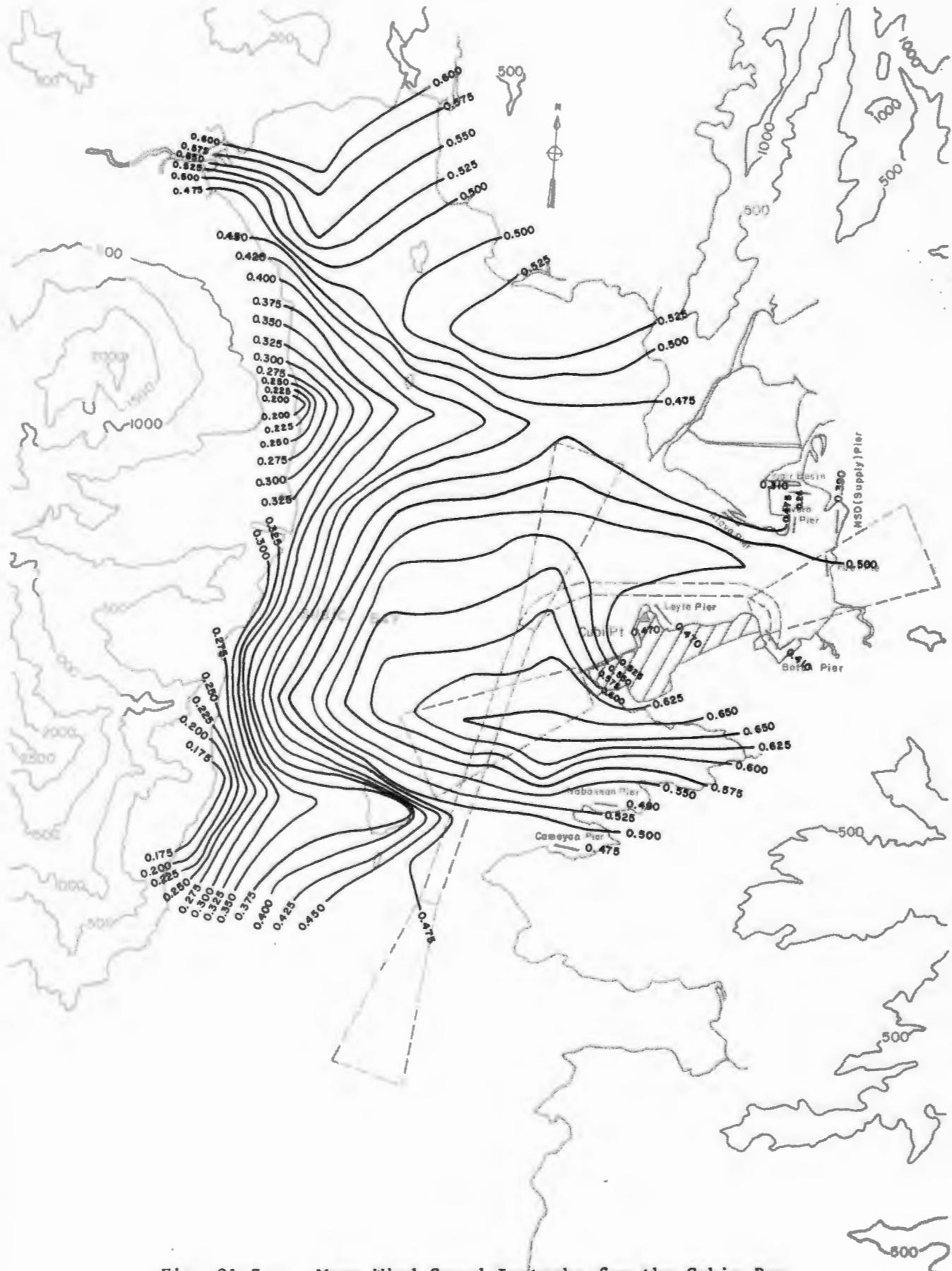
Fig. 21-3-a. Mean Wind Speed Isotachs for the Subic Bay Basin at 270°T, z = 195 ft (59.5 m)
