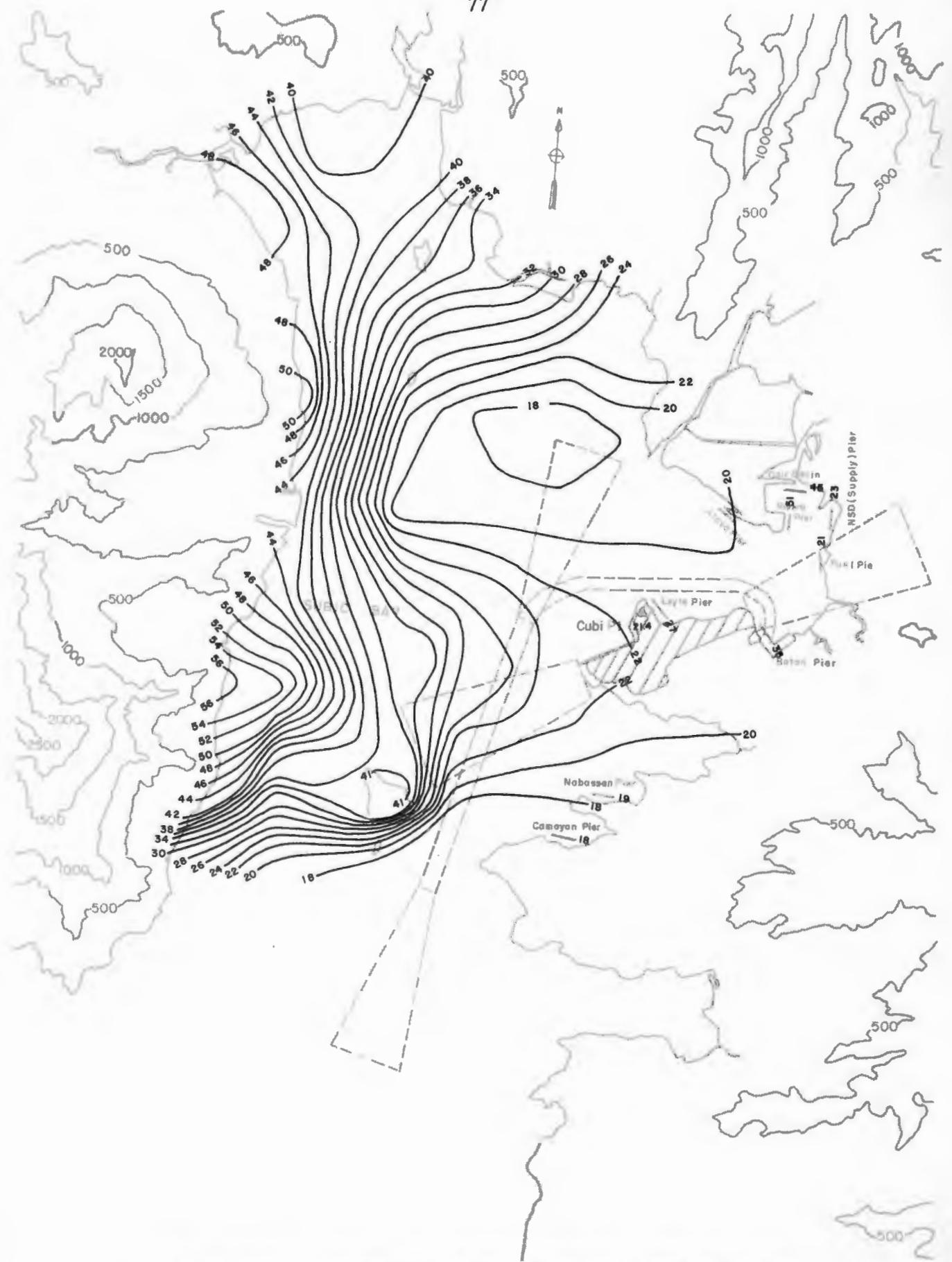
Fig. 20-3-b. Turbulence Intensity Contour Lines for the Subic Bay Basin at 255°T, z = 195 ft (59.5 m)
