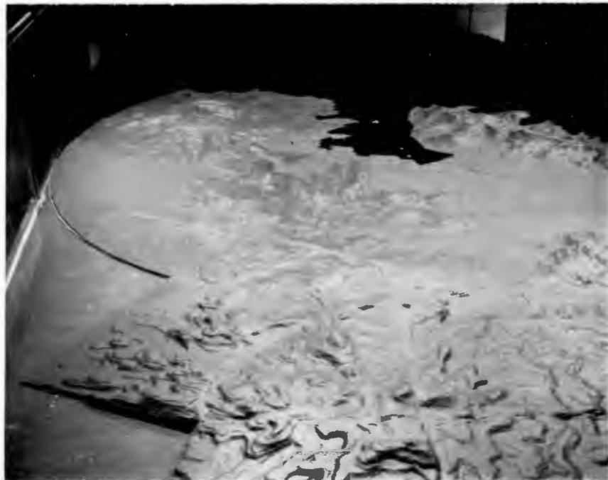
Fig. 3. Topographical Model in Wind Tunnel
