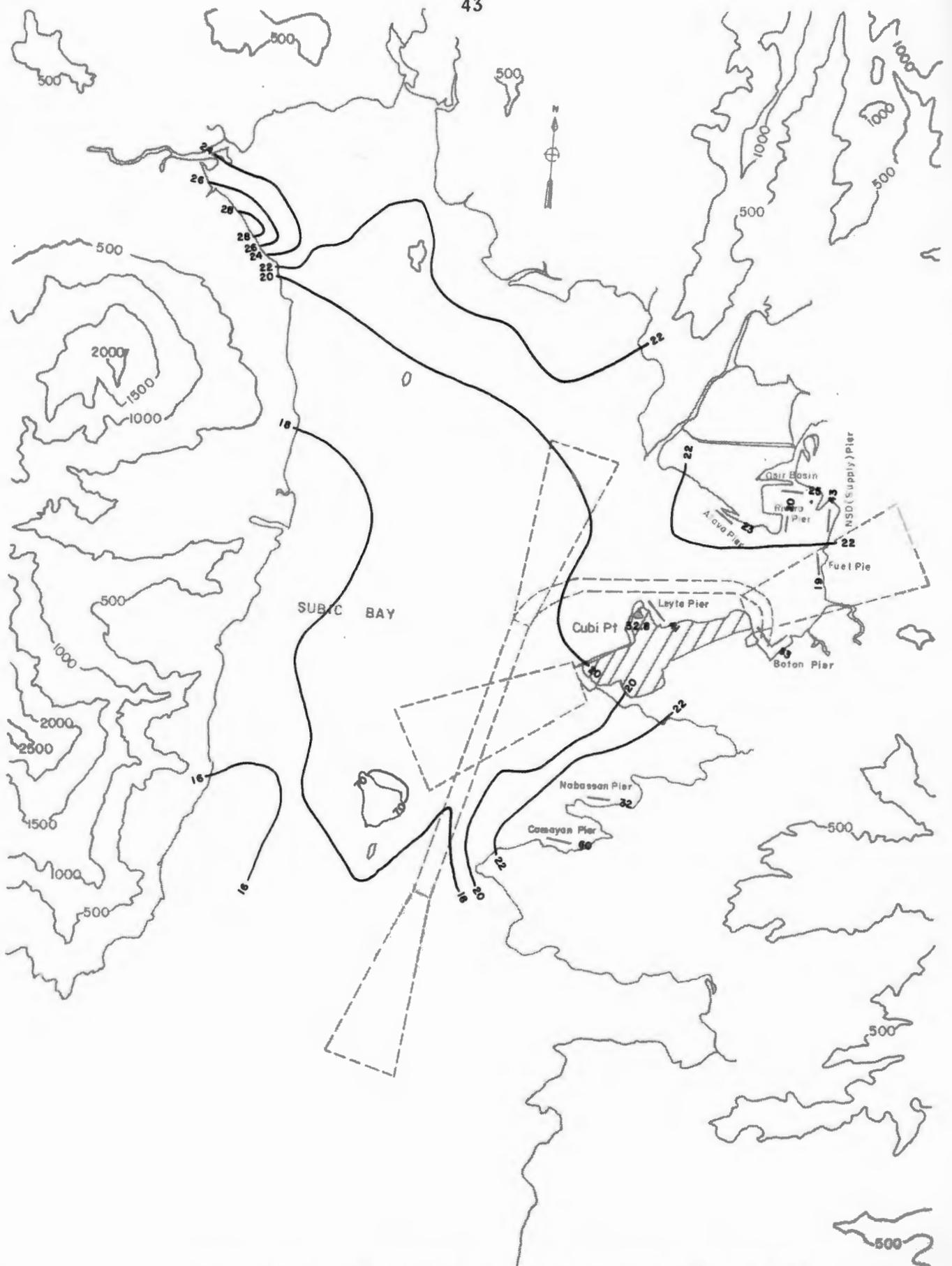
Fig. 16-2-b. Turbulence Intensity Contour Lines for the Subic Bay Basin at 195°T, z = 150 ft (45.7 m)
