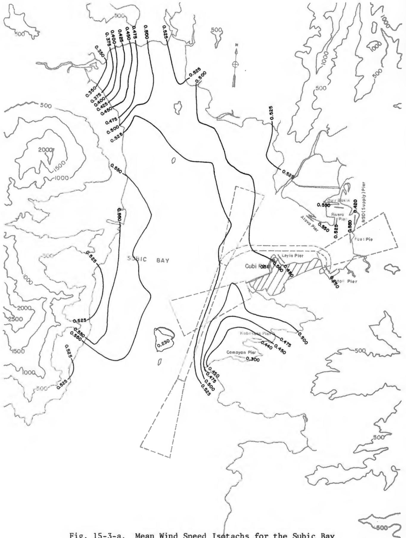
Fig. 15-3-a. Mean Wind Speed Isotachs for the Subic Bay Basin at 180°T, z = 195 ft (59.5 m)
