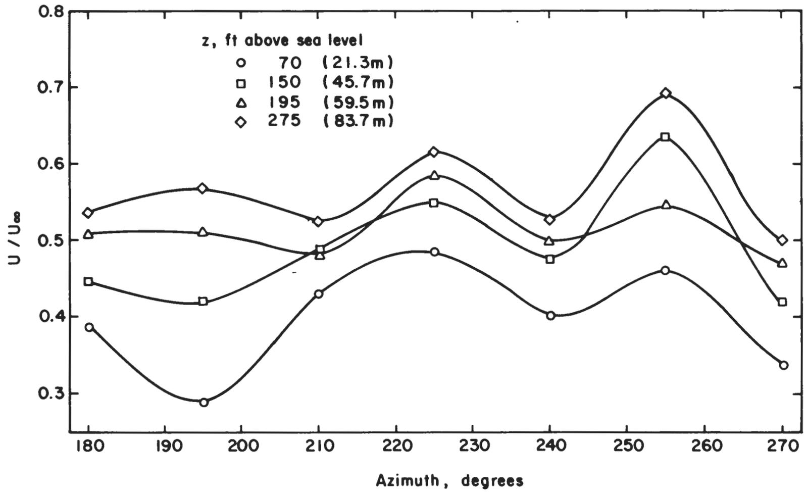
Fig. 23. Mean Velocity at Cubi Point Meteorological Station
