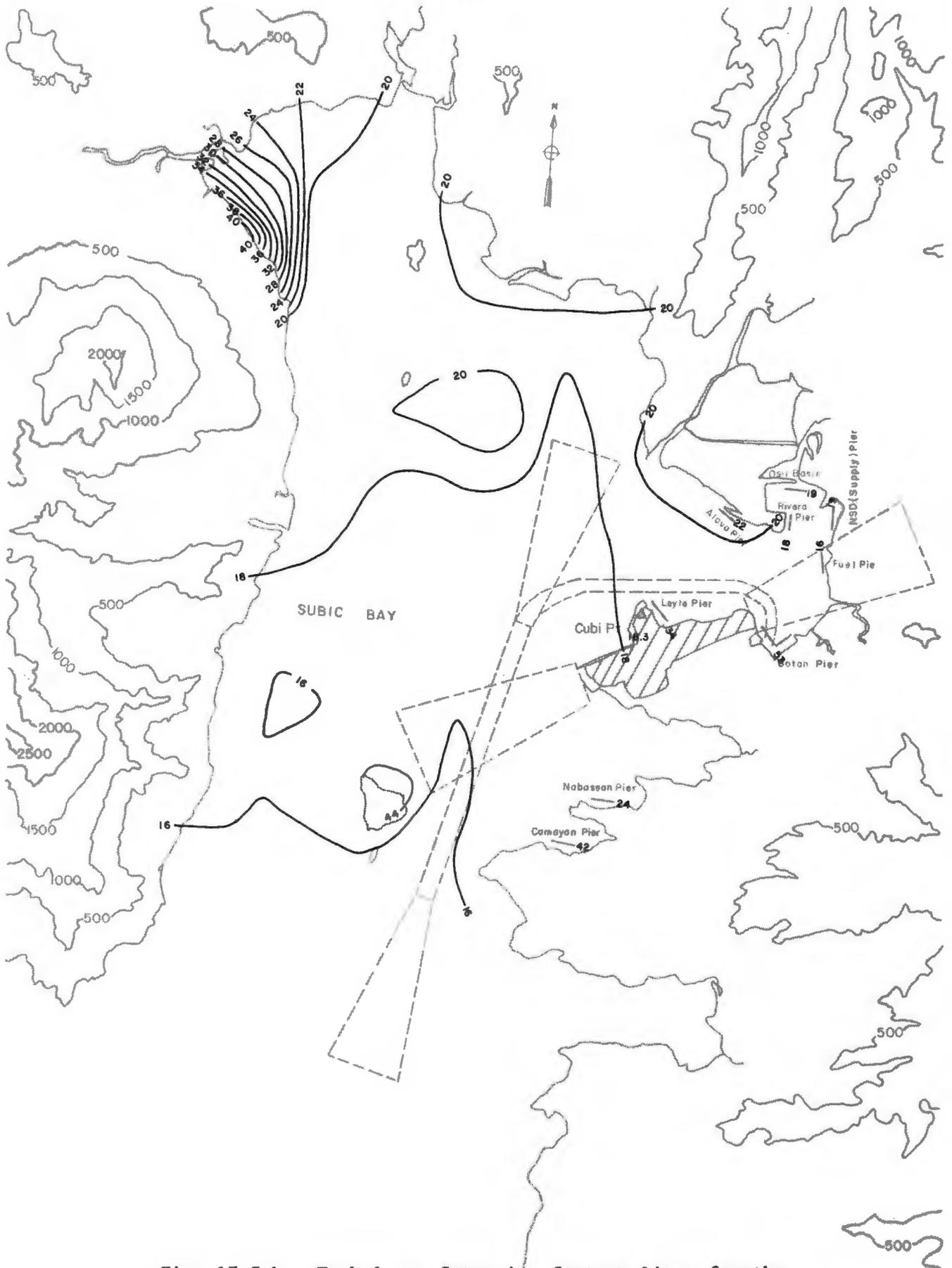
Fig. 17-3-b. Turbulence Intensity Contour Lines for the Subic Bay Basin at 210°T, z = 195 ft (59.5 m)
