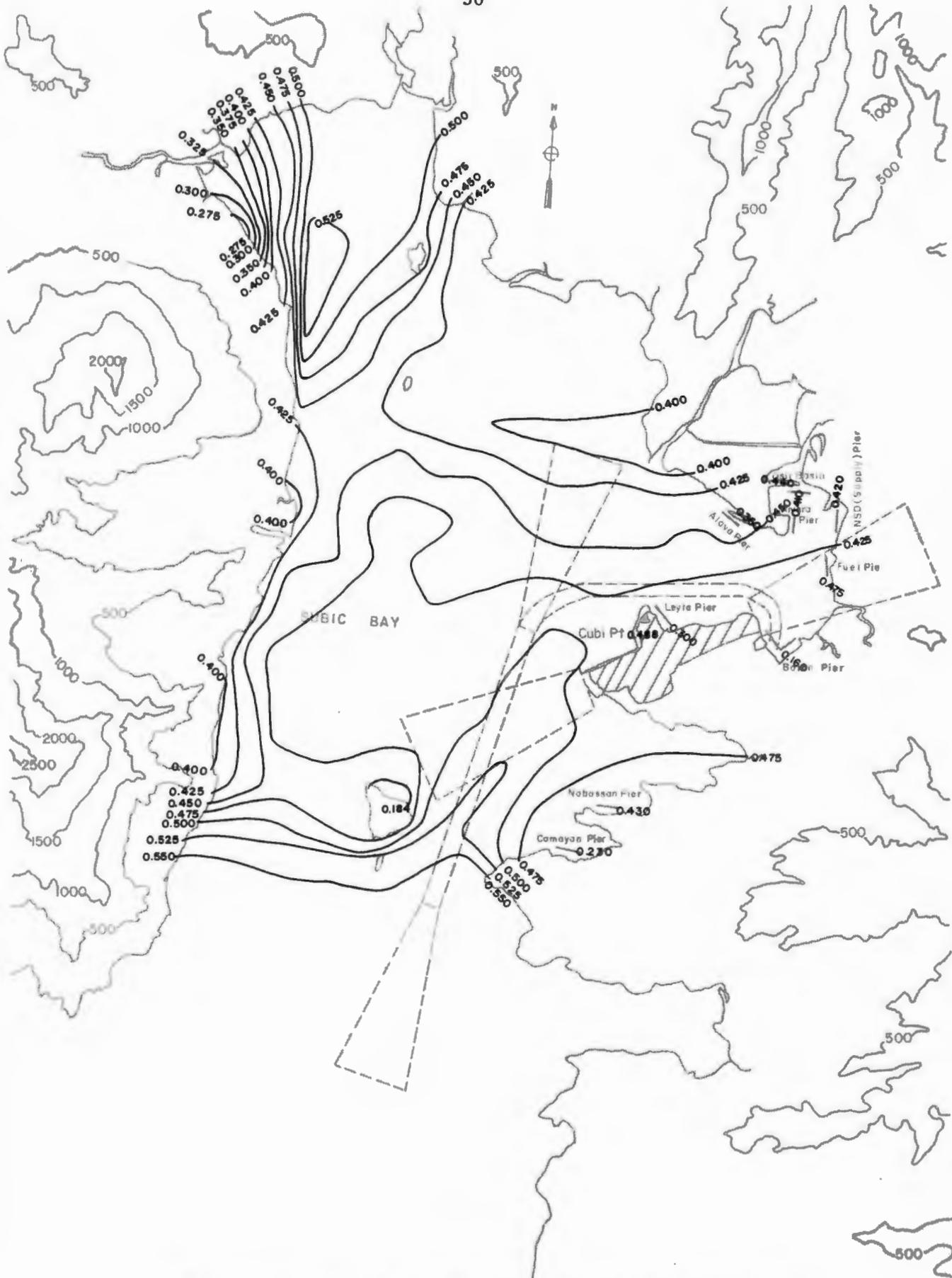
Fig. 17-2-a. Mean Wind Speed Isotachs for the Subic Bay Basin at 210°T, z = 150 ft (45.7 m)
