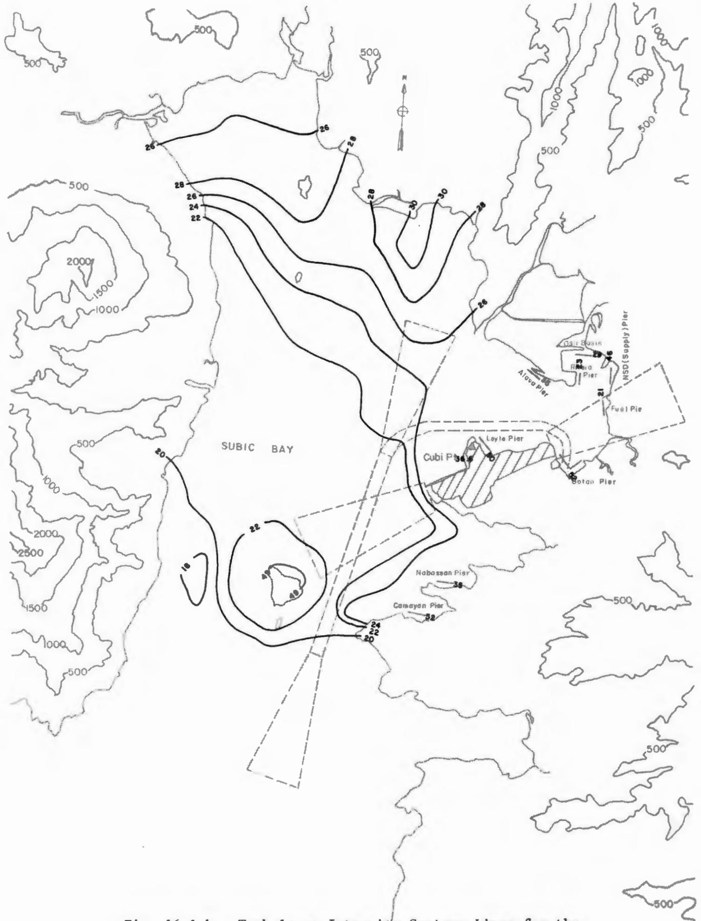
Fig. 16-1-b. Turbulence Intensity Contour Lines for the Subic Bay Basin at 1950°T, z = 70 ft (21.3 m)
