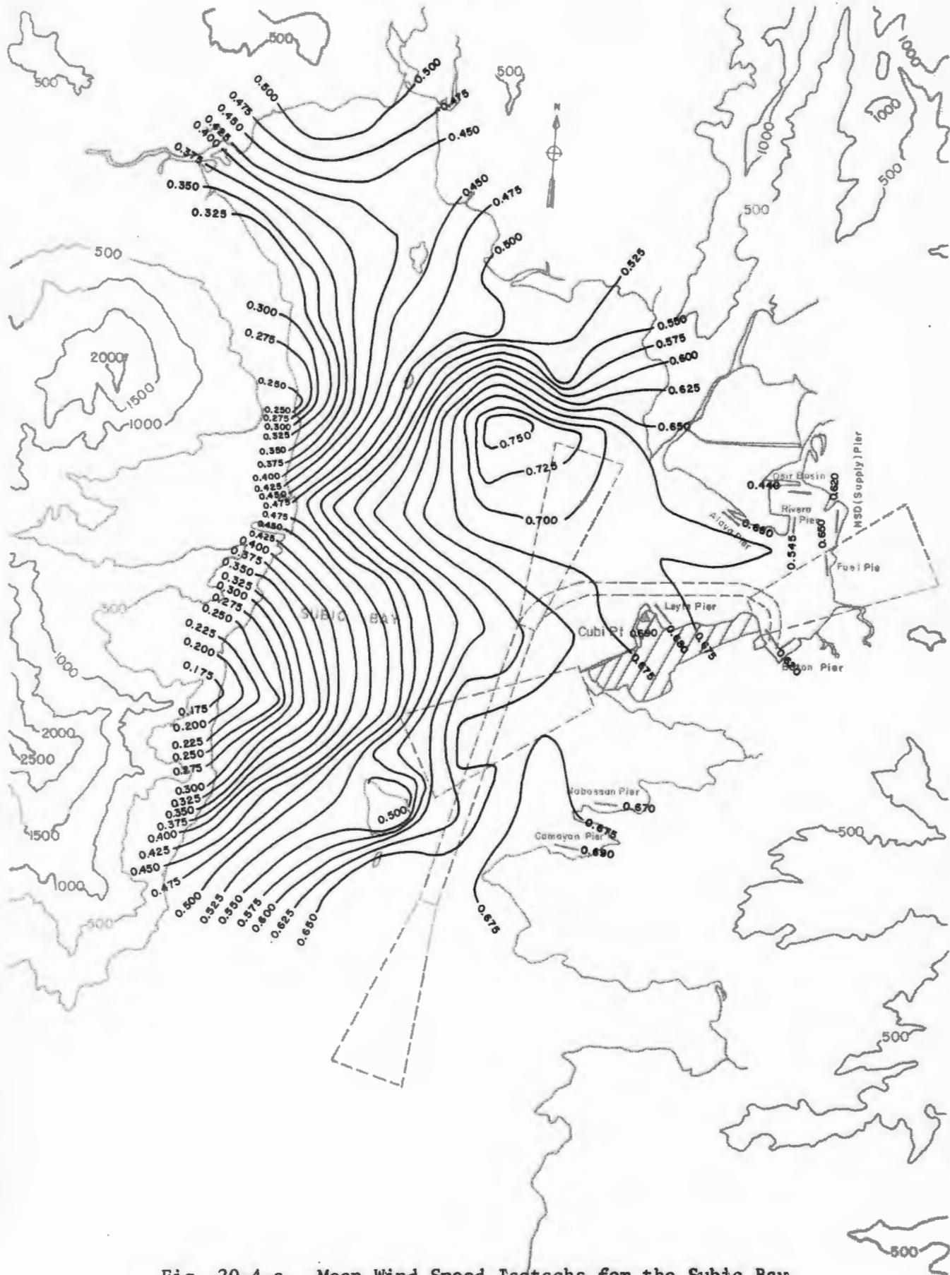
Fig. 20-4-a. Mean Wind Speed Isotachs for the Subic Bay Basin at 255°F, z = 275 ft (83.9 m)
