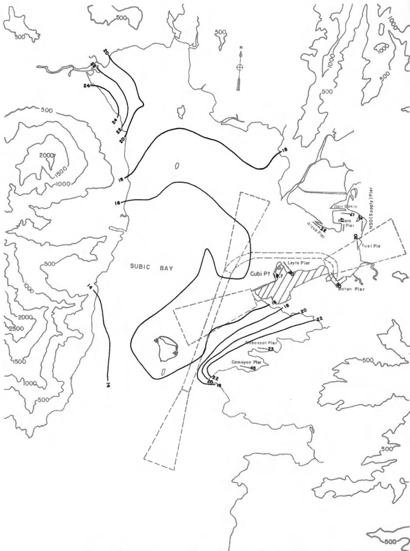
Fig. 16-4-b. Turbulence Intensity Contour Lines for the Subic Bay Basin at  $195^{\circ}\text{T}$ ,  $z = 275 \text{ ft}$  (83.9 m)
