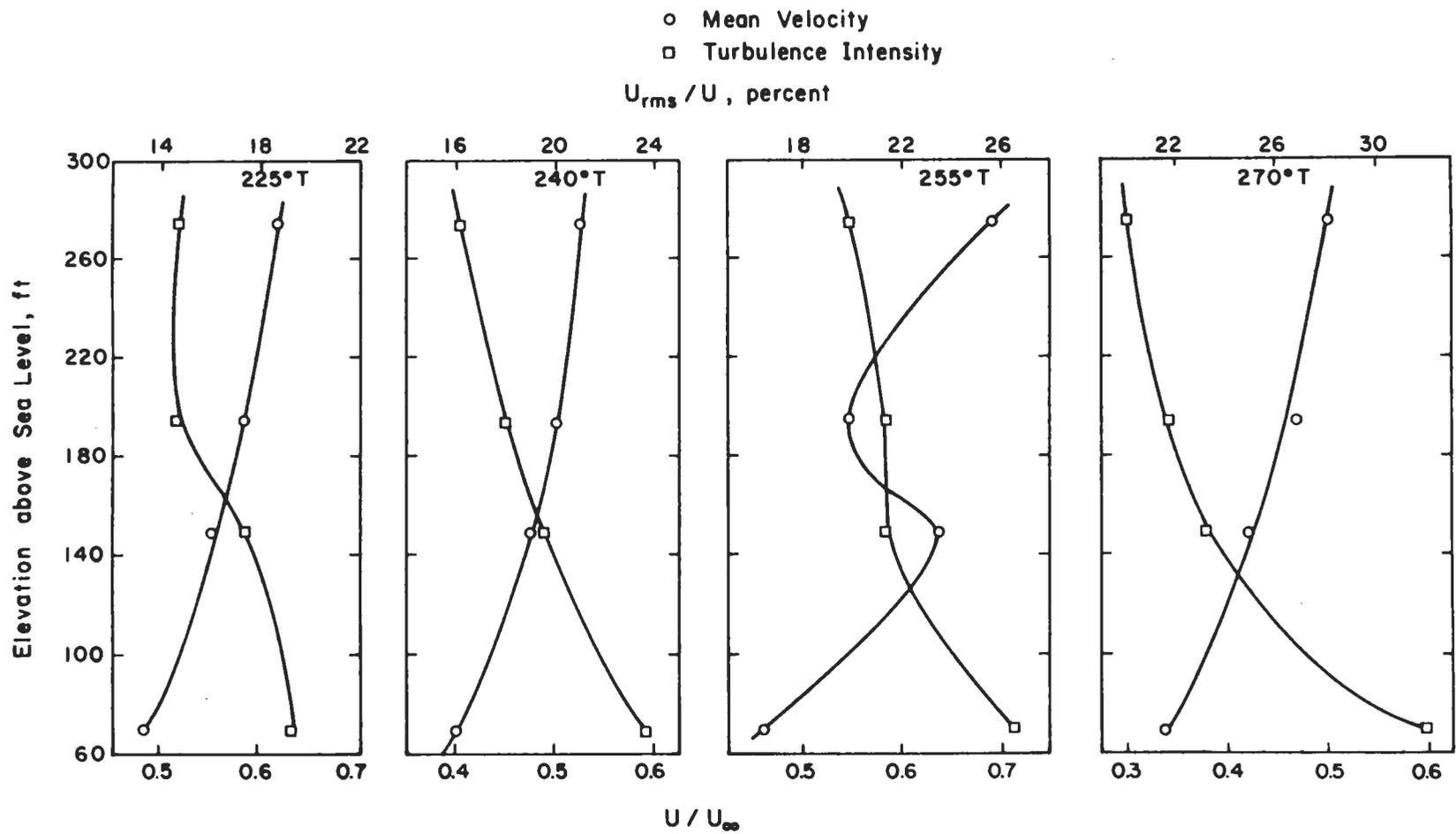
Fig. 22-b. Mean Velocity and Turbulence Profiles at Cubi Point Meteorological Station at 15 Degree Intervals
