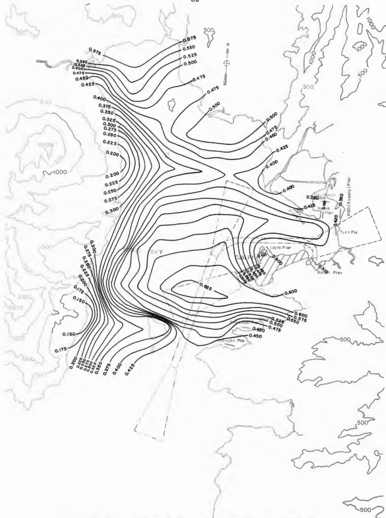
Fig. 21-2-a. Mean Wind Speed Isotachs for the Subic Bay Basin at 270°T, z = 150 ft (45.7 m)
