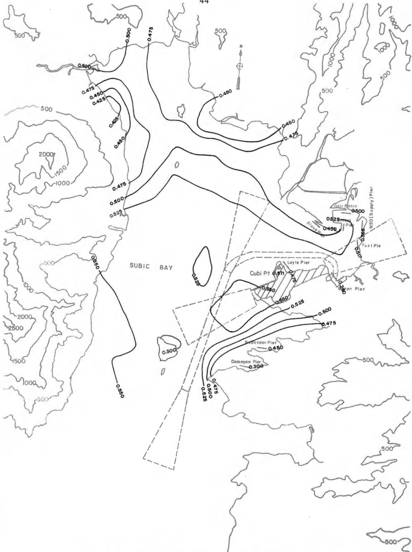
Fig. 16-3-a. Mean Wind Speed Isotachs for the Subic Bay Basin at 195°T, z = 195 ft (59.5 m)
