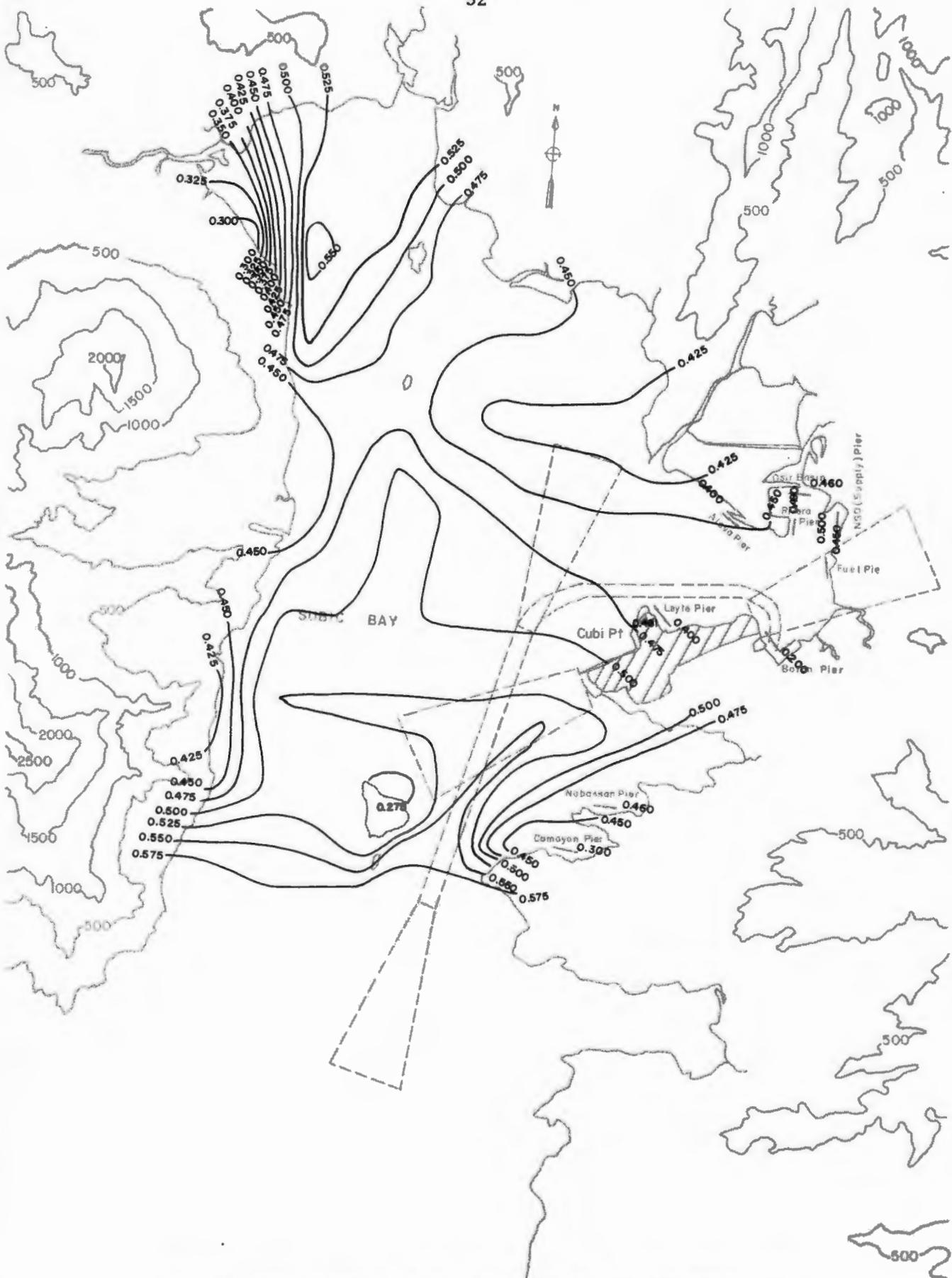
Fig. 17-3-a. Mean Wind Speed Isotachs for the Subic Bay Basin at  $210^\circ T$ ,  $z = 195$  ft (59.5 m)
