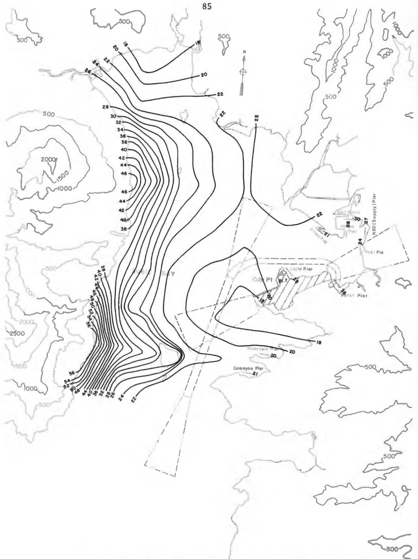
Fig. 21-3-b. Turbulence Intensity Contour Lines for the Subic Bay Basin at  $270^\circ T$ ,  $z = 195$  ft (59.5 m)
