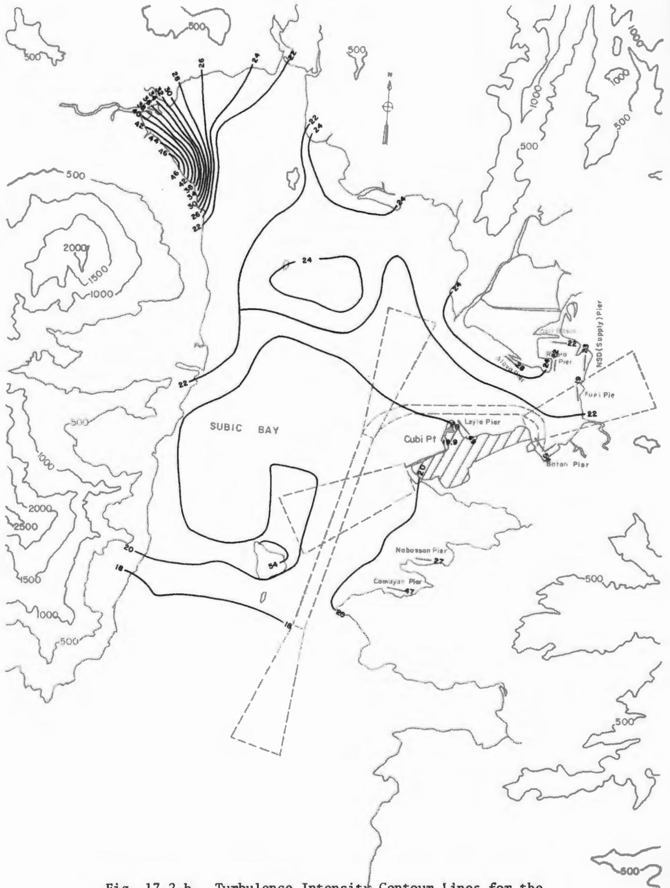
Fig. 17-2-b. Turbulence Intensity Contour Lines for the Subic Bay Basin at 210<sup>th</sup>T, z = 150 ft (45.7 m)
