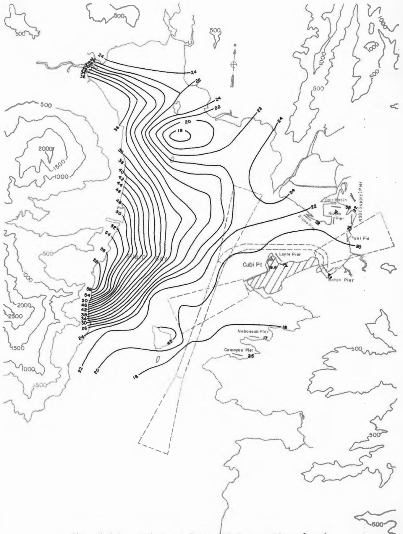
Fig. 19-2-b. Turbulence Intensity Contour Lines for the Subic Bay Basin at  $240^{\circ}T$ ,  $z = 150$  ft (45.7 m)
