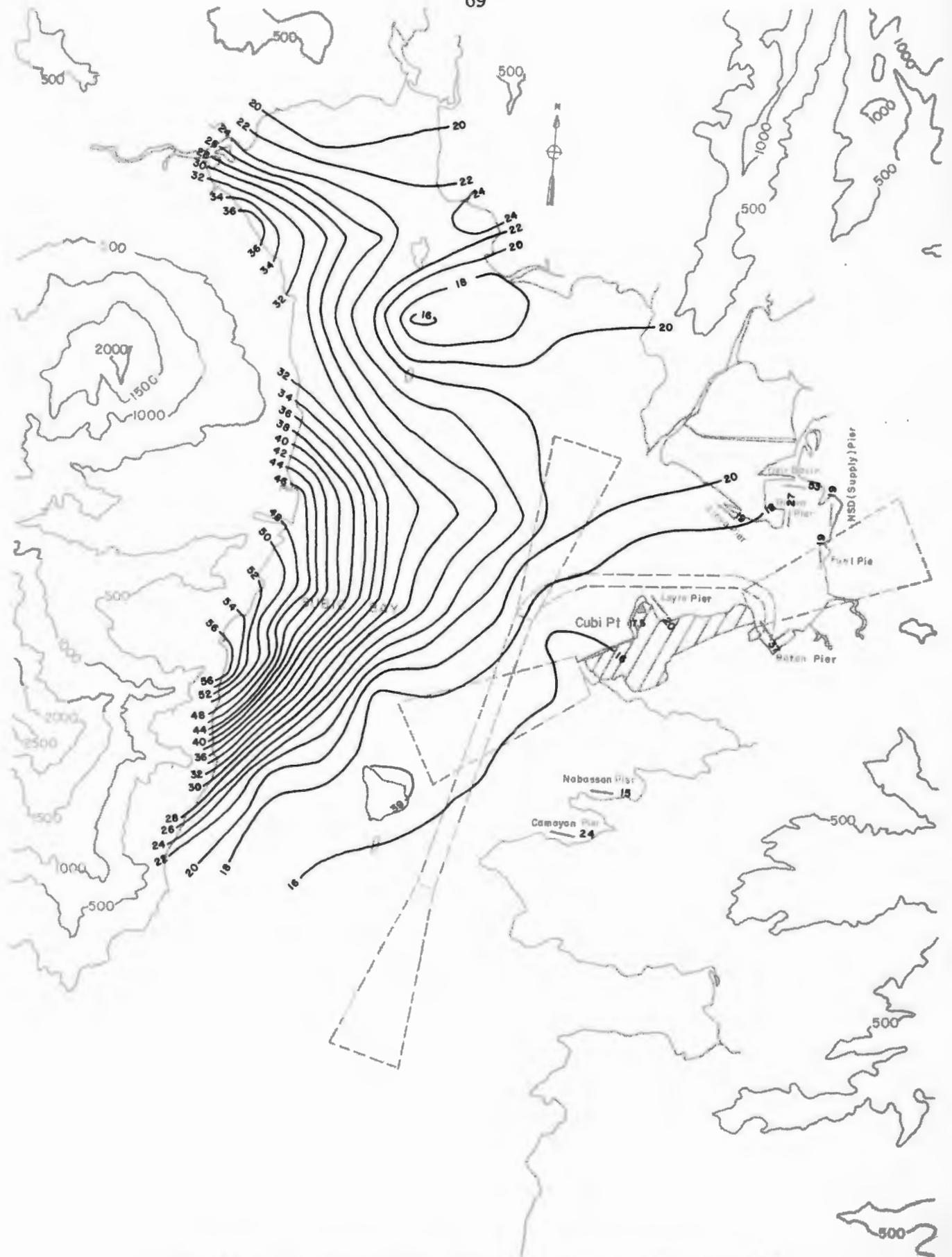
Fig. 19-3-b. Turbulence Intensity Contour Lines for the Subic Bay Basin at 240°T, z = 195 ft (59.5 m)
