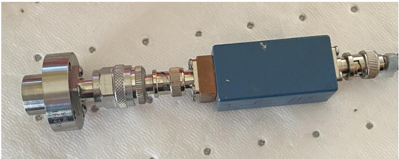
Figure 5: D-dot probe with RC integrator.
