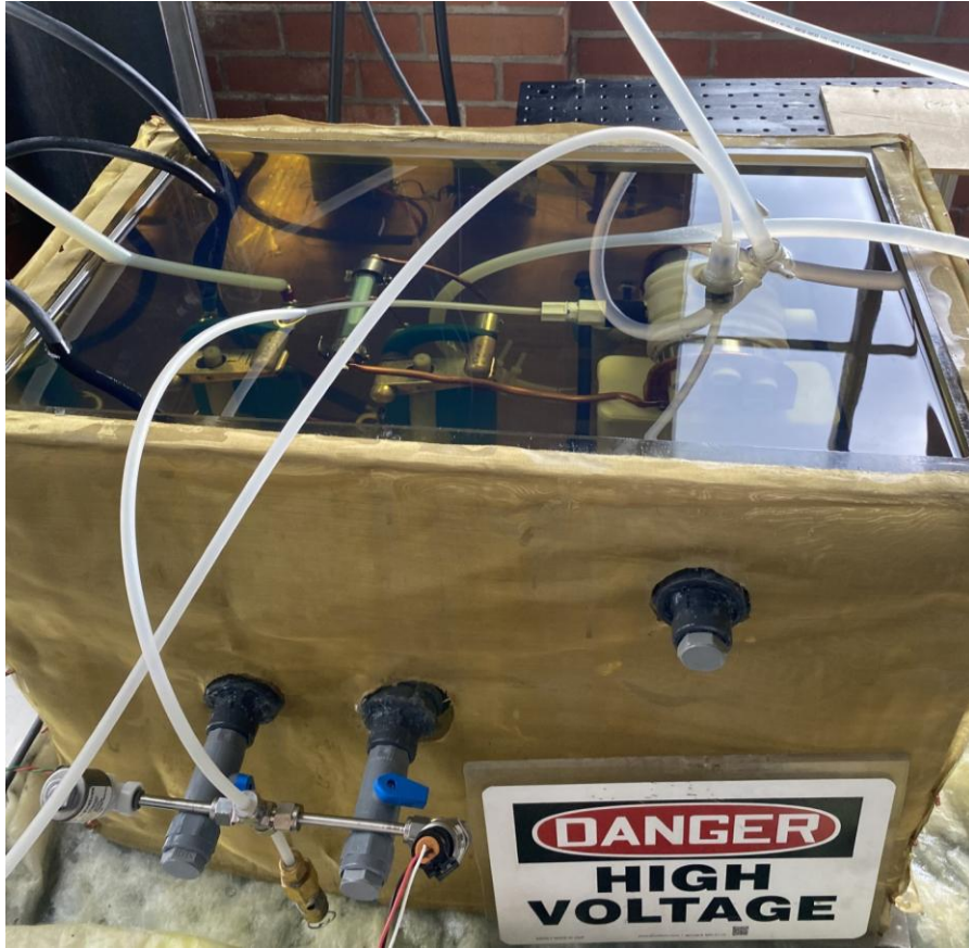
Figure 11: High voltage switch experiment with Faraday cages.
