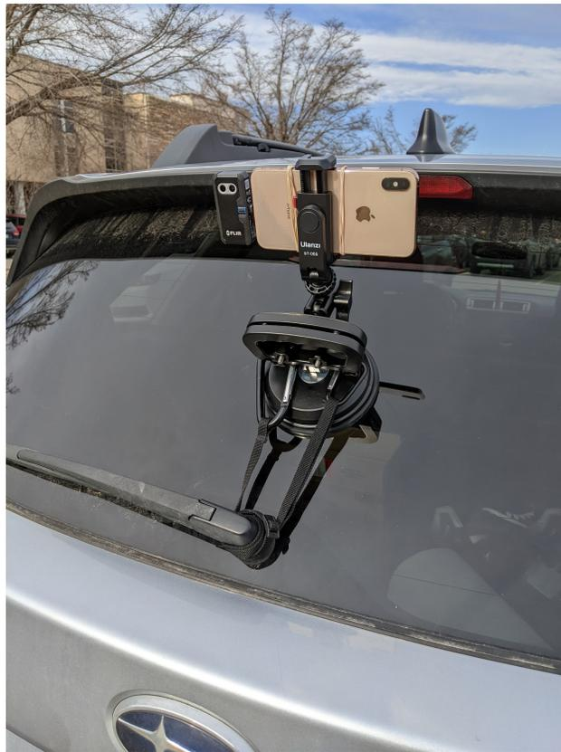
**Figure 4.2:** FLIR thermal camera setup.
