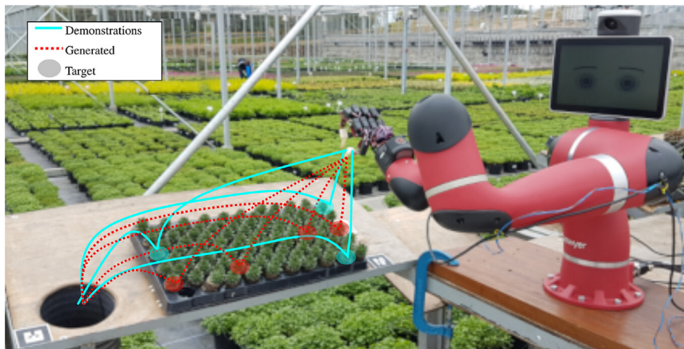
Figure 2.8: Learning from human demonstrations on how to discard unhealthy potted plants. The targets are labeled with shaded circles, and the human demonstrations (in cyan) are provided to the agent for learning. After training, the robot’s attempts at the task are shown in red.
