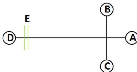
**Figure 1.5:** The basic design for buffer reservoirs and channels in a microchip is shown. (A) is the sample reservoir, (B) is the buffer reservoir, (C) is the buffer waste reservoir, (D) is the sample waste reservoir and (E) is the detection electrodes.
