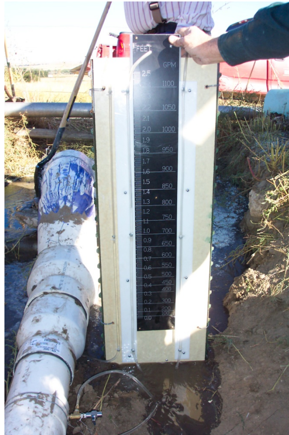
Figure 4. PID demonstration pipe-fitting Venturi and manometer
