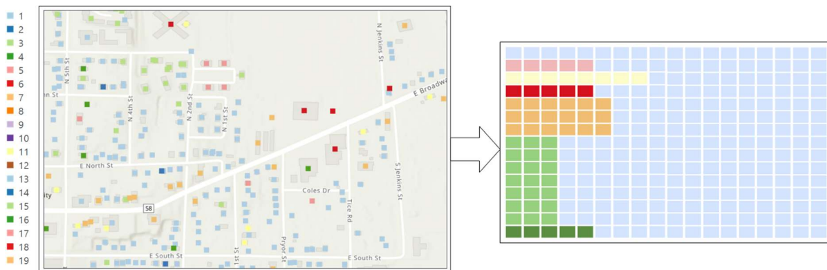
Figure 41: Schematic visualization of the conversion of building data from the x-y continuous map space (left) to discrete bin space (right) for a section of Mayfield. The legend here shows the archetypes of these structures (Memari et al., 2018)
