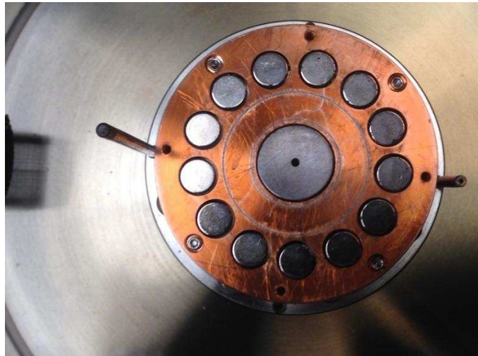
Figure 2.4. Top view of a modern magnetron sputtering gun. The bar magnets surrounded have identical S poles pointing up and the center magnet has an opposite pole direction. Sometimes the center magnet is replaced with a Cu rod for non-magnetic materials, as shown in the figure.
