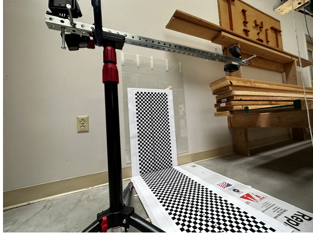
Figure 3.32: 3D calibration target set-up for dual stereo pairs calibration with the camera rig suspended above the target
