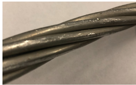
Figure 3.8: The ACSR cable used in the experiment
