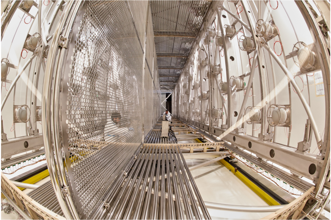
Figure 2.1: A fisheye view inside one of the ICARUS T300 during upgrades at CERN. The two TPCs are separated by a perforated cathode shown on the left side of the image, with the PMTs and wire-planes located on the right hand side and the field cage on the top and bottom of the TPC. Figure courtesy of CERN.
