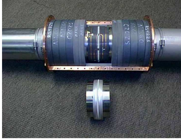
Figure 6.5: The Resistive Wall Monitor (RWM) showing the circuit board and ferrite used to extract the timing structure of the protons immediately before they hit the target. Picture from [21].
