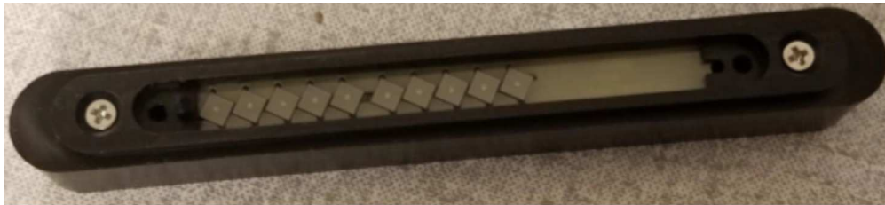
(b) SiPM based Optical Readout Modules used for the Side CRTs. Photo from [62].
