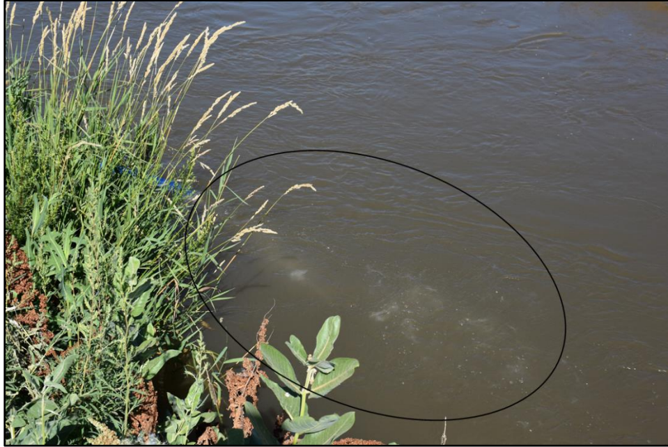
Figure B4-8: Viscous Xanthan Gum solution being poured into the canal via pump.
