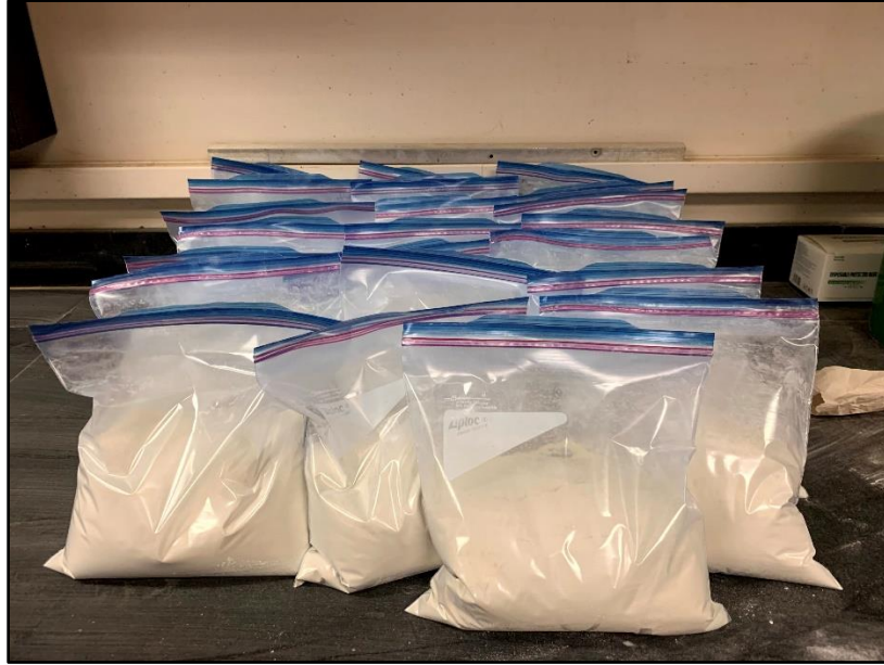
Figure B2-6: Pre-weighed Xanthan Gum in ziplock bags, ready for field application
