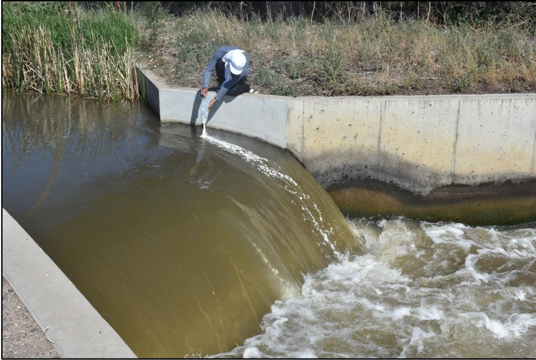
Figure B3-1: Dry XG applied at a flow-regulating structure (a tilting weir) during the 2022 XG application, approximately 300 meters upstream from the test reach on the LWC
