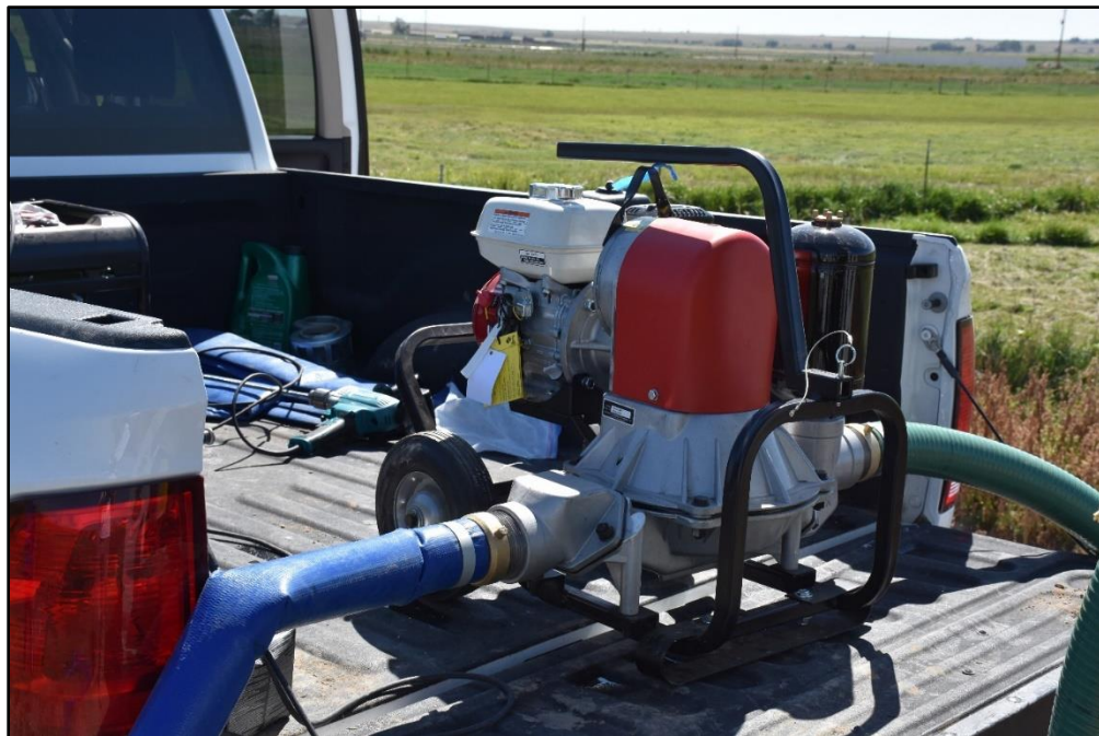
Figure B4-3: Honda WDP30XK1AT pump used to pump the viscous Xanthan Gum solution from the tank to the canal.
