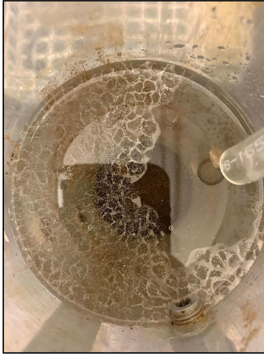
Figure B2-4: Top view of a column after pre-weighed Xanthan Gum (XG) was added, showing a slimy texture on the water surface.
