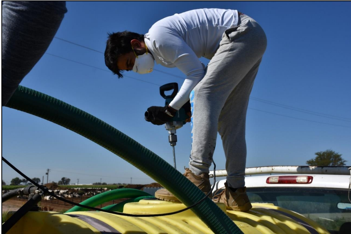
Figure B4-6: Technician using a Makita 8.5 Amp Corded Spade Handle Drill to mix and prepare the viscous Xanthan Gum solution.
