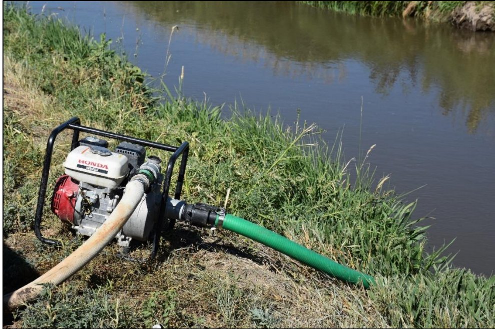
Figure B4-4 Centrifugal pump drawing water from the canal to the tank for Xanthan Gum preparation.
