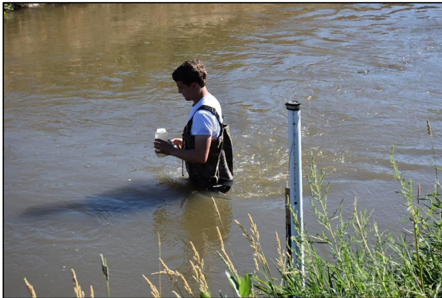
Figure B1-4: Technician collecting canal water samples near the upstream section of LWC reach for TSS analysis, replicated in laboratory experiments.
