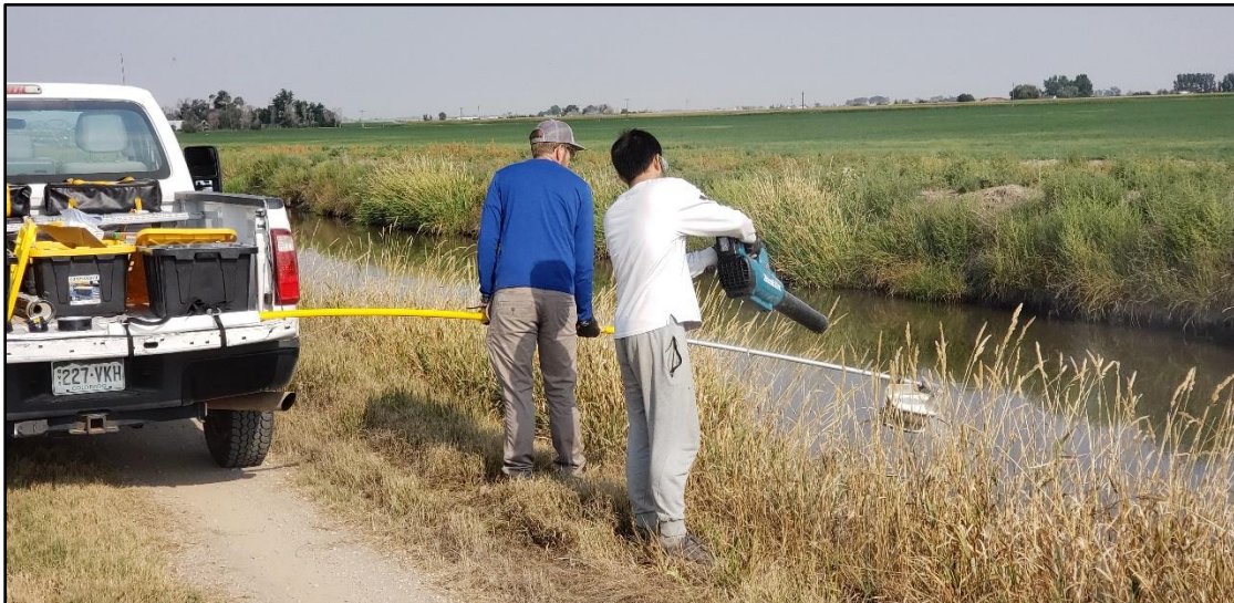
Figure B3-2: Dry XG application tool designed for use from the canal bank in 2021. An automated fertilizer spreader, loaded with XG, was mounted on a rod that was securely fixed to the bed of a truck carrying the supplies, including the XG.
