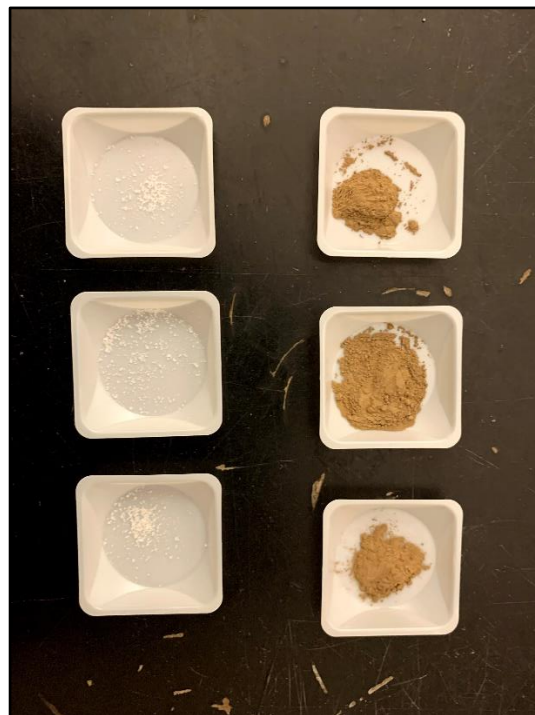
Figure B2-3: Pre-weighed TSS and polymer prepared in the laboratory for column experiments.
