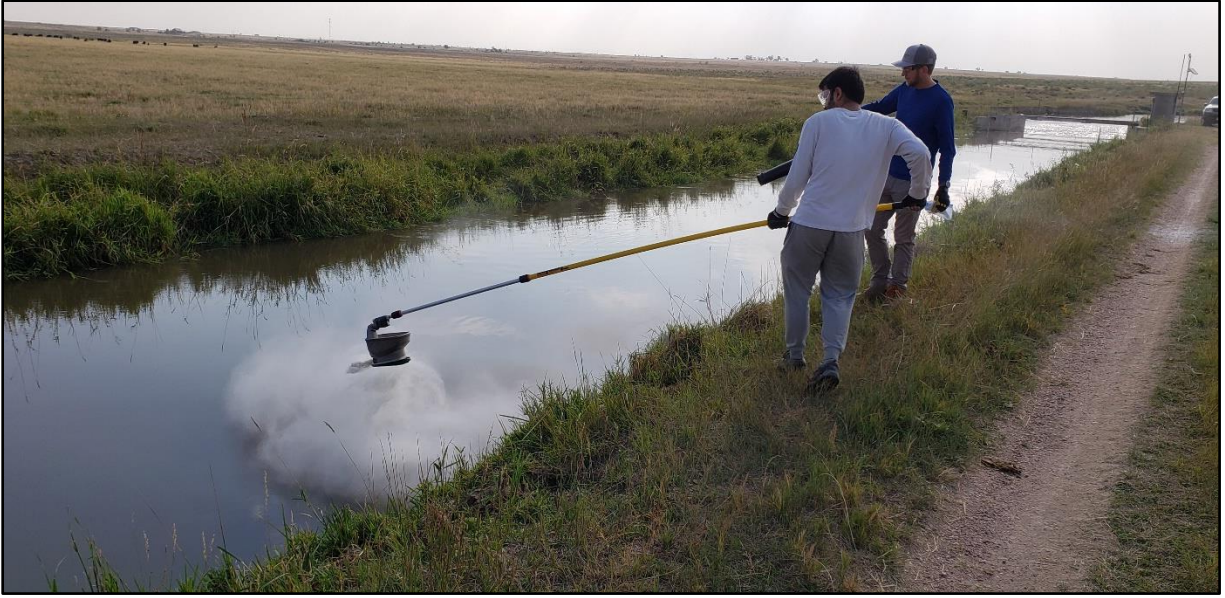
Figure B3-3: Another trial of dry XG application tool designed for use from the canal bank in 2021. One technician operated an automated fertilizer spreader, loaded with XG, while the other used a leaf blower to direct the XG onto the canal water surface.
