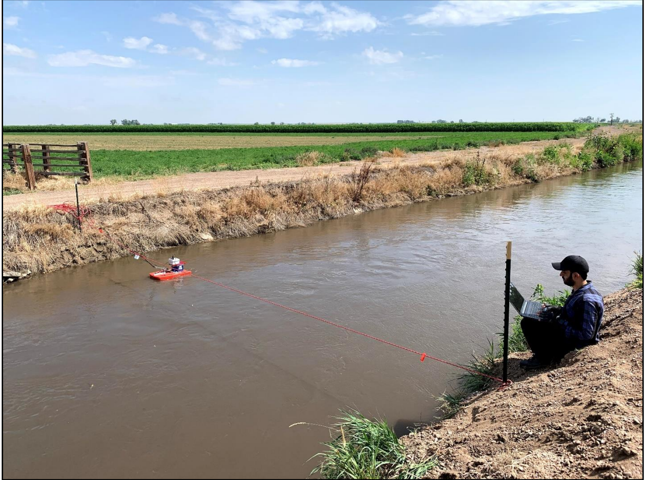
Figure B1-1: ADCP flow measurement in progress at the upstream section of the Larimer and Weld Canal (LWC) in 2021.
