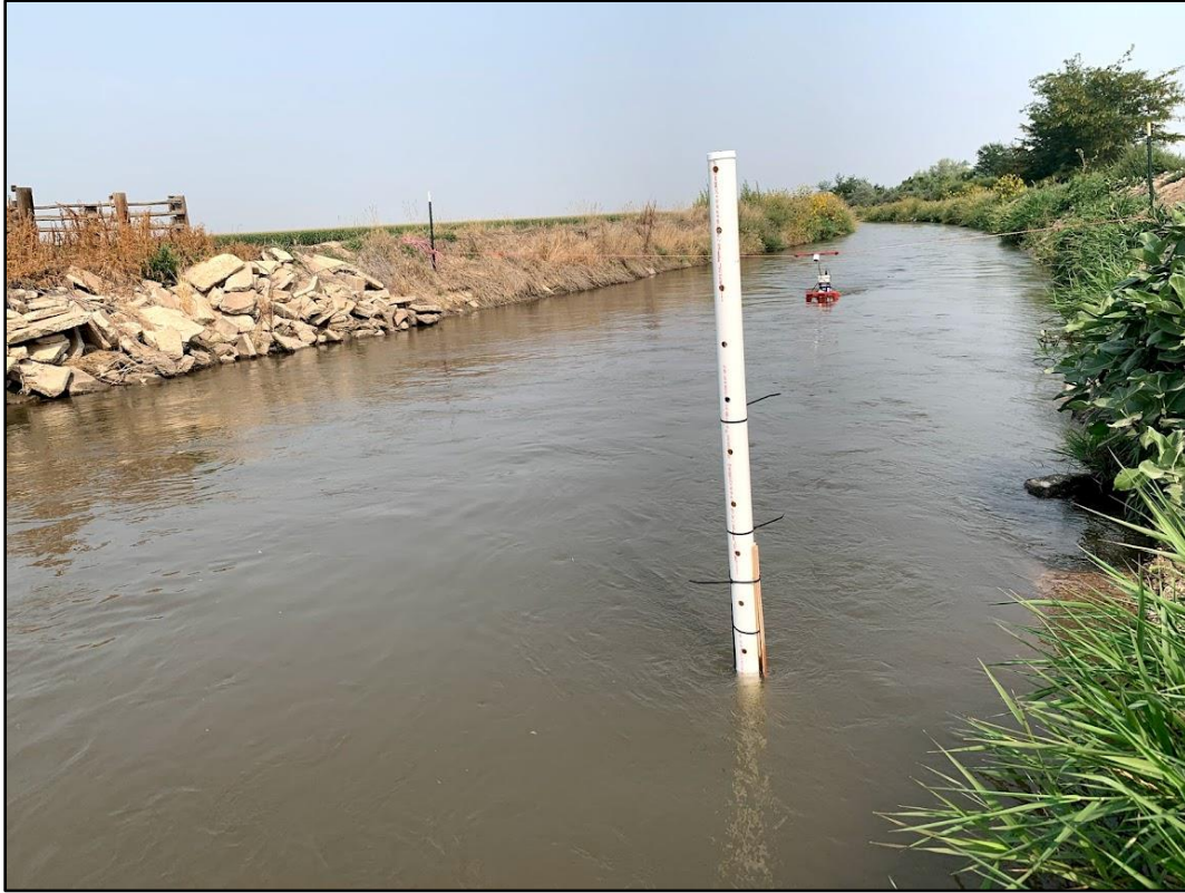
Figure B1-3: Perforated PVC pipe installed to hold the HOBO water level logger, used for recording water level fluctuations for storage change calculations.
