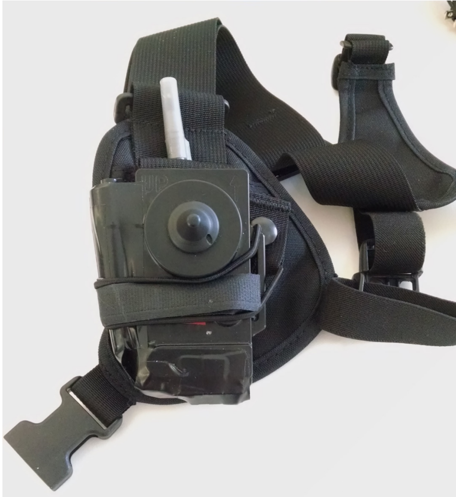
Figure C2: Modified UPAS. An Ultrasonic Personal Aerosol Sampler (UPAS) was modified to include a pushbutton (mounted on the side) and global positioning system (GPS; mounted on the bottom). Volunteers used the three-point harness to wear the UPAS for multiple days to collect the GPS, environmental (temperature, pressure, relative humidity, UV light), and motion data..
