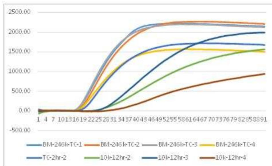
**Figure 1A.6:** WARP QT-NASBA from blood with 246,000 *P. falciparum* gametocytes/mL (BM-246k-TC-1 to 4), the same blood 2 hours post ingestion by an *An. gambiae* mosquito (TC-2hr-2), and three 10,000 gam./mL samples 12 hours post ingestion. Y-axis denotes relative fluorescence units (RFU), and the x-axis denotes time in minutes.
