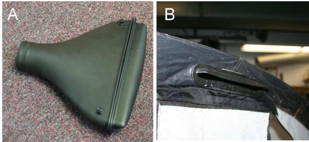
**Figure 2.2:** Overview of tent suction port showing: top-down view (A), installed port showing opening design (B).
