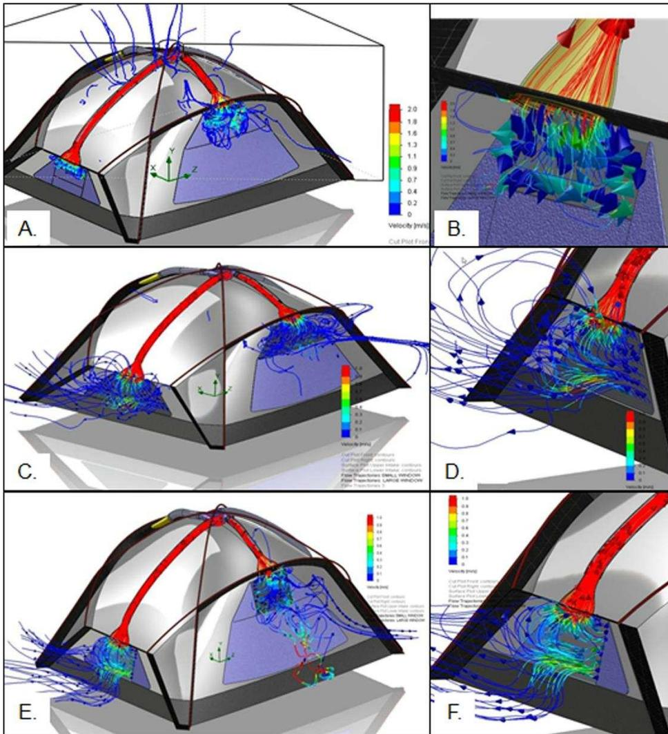
**Figure 2.3:** Computational fluid dynamics visualization demonstrating volatile distribution and recirculation in all possible patch configurations.
