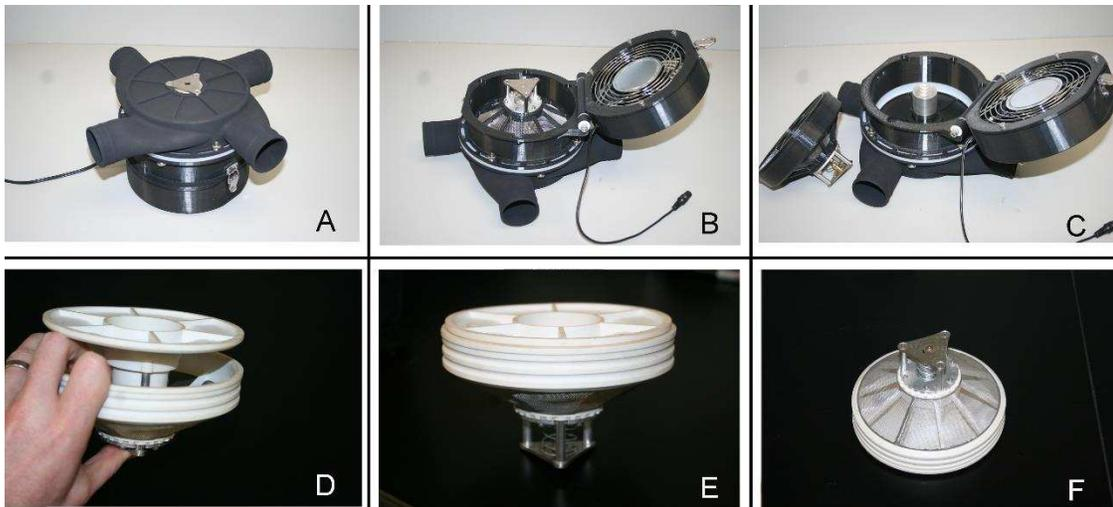
**Figure 2.4A-F.** Pictures of whole manifold (A), vector trap screwed in manifold with fan attachment open (flipped upside-down) (B), manifold with vector trap removed (flipped upside-down) (C), vector trap open from side (D), closed collection chamber from above (E), and below (F). Note: D-F are the newer version of the collection chamber. This design added the spokes to limit vector movement, and utilized white plastic for easier vector viewing/removal.
