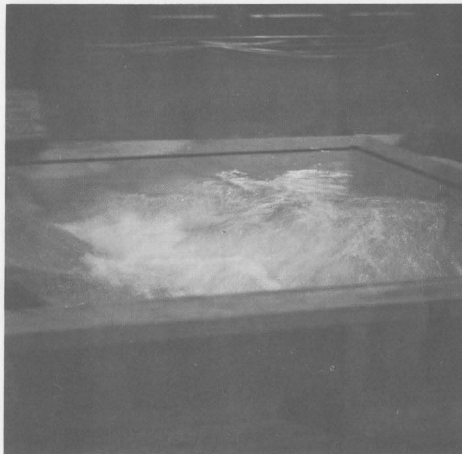
Fig. 23. Operation of energy dissipator at 24,000 cfs
