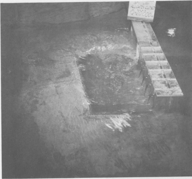
Fig. 16. Flow at 20,000 cfs with gates closed
