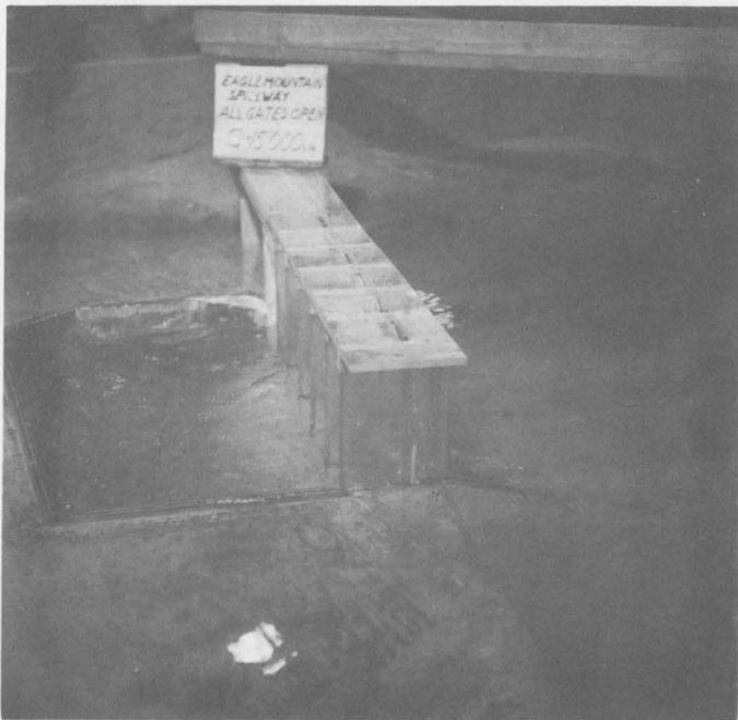
Fig. 11. Flow at 15,000 cfs with gates open
